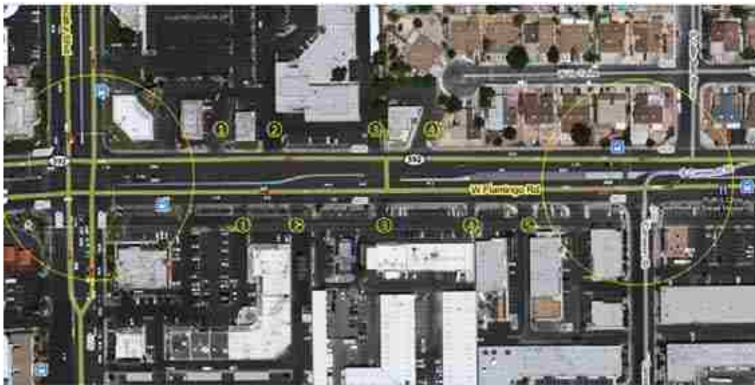
Figure 4-5 Illustration of Driveways and Median Opening
