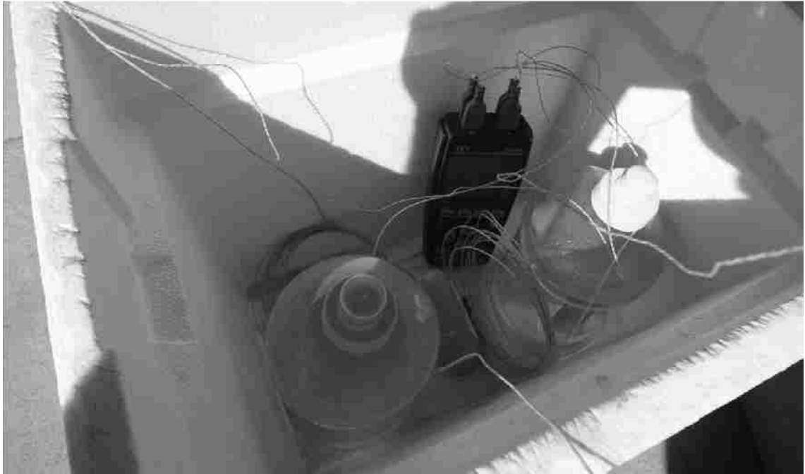
Figure 2.5 YCT brand temperature data logger with ice water containers
