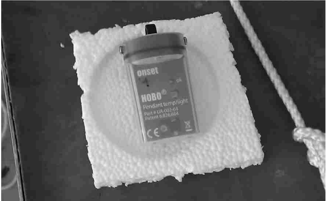
Figure 2.7 Onset HOBO® pendant temperature/light data logger
