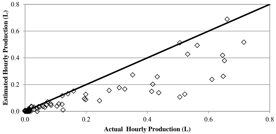
Figure 3.48 Estimated vs. actual hourly production for SS1-B (13 L)
