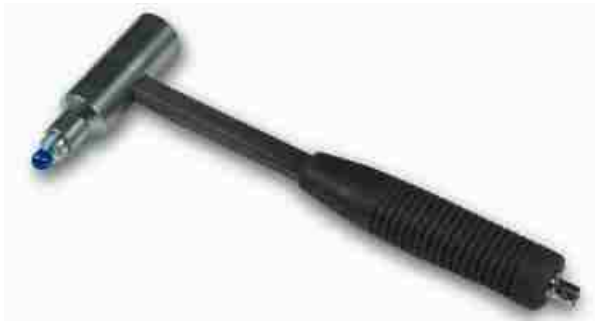
(a) Impact hammer, PCB 086D05
