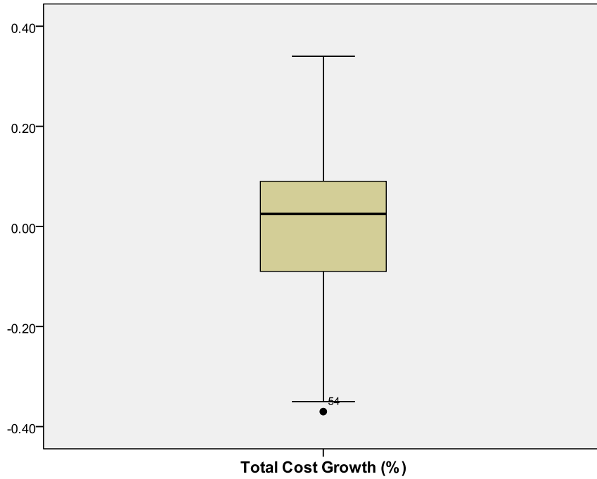
Figure C- 29. Box plot for total cost growth (%) of TXDOT and CCDPW road projects
