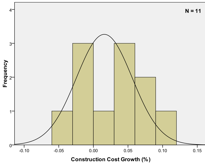
Figure B- 18. Histogram for construction cost growth (%) of CCDPW flood control projects
