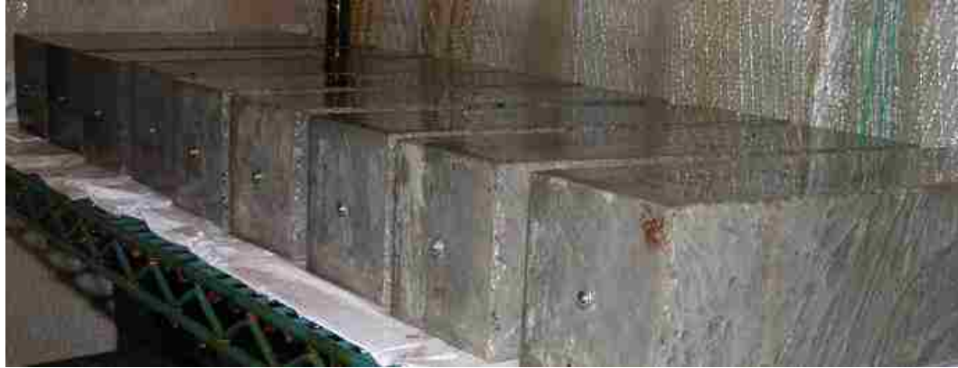
Figure 2.10: Prisms stored in a moisture room for ASTM C 1105 test
