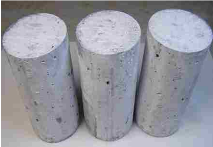
(a) Cylinders made with the innocuous aggregate (SN-E)
