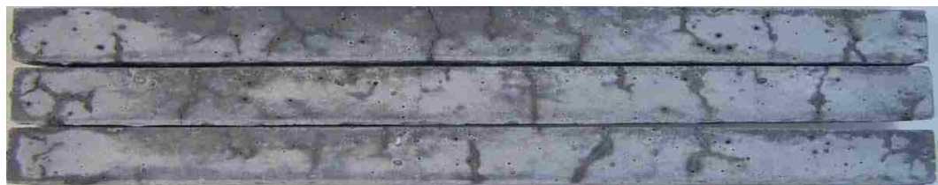
(e) Treated mortar bars with the lithium-to-alkali molar ratio of 1.04
