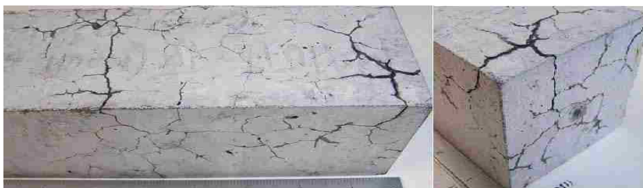
Figure 3.28: Prism containing highly reactive aggregate (NN-B)
