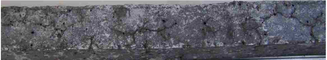
(b) Mortar bar submerged in the 0.5N NaOH
