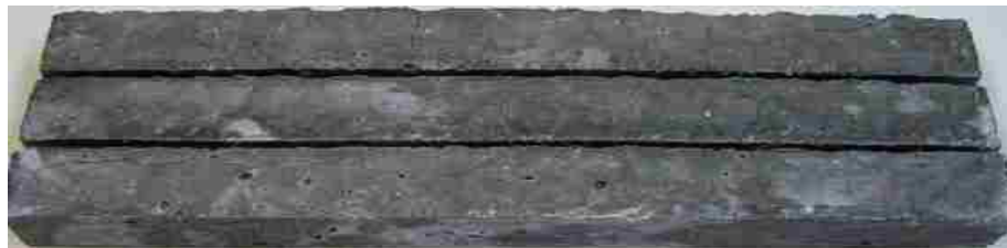
(e) Treated bars with the 15%FA+100%Li ( E_{14\text{-day}} = 0.052\% ; E_{98\text{-day}} = 0.82\% )
