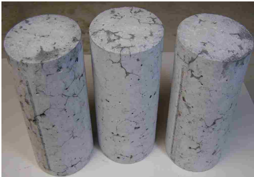
(b) Cylinders made with the reactive aggregate (NN-C)
