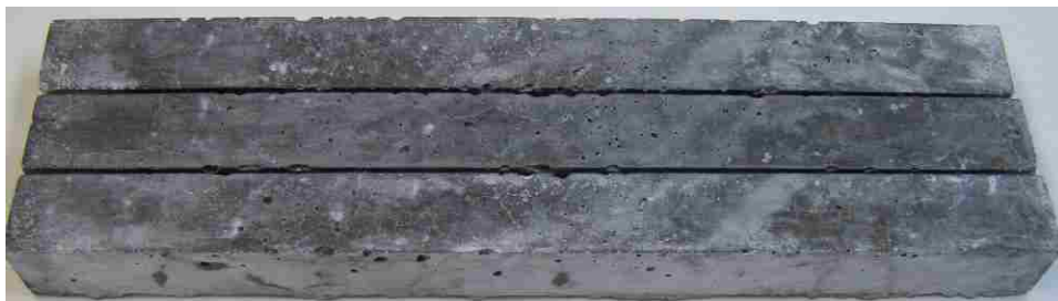
(e) Treated mortar bars with the 30% Class F fly ash
