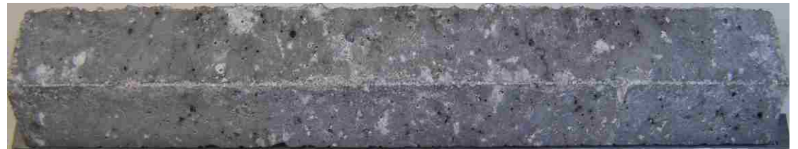
(c) Mortar bar submerged in the 0.25N NaOH
