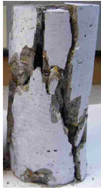
(b) Cylinder made with reactive agg.
