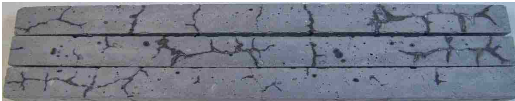
(c) Treated mortar bars with the lithium-to-alkali molar ratio of 0.74
