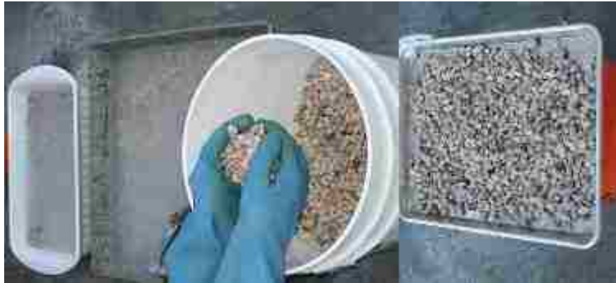
Figure 2.2: Washing coarse aggregates
