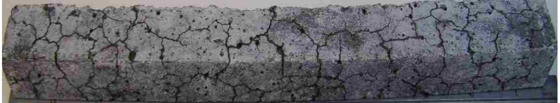
(a) Mortar bar submerged in the 1N NaOH
