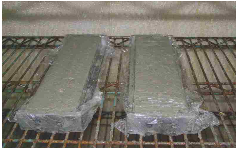
Figure 2.8: Mortar bars cured for 24 hours in a moisture room after casting
