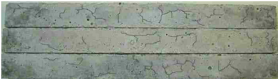
(c) Treated mortar bars with the 20% Class F fly ash
