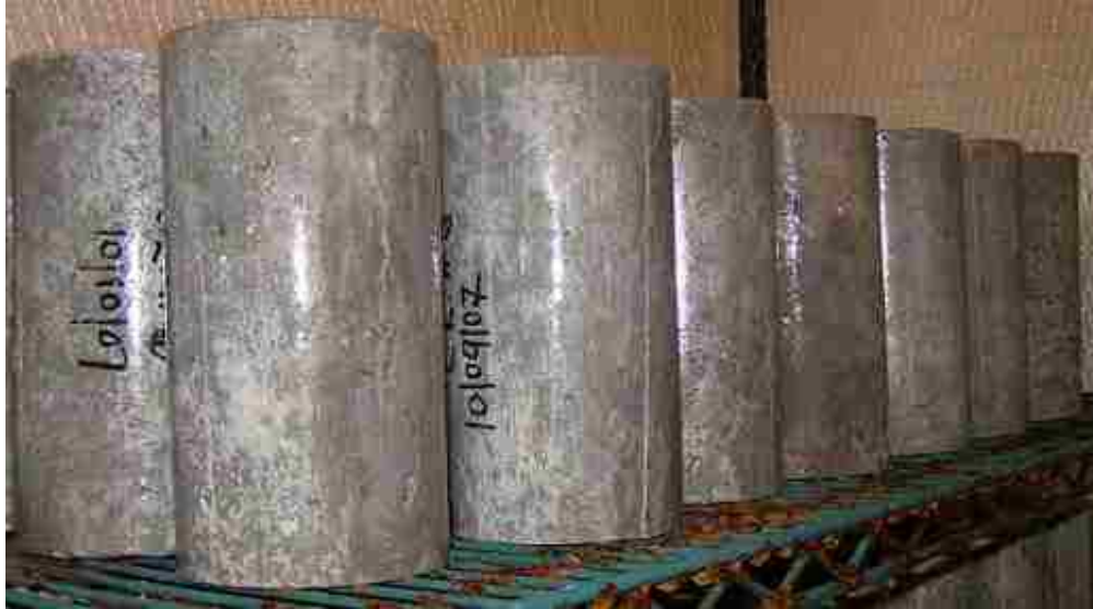
Figure 2.11: Cylinders stored in a moisture room at a temperature of 20°C
