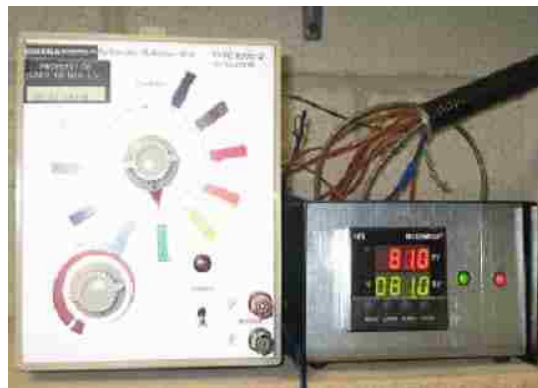
(c) Temperature controller
