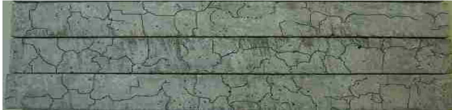
(b) Treated mortar bars with the 15%FA ( E_{14\text{-day}} = 0.25\% ; E_{98\text{-day}} = 1.62\% )
