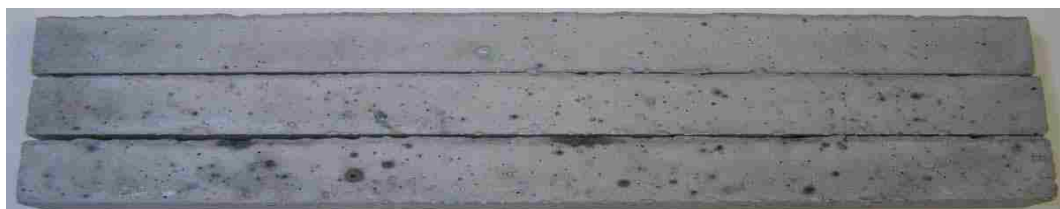
(f) Treated mortar bars with lithium-to-alkali molar ratio of 1.19
