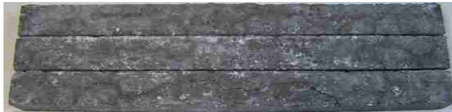
(d) Treated bars with the 100%Li ( E_{14\text{-day}} = 0.18\% ; E_{98\text{-day}} = 1.04\% )
