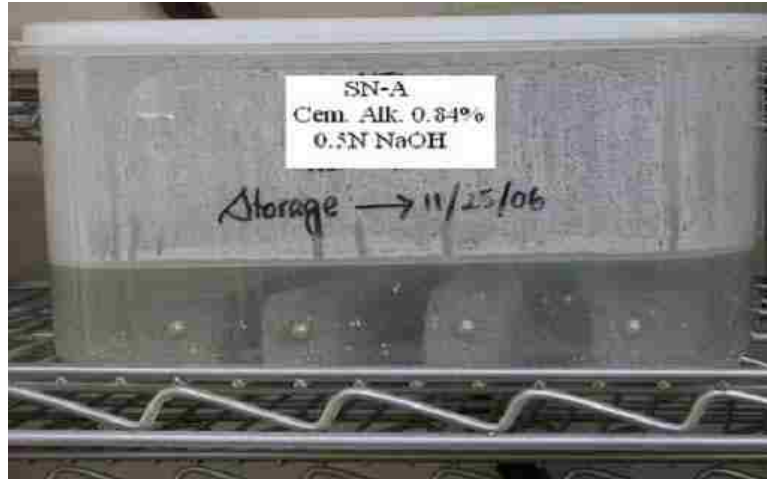
Figure 2.9: Mortar bars stored in NaOH solution at 80°C
