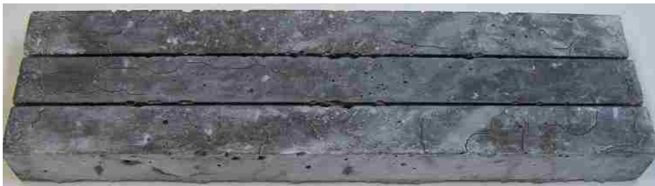
(d) Treated mortar bars with the 25% Class F fly ash
