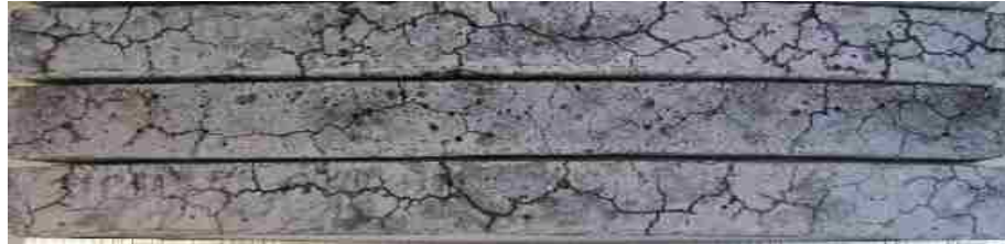
(a) Untreated mortar bars ( E_{14\text{-day}} = 1.10\% ; E_{98\text{-day}} = 2.34\% )
