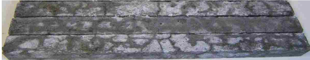
(b) Treated mortar bars with the lithium-to-alkali molar ratio of 0.59
