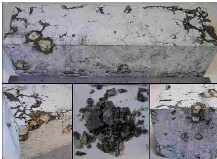
Figure 3.29: Aggregates popped-out from the prism of highly reactive aggregate (SN-G)
