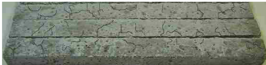
(c) Treated mortar bars with the 20%FA ( E_{14\text{-day}} = 0.152\% ; E_{98\text{-day}} = 1.17\% )
