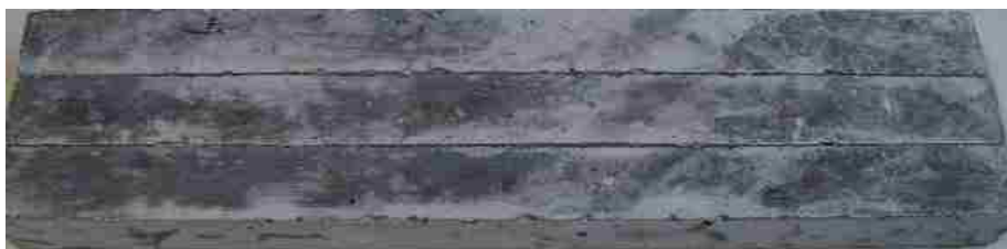
(f) Treated bars with the 20%FA+100%Li ( E_{14\text{-day}} = 0.042\% ; E_{98\text{-day}} = 0.59\% )
