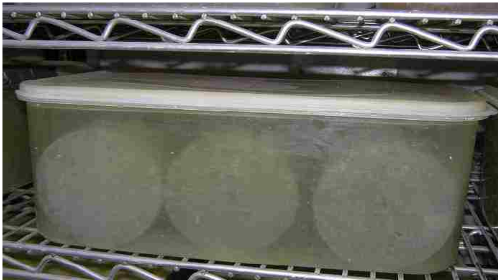
Figure 2.12: Cylinders stored in 1N NaOH solution at a temperature of 80°C
