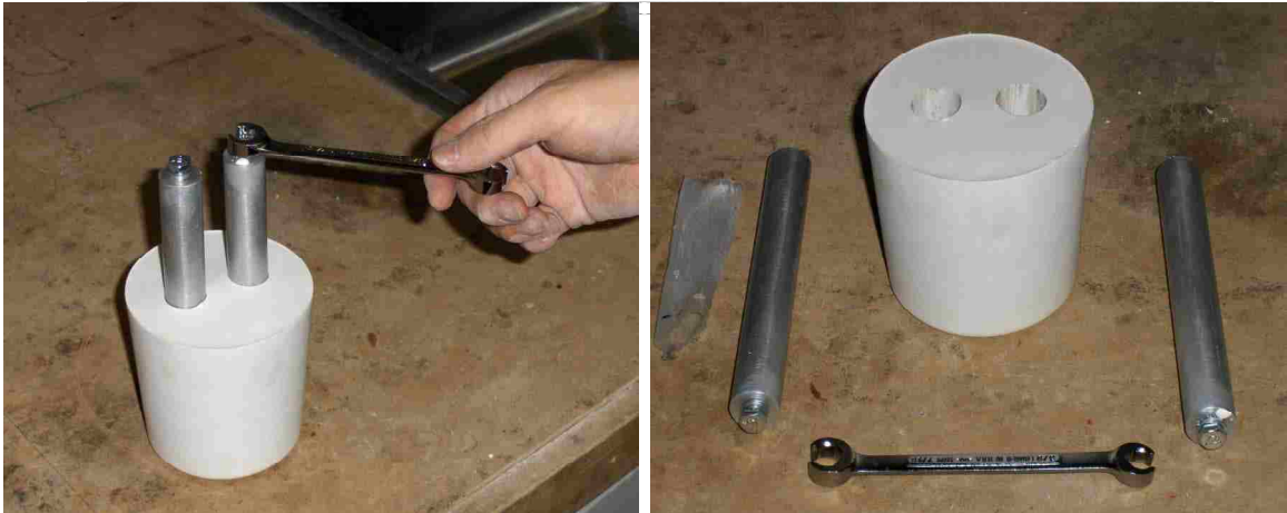
Figure 16 Aluminum Rod Removal Test
