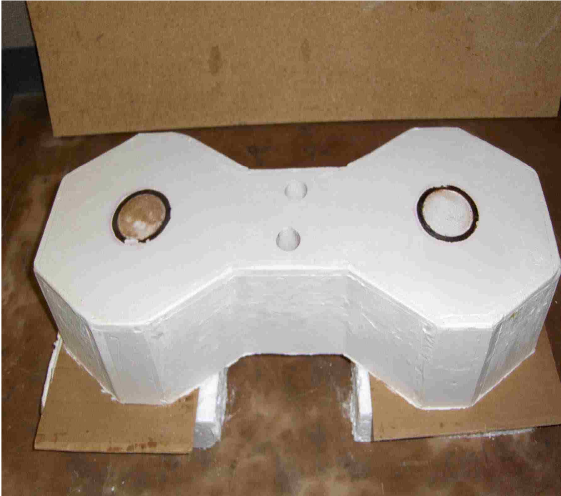
Figure 17 Dog Bone 5 after Aluminum Rods and Mold Removals
