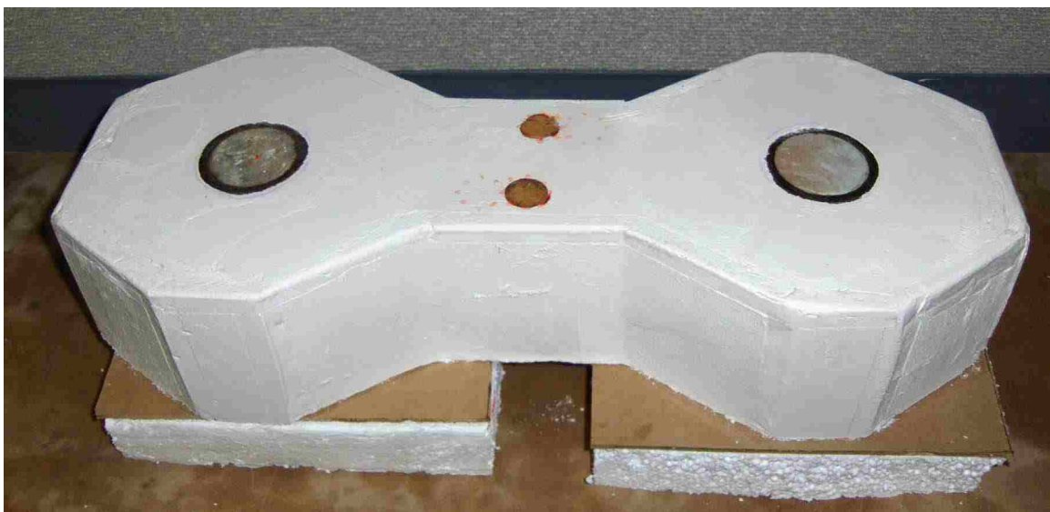
Figure 14 Dog Bone 4 after Mold Removal
