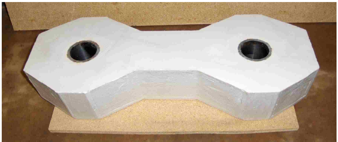
Figure 2 Hydro-Stone TB Specimen Dog Bone 1
