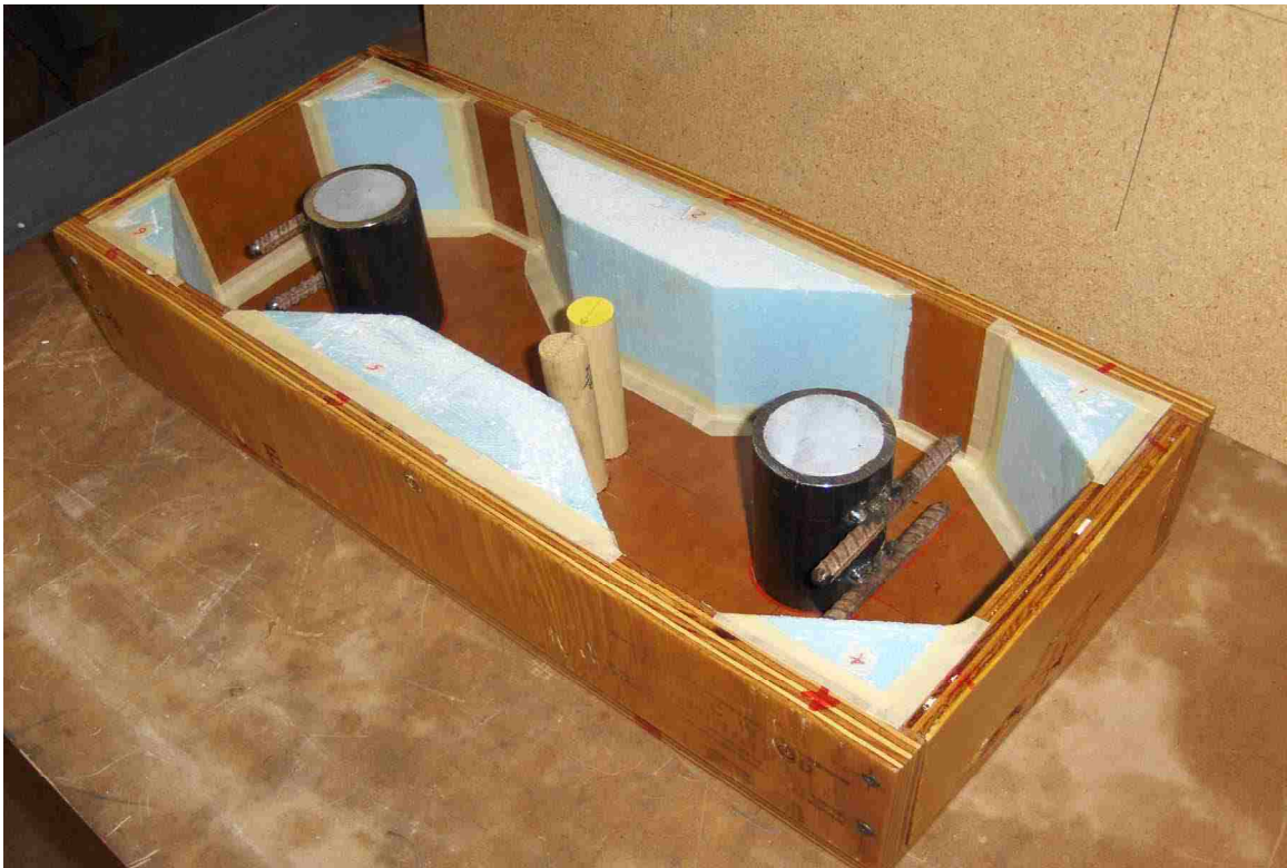
Figure 10 Mold for Dog Bone 3 with Pipes, Bars and Porosity Dowels
