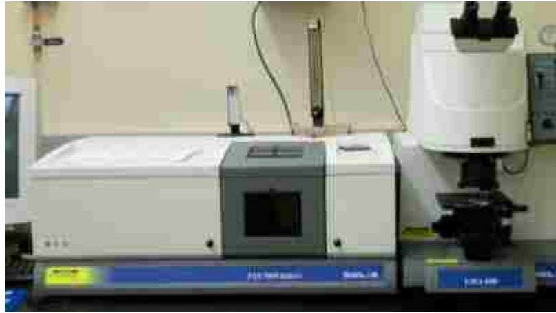
(a) Phase 2 – FTIR spectrometer and microscope
