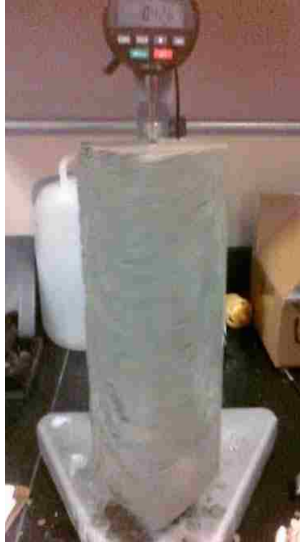
Figure 18 – Comparator used to measure change of length in freezing and thawing sample
