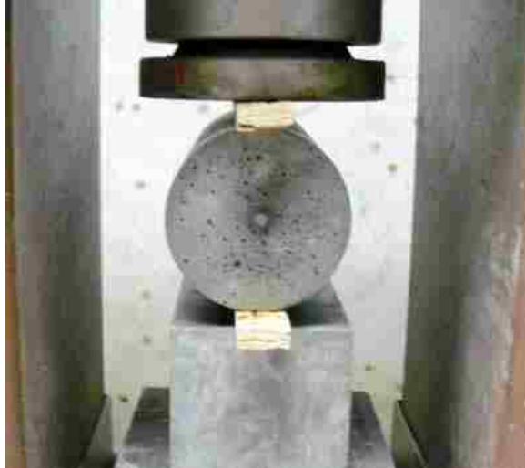
Figure 12 – Splitting tensile strength
