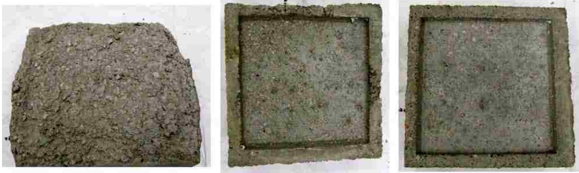
Figure 42 – Images of surface scaling samples (from left to right: NC, SBR, WLP)
