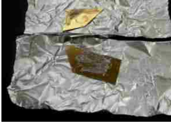
(c) Phase 2 – Dried paint on gold substrate
