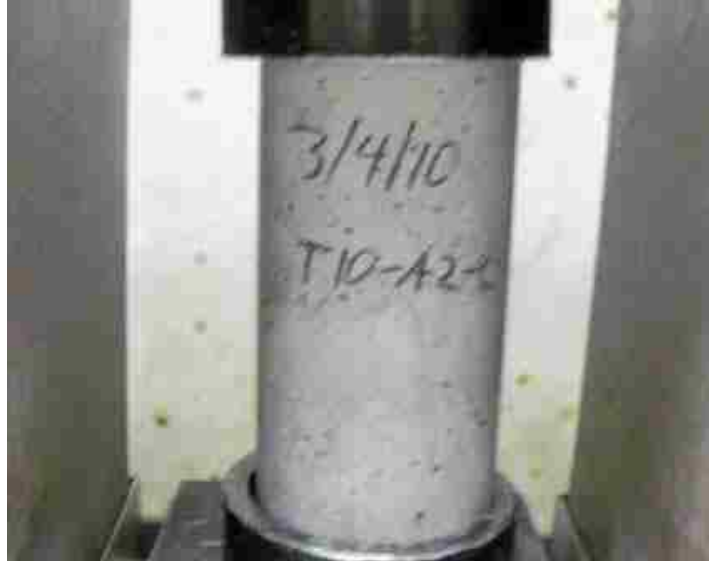
Figure 11 – Compressive strength setup
