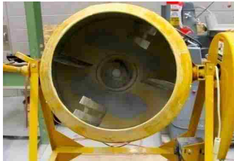
Figure 4 – Steel drum mixer
