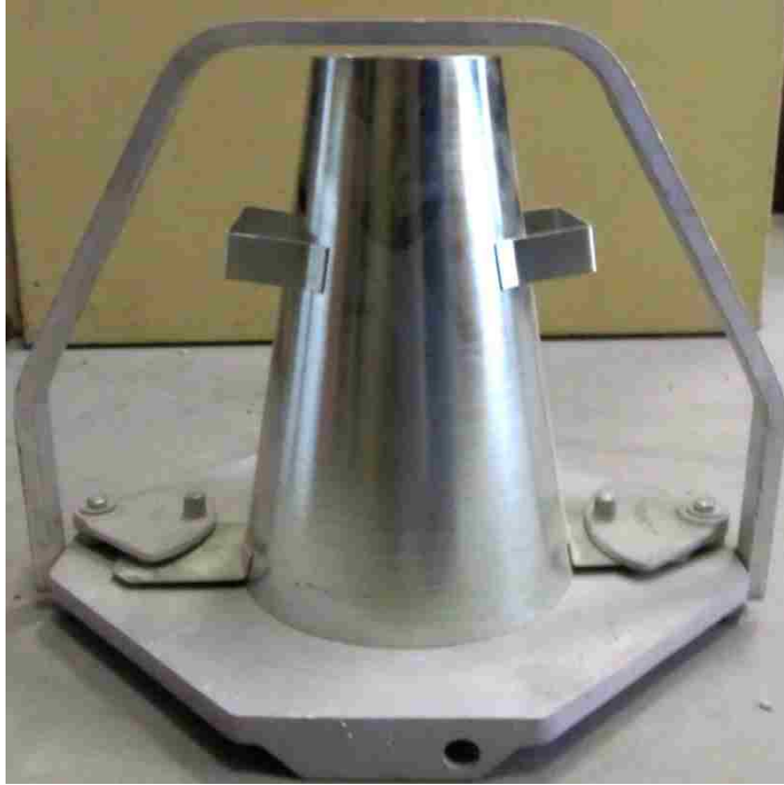
Figure 8 – Slump cone used for testing
