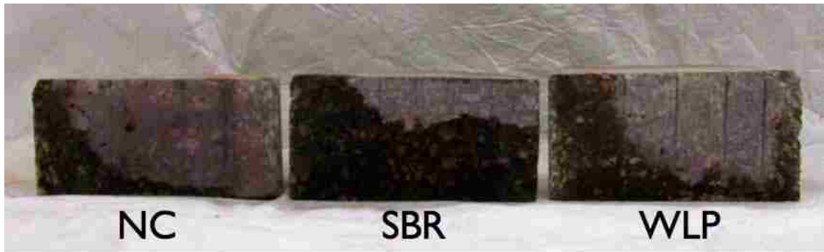
Figure 35 – Images of chloride penetration depth on RCPT samples
