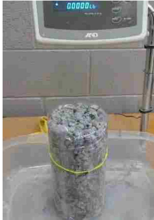
Figure 20 – Porosity of pervious concrete setup
