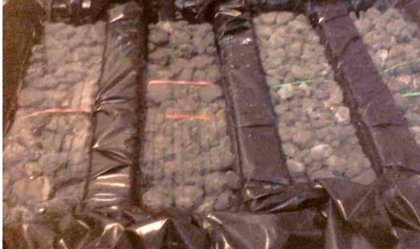
Figure 19 – Pervious concrete in freeze-thaw test
