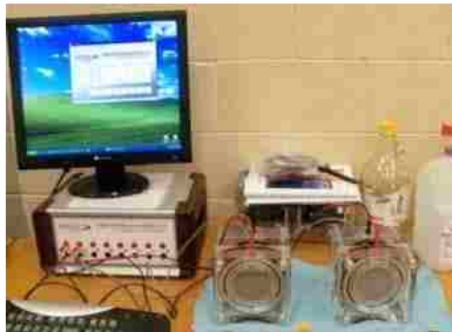
Figure 16 – Rapid chloride penetrability test setup
