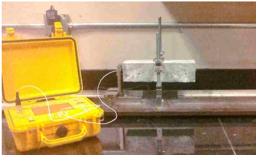
Figure 17 – Transverse elasticity test setup of freezing and thawing sample
