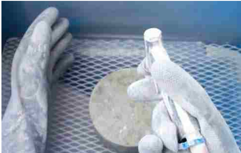
Figure 15 – Abrasion by sandblasting
