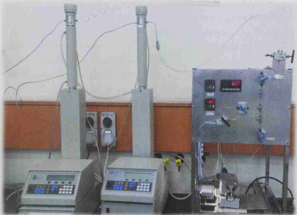
Figure 4.4: The PVT cell experimental setup used in this work
