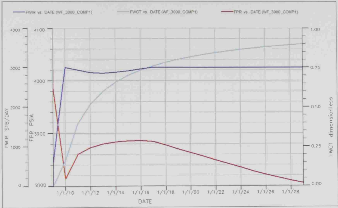
Figure 5.7: Waterflooding injection at 3000 STB/D (COMP1) reservoir performance
