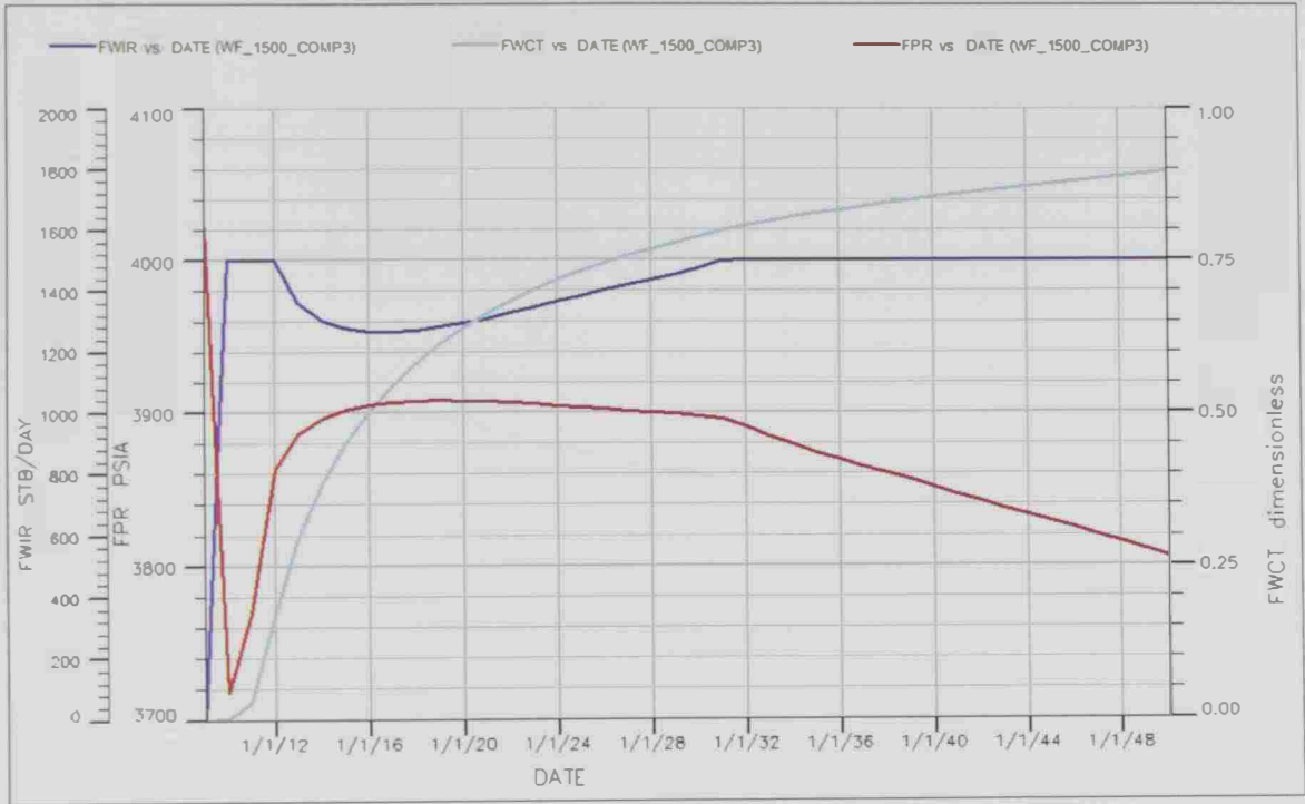
Figure 5.12: Waterflooding injection at 1500 STB/D (COMP3) reservoir performance
