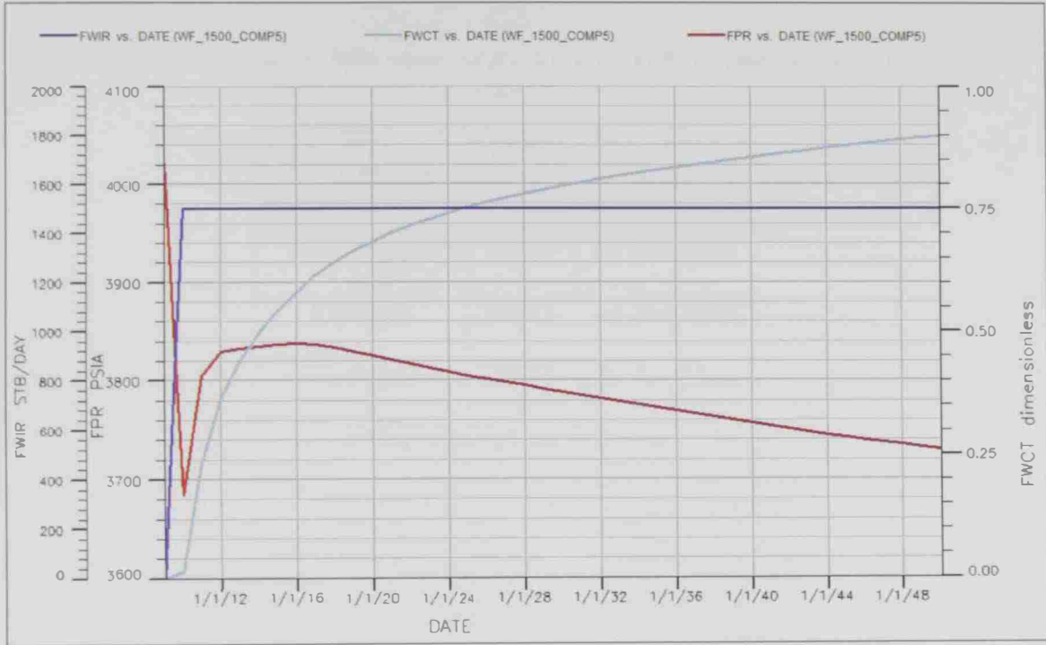
Figure 5.14: Waterflooding injection at 1500 STB/D (COMP5) reservoir performance
