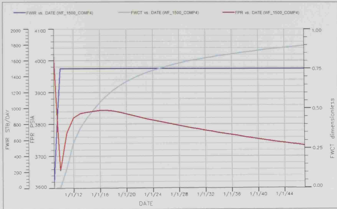
Figure 5.13: Waterflooding injection at 1500 STB/D (COMP4) reservoir performance
