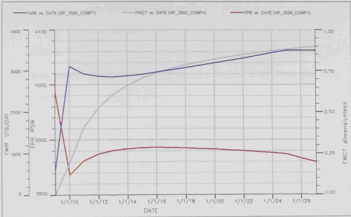
Figure 5.8: Waterflooding injection at 3500 STB/D (COMP1) reservoir performance
