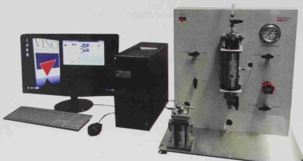
Figure E.1: PoroPerm instrument used for porosity and permeability measurement
