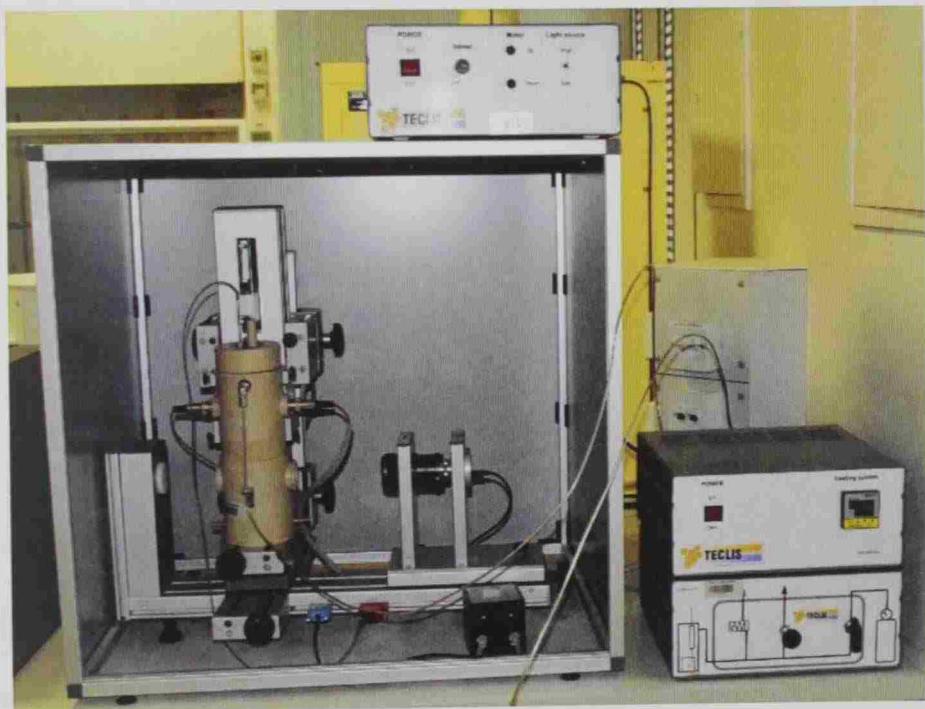
Figure 2.6: Teclic-Tracker used for IFT and contact angle measurements
