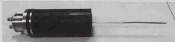
Figure E.3: A complete set-up of flood head, end-stem, core plug and sleeve
