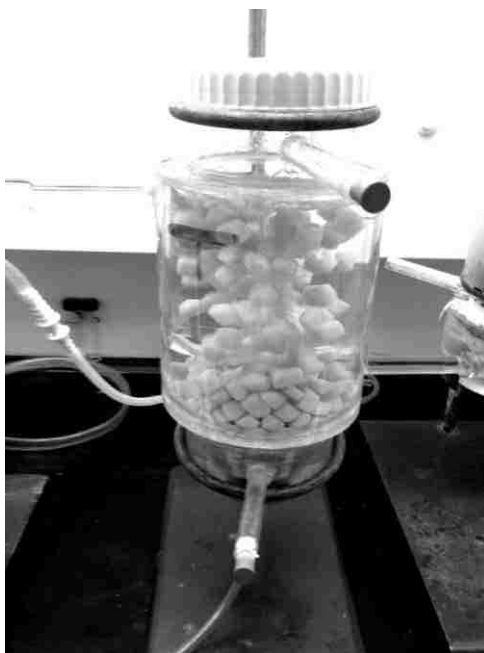
Fig. 4.3.17 Mixing regime in the short reactor at AFR of 1 l/min: pH 7.0; T = 30 °C; C_o = 75 mg/l
