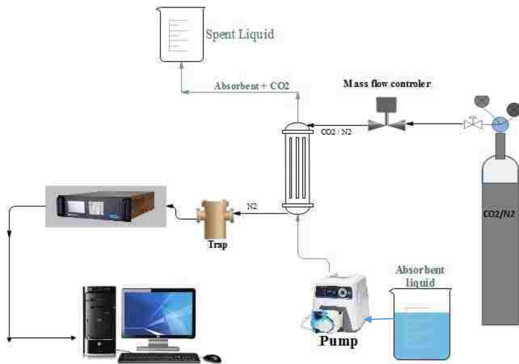
Figure 21: Schematic set-up of absorption process
