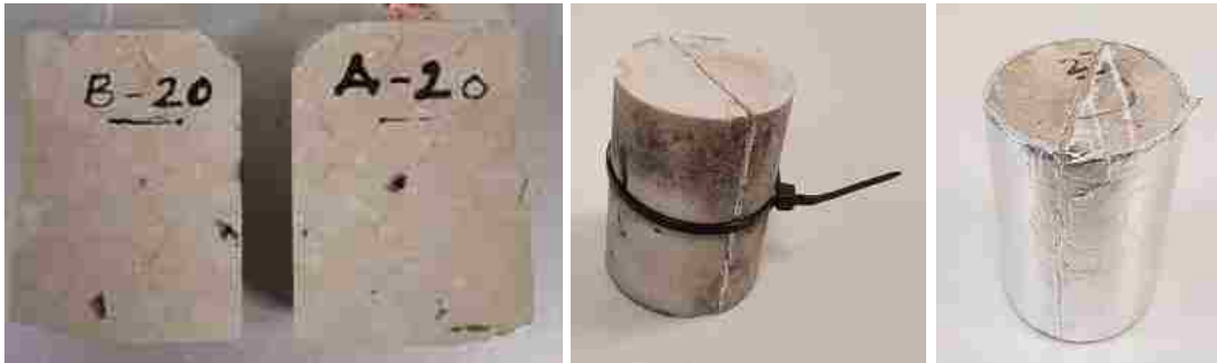
Figure 10: Simulating a single induced fracture
