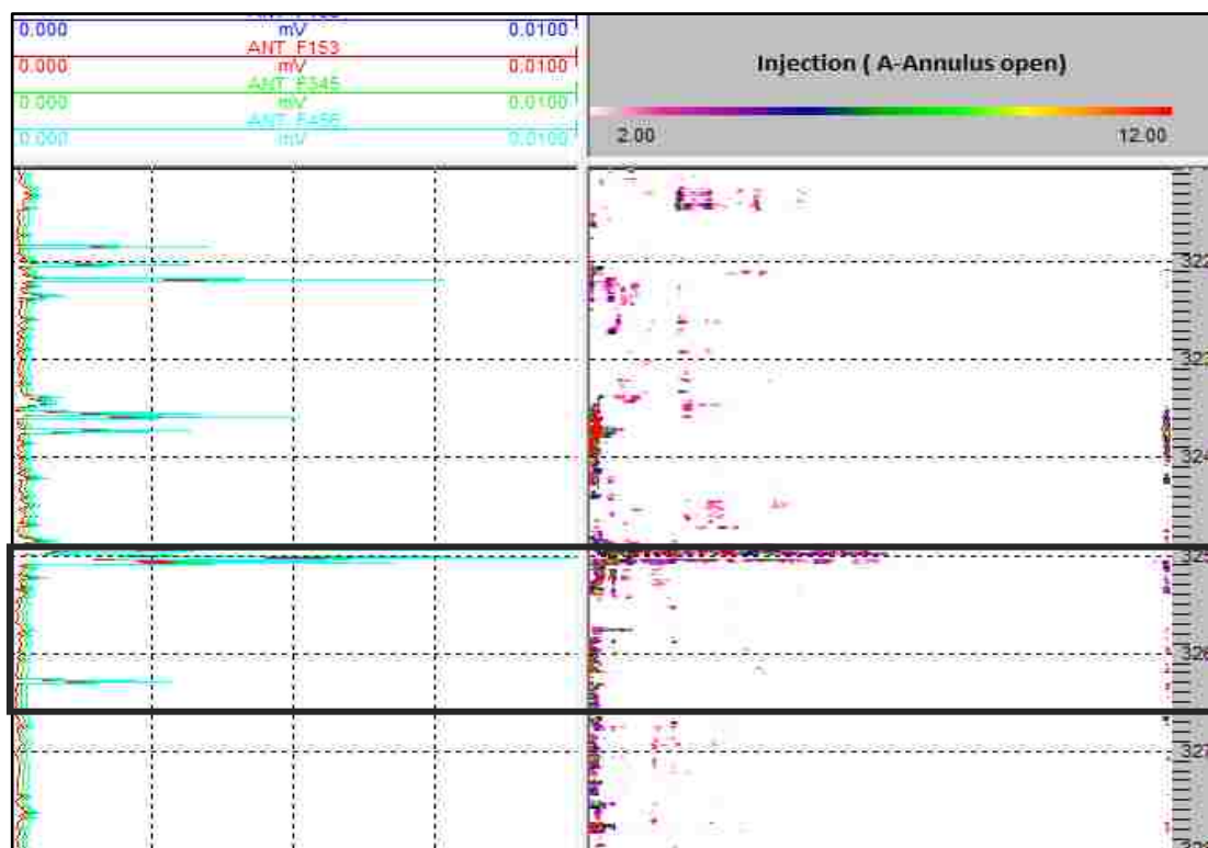
Figure 34: Array noise log under injection with open A-Annulus condition at the packer interval
