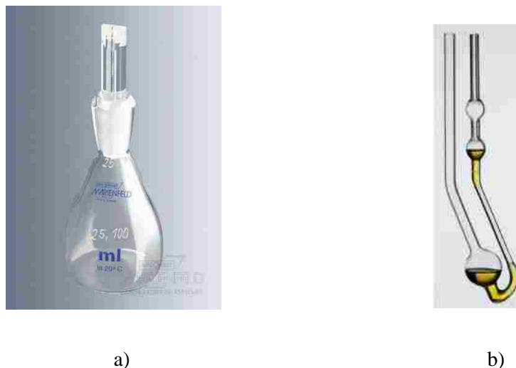
Figure 3.3: a) Pycnometer b) Canon-Fenske
