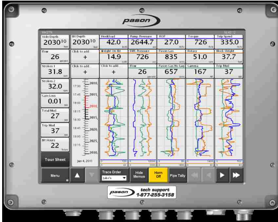
Figure 1.9. Example of an EDR Screen, From Pason Systems
