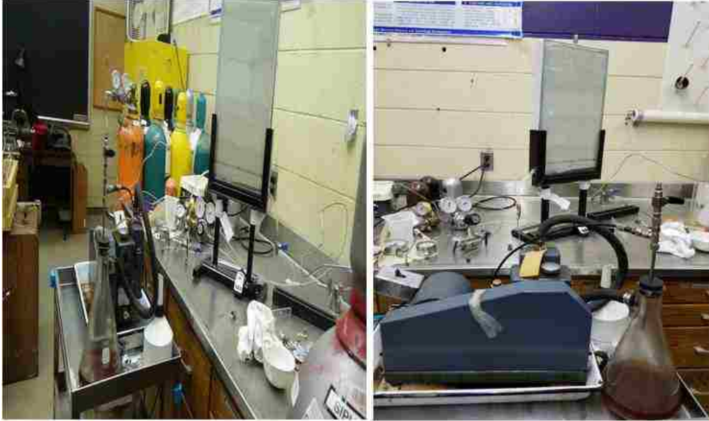
Figure 0.10. Vacuum Pump applied to the model prior to GAGD runs
