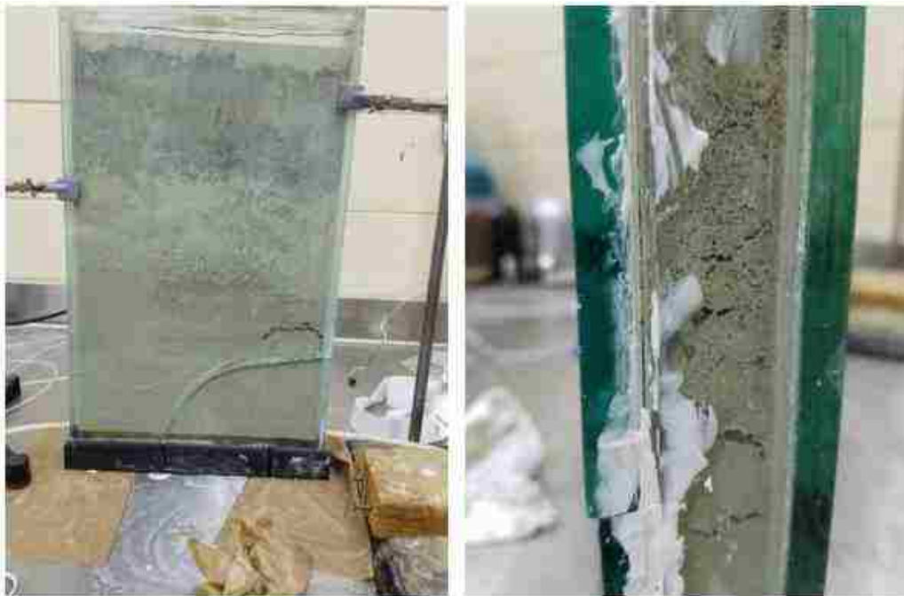
Figure 3.4. Cracked model due to the increased pressure
