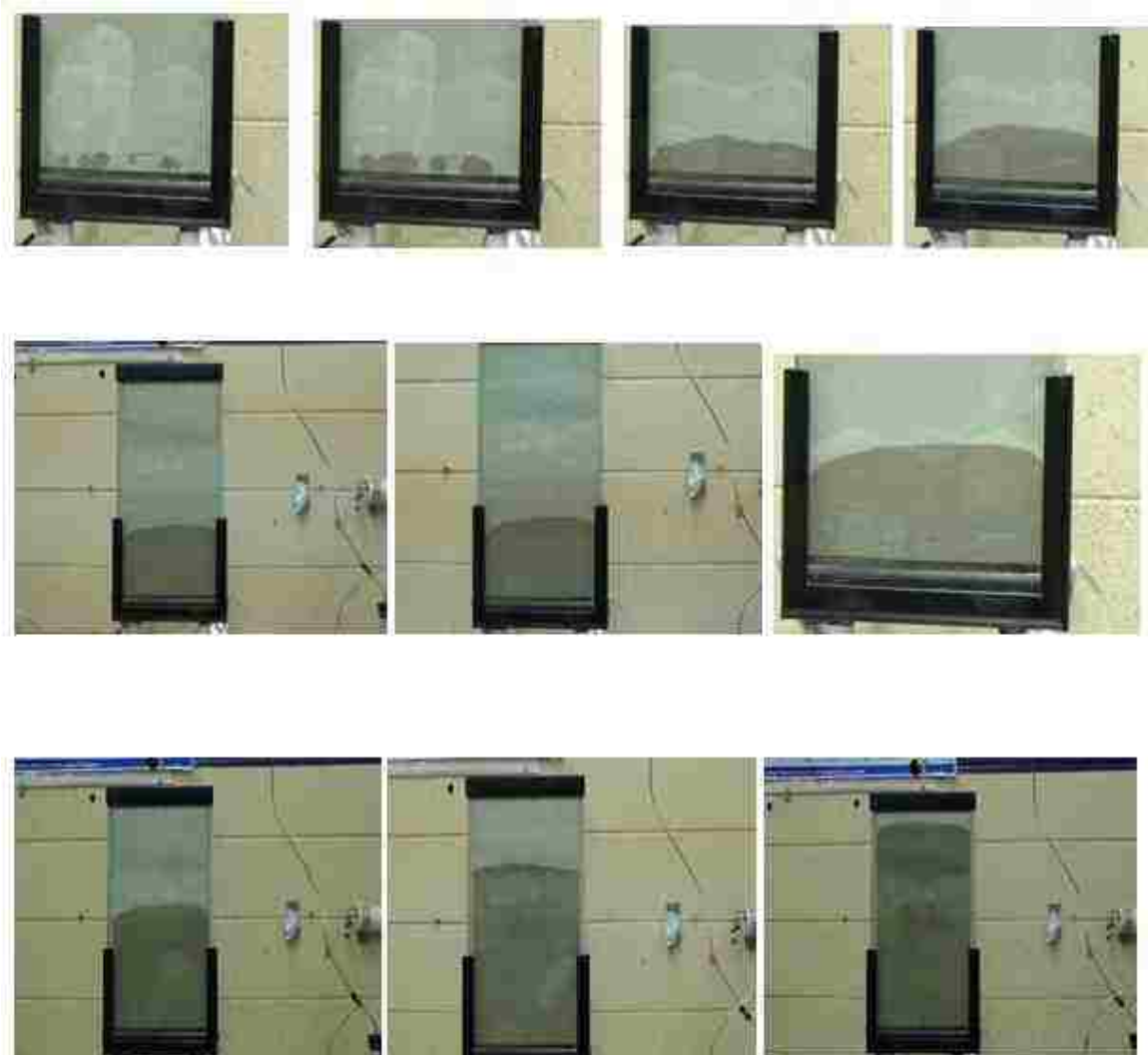
Figure 3.3. Water front propagation moving through the model upon initial water saturation run
