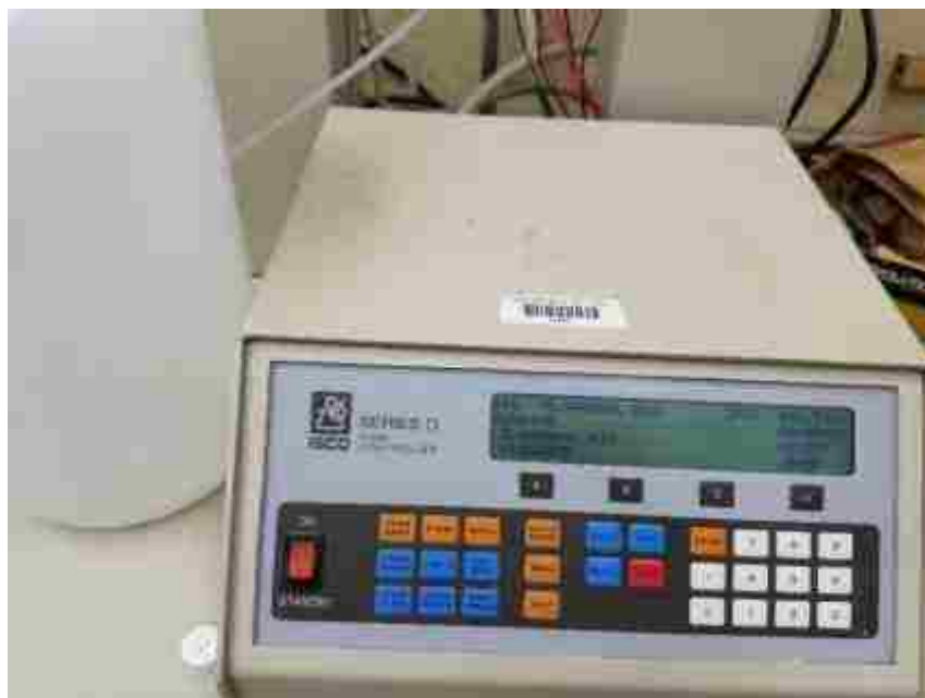
Figure 3.2. Pump Controls for the Series D Pump
