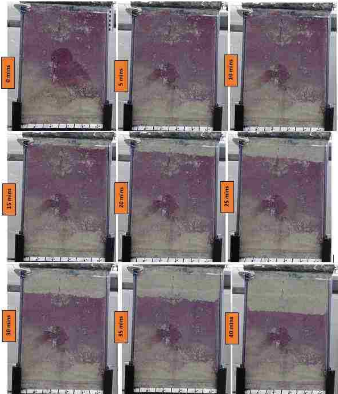
Figure 0.9. Front propagation for N 2 flooding at 5 cc/min for Model # 1 (1 of 2)
