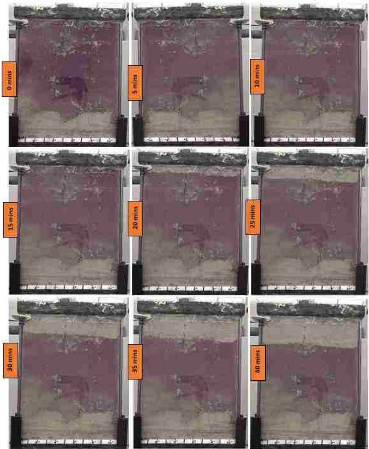
Figure 0.11. Front propagation for CO 2 flooding at 5 cc/min for Model # 1 (1 of 2)
