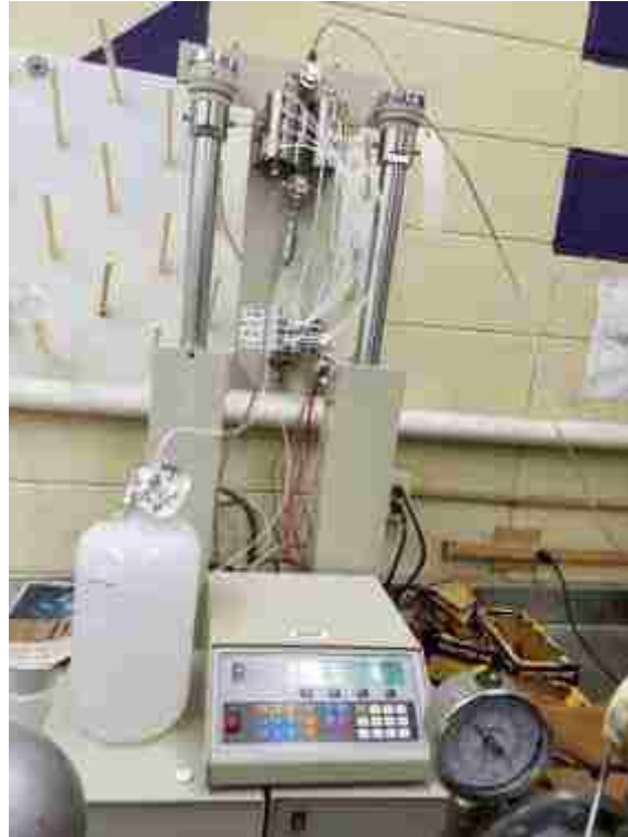
Figure 3.1. Teledyne ISCO Series D Pump used initially for fluid injection
