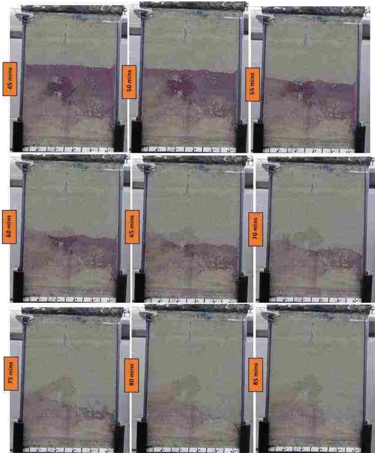
Figure 0.10. Front propagation for N 2 flooding at 5 cc/min for Model # 1 (2 of 2)
