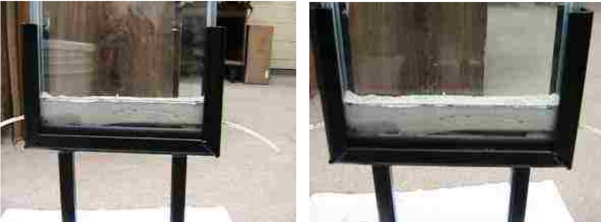
Figure 0.9. Placement of a 2” layer of higher sized carbonate grains (600 \mu\text{m} ) in the model
