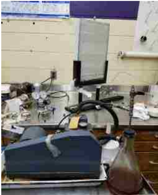
Figure 0.7. Vacuum pump used to remove trapped air from the model
