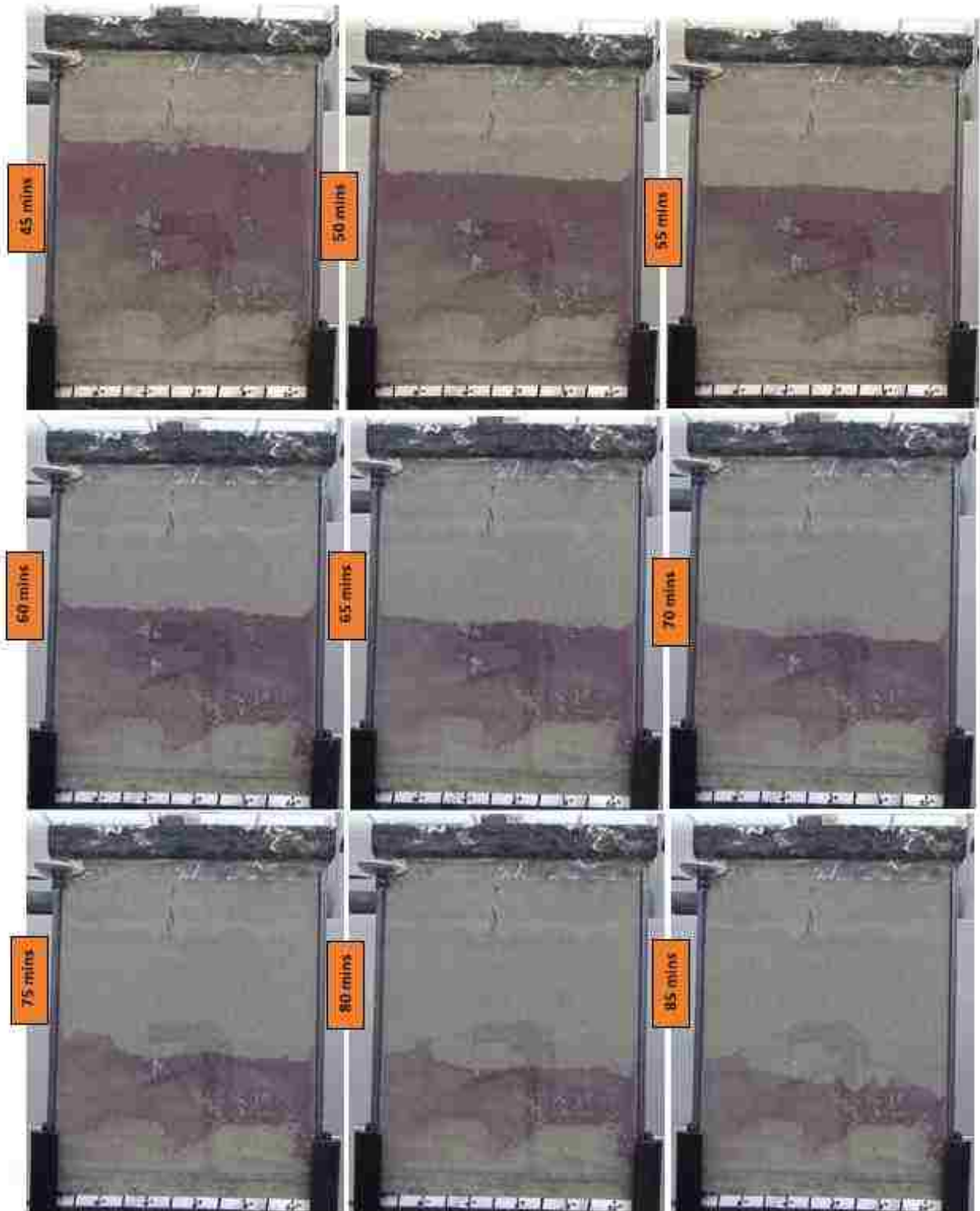
Figure 0.12. Front propagation for CO 2 flooding at 5 cc/min for Model # 1 (2 of 2)
