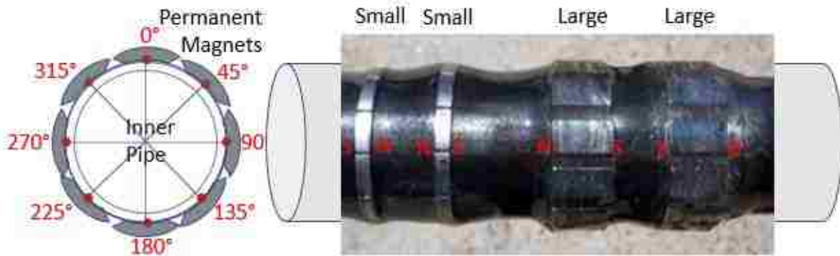
Fig. C1. Magnetic Field Measurement at permanent magnets
