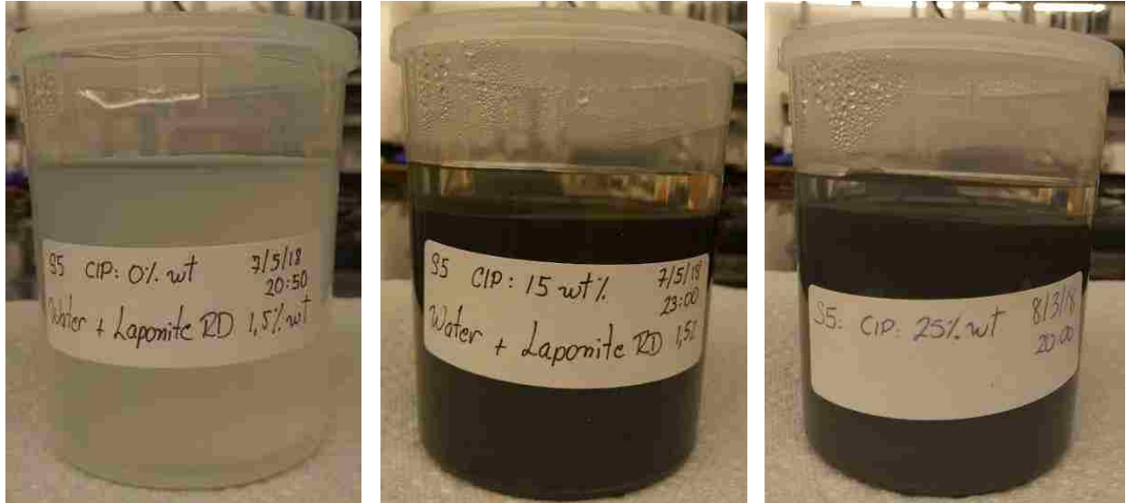
Fig. 22. Settling Ratio of Sample S5 after 77 days of mixed
