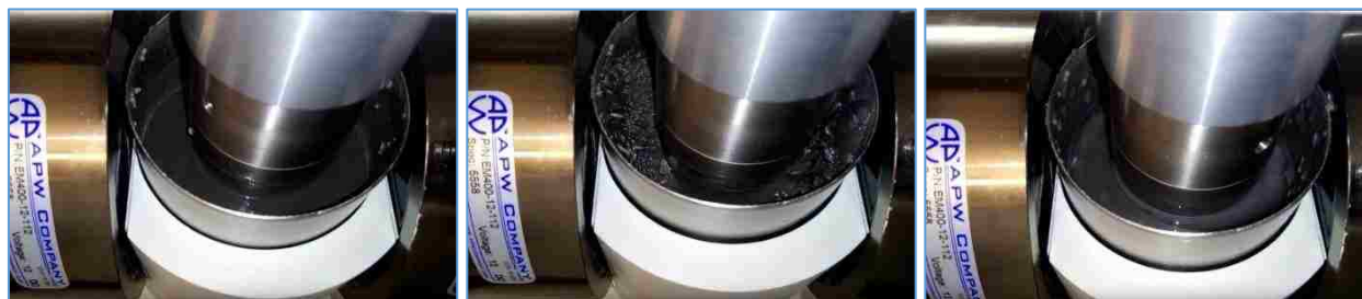
Fig. F1. Sample S1 CIP 15wt% reaction to 48V ON/OFF
