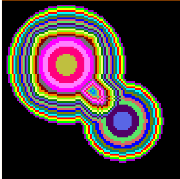
Figure 4.1. Burn map for two overlapping spheres, 100 voxels per side with a nominal voxel width of 0.01 cm
