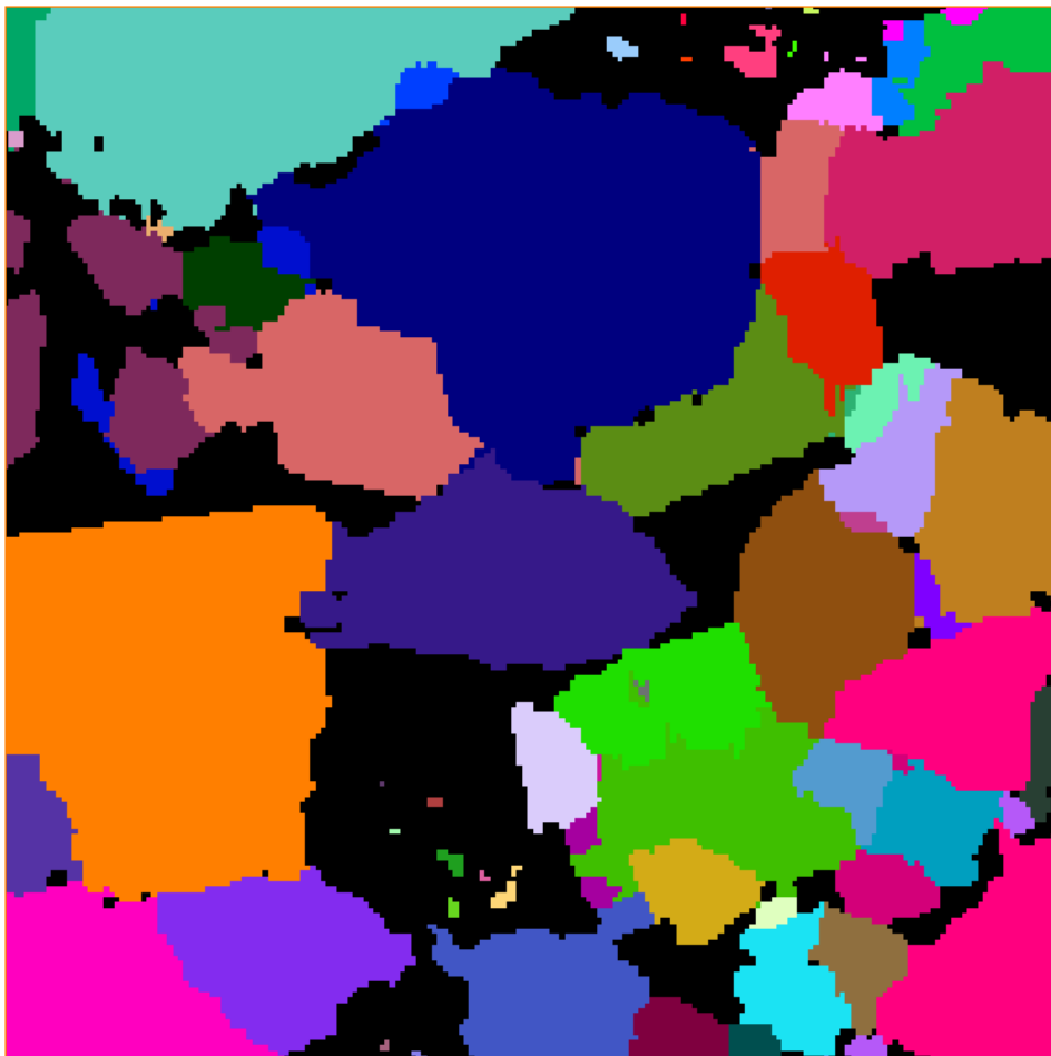
Figure 4.14. Partitioned quartz-feldspar image with 0 voxel overwrites and 1 grain assembly iteration, 820 \mu m per side, 200 3 voxels
