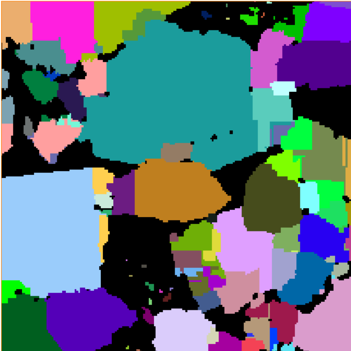
Figure 4.23. Partitioned quartz-feldspar using original program, 820 \mu m per side, 200 3 voxels
