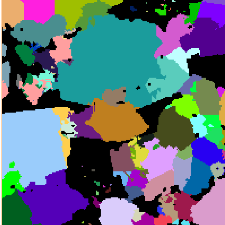
Figure 3.9. Partitioned image of quartz-feldspar rock using burn connectivity value of six and a connectivity for contacts of twenty-six, 820 \mu m per side, 200 3 voxels
