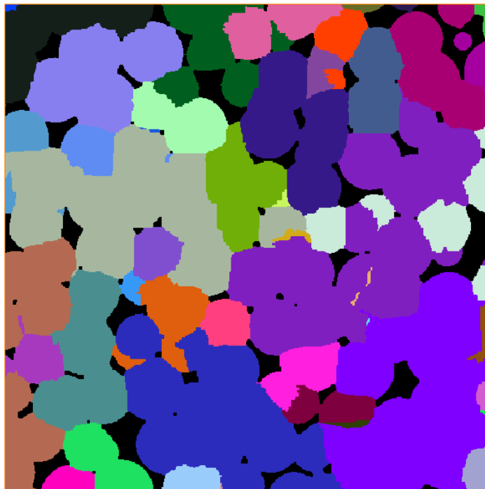
Figure 3.16. Refined output using the initial automerge logic with a contact area to surface area ratio of 0.15, 500 voxels per side with a nominal voxel width of 0.01 cm/voxel
