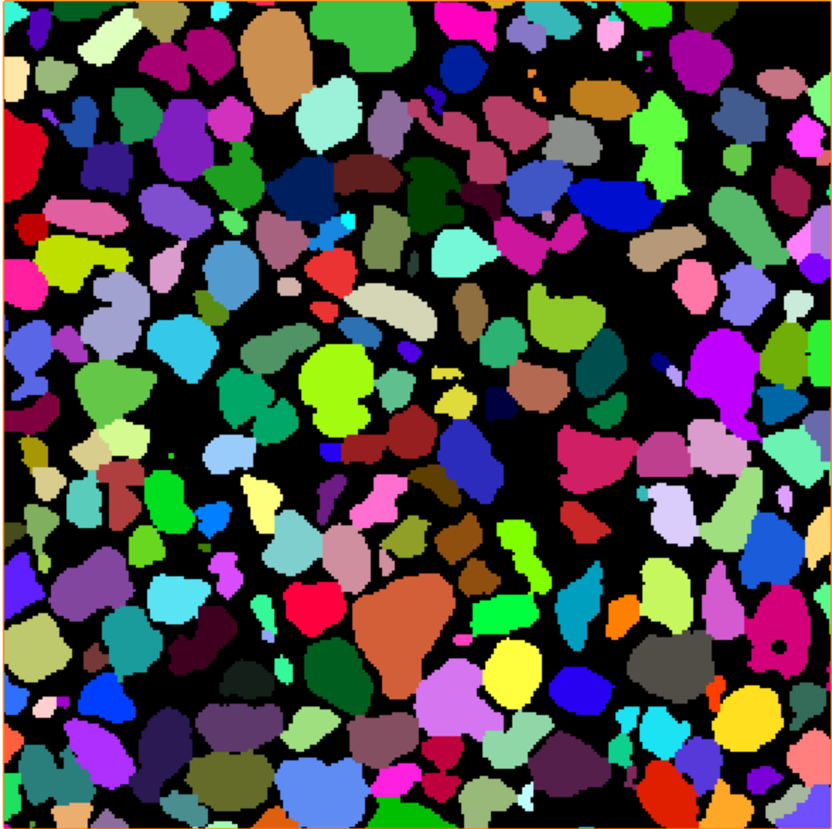
Figure A.11. Ottawa sand 10 after trial 2 logistic regression equation, 3045 grains, 3.025 mm per side, 275^3 voxels
