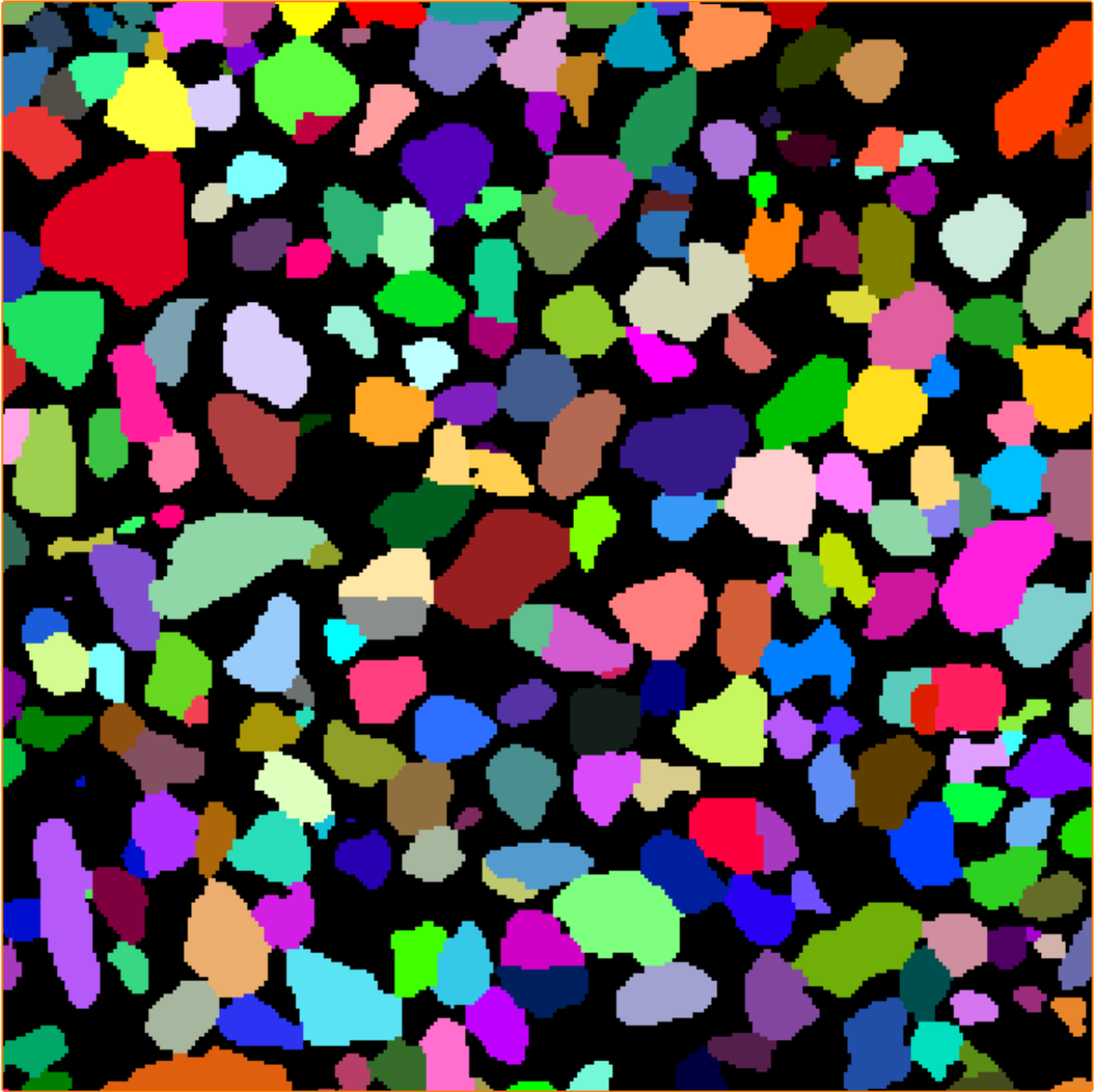
Figure A.4. Ottawa sand 5 VOX2GRAINS updated output, 3775 grains, 3.025 mm per side, 275^3 voxels
