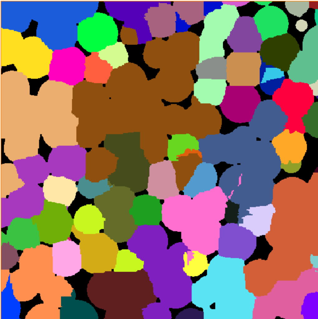
Figure 4.25. Partitioned overlapping sphere pack with updated automerge logic and a contact area to surface area ratio of 0.95, 500 voxels per side with a nominal voxel width of 0.01 cm
