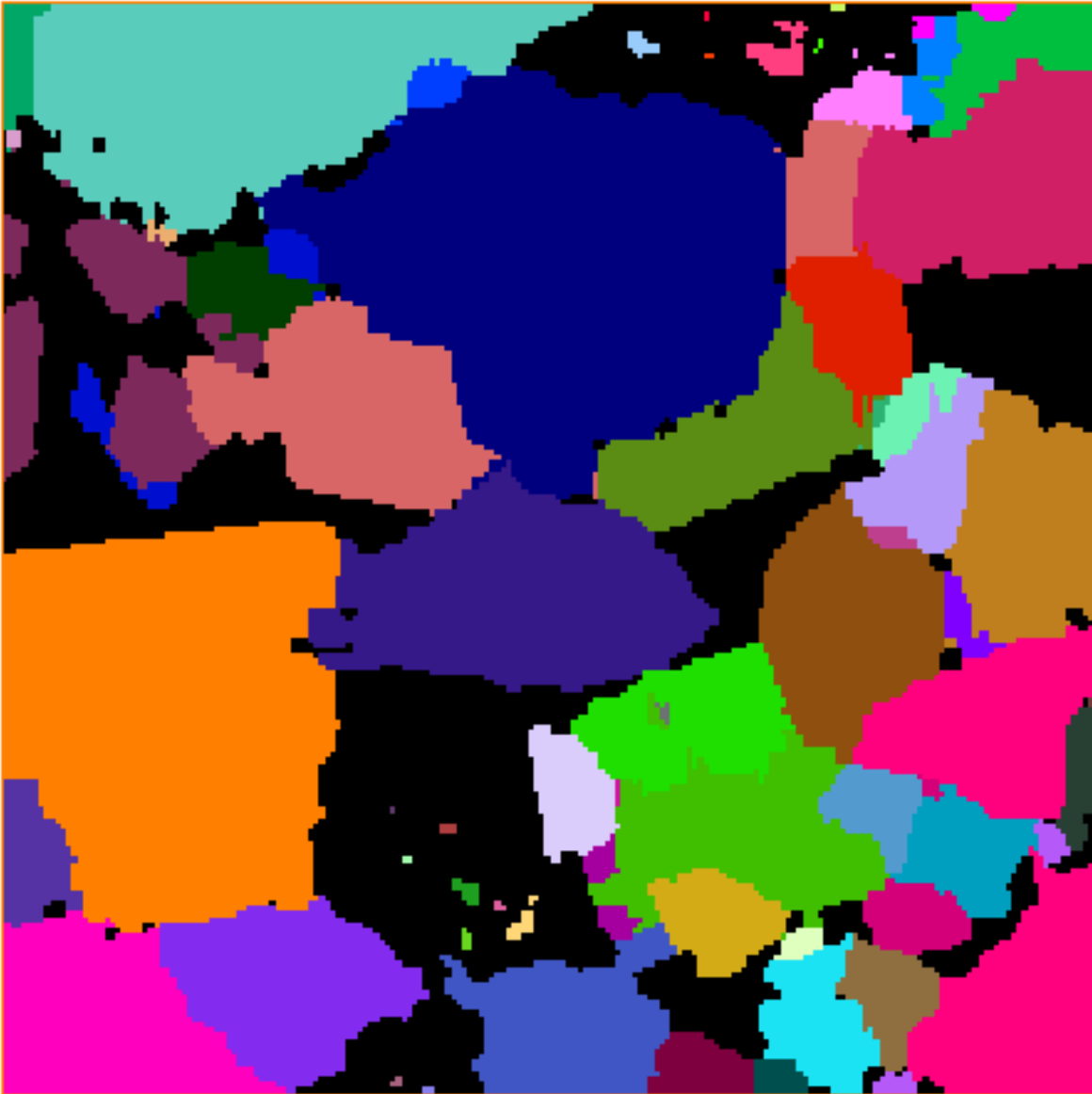
Figure 4.10. Partitioned quartz-feldspar image after 0 voxel overwrite iterations, 820 \mu m per side, 200 3 voxels
