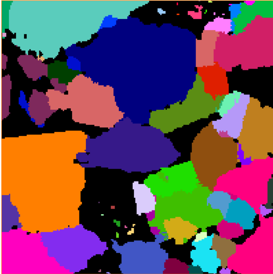
Figure 4.15. Partitioned quartz-feldspar image with 0 voxel overwrites and 10 grain assembly iterations, 820 \mu m per side, 200 3 voxels
