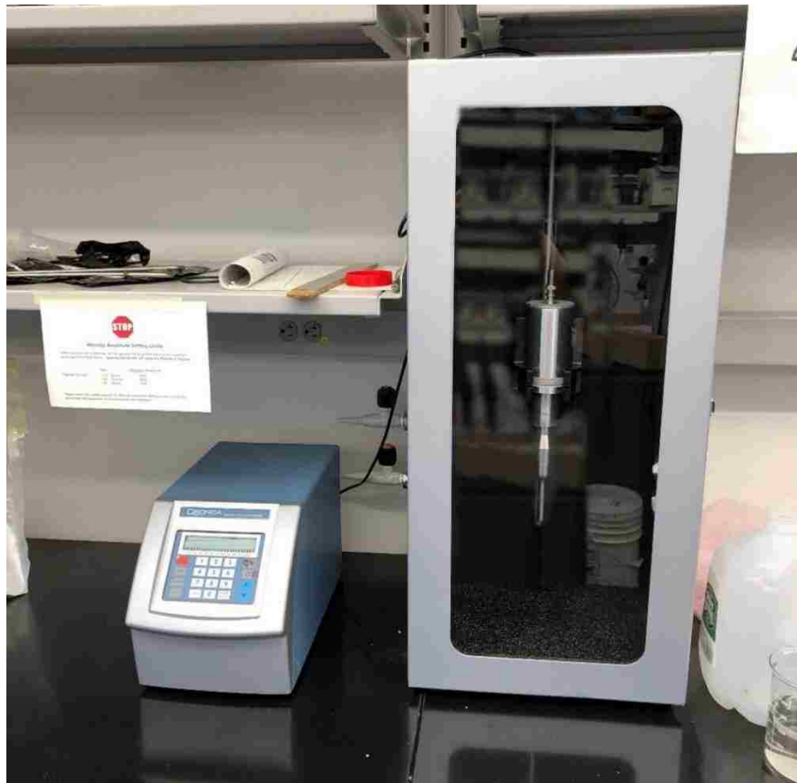
Figure 4.3. Q-Sonica Q500 Ultrasonicator used to generate each of the emulsion fluids.
