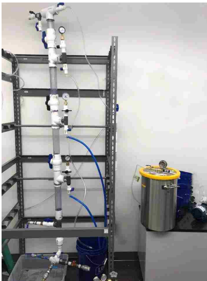
Figure 3.1. The first low-pressure prototype experimental apparatus used to develop the experimental procedures for each of the mass transfer processes and test initial concepts of future apparatus designs.
