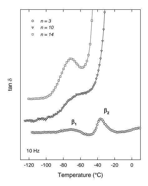
**Figure 4.5:**  $tan\delta$  versus temperature (°C) for PEGDA networks in the sub-glass transition range. Curves are offset vertically for clarity. Frequency of 10 Hz; heating rate of 1°C/min.
