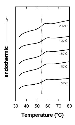
**Figure 6.2:** DSC heating sweeps (10°C min<sup>-1</sup>) for isothermally melt crystallized PTT: expanded view of glass transition region.
