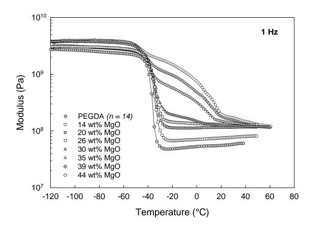
**Figure 4.35:** Dynamic mechanical storage modulus (E) versus temperature for PEGDA networks with varying MgO (wt%) loading. Frequency of 1 Hz; heating rate of 1°C/min.
