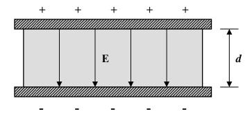
**Figure 3.9:** Parallel-plate capacitor arrangement for a dielectric material of thickness d, placed in an electric field E.
