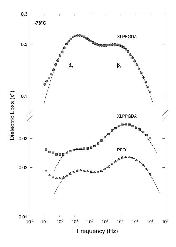
**Figure 5.7:** Dielectric loss ( $\varepsilon''$ ) vs. frequency (Hz) for XLPEGDA, XLPPGDA and PEO at -78°C. Solid curves are dual HN fits.
