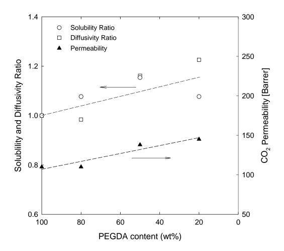
**Figure 4.33:** CO<sub>2</sub> transport properties determined at 35°C and infinite dilution for PEGDA/water networks. Solubility, diffusivity ratios defined relative to values for 100% PEGDA (n=14): S = 1.3 cm<sup>3</sup>(STP)/(cm<sup>3</sup>-atm), D = 6.2 x 10<sup>-7</sup> cm<sup>2</sup>/s. <sup>115</sup>
