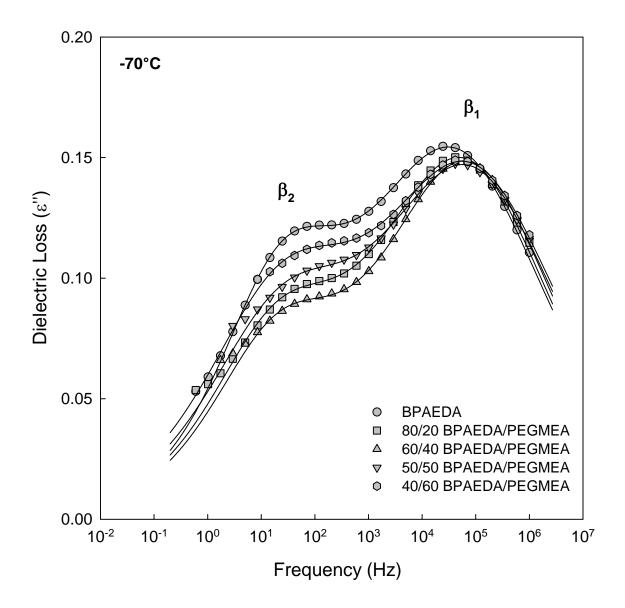
**Figure 5.38:** Dielectric loss ( $\varepsilon'$ ) vs. frequency for BPAEDA/PEGMEA copolymer networks at -70°C. Solid curves are dual HN fits.
