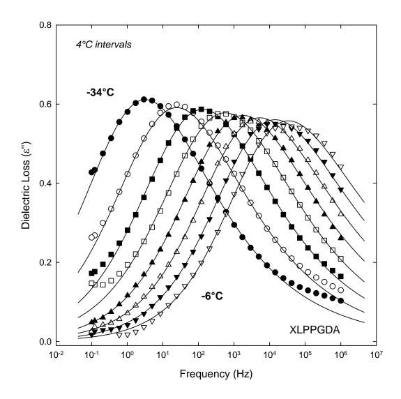
**Figure 5.11:** Dielectric loss ( $\varepsilon''$ ) vs. frequency (Hz) for XLPPGDA; temperatures from - 34°C to -6°C at 4°C intervals. Solid curves are HN fits.
