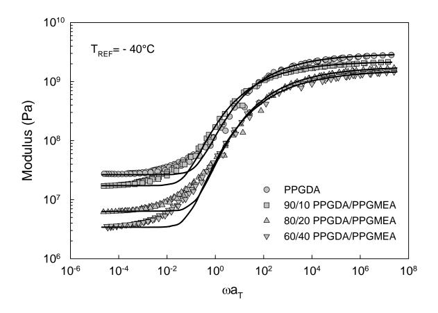
**Figure 4.26:** Time-temperature master curves for PPGDA/PPGMEA copolymer networks;  $T_{REF} = -40$ °C. Solid curves are KWW best fits.
