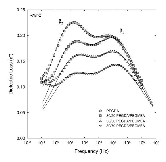
**Figure 5.17:** Dielectric loss ( $\varepsilon''$ ) vs. frequency for PEGDA/PEGMEA copolymer networks at -78°C. Solid curves are dual HN fits.
