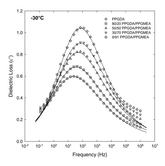
**Figure 5.32:** Dielectric loss ( $\varepsilon'$ ) vs. frequency for PPGDA/PPGMEA copolymer networks at -30°C. Solid curves are dual HN fits.
