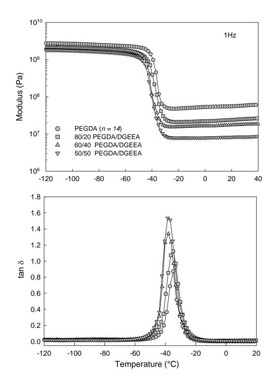
**Figure 4.22:** Dynamic mechanical properties  $(E'; tan \delta)$  versus temperature for PEGDA/DGEEA copolymer networks. Frequency of 1 Hz; heating rate of 1°C/min.
