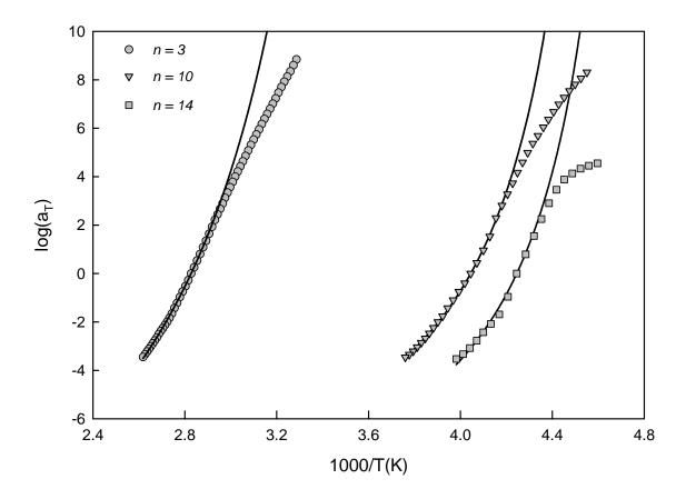
**Figure 4.8:** Arrhenius plots of  $log(a_T)$  versus 1000/T(K) for PEGDA networks. Solid curves are WLF fits.
