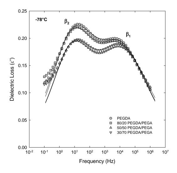
**Figure 5.20:** Dielectric loss ( $\varepsilon''$ ) vs. frequency for PEGDA/PEGA copolymer networks at -78°C. Solid curves are dual HN fits.
