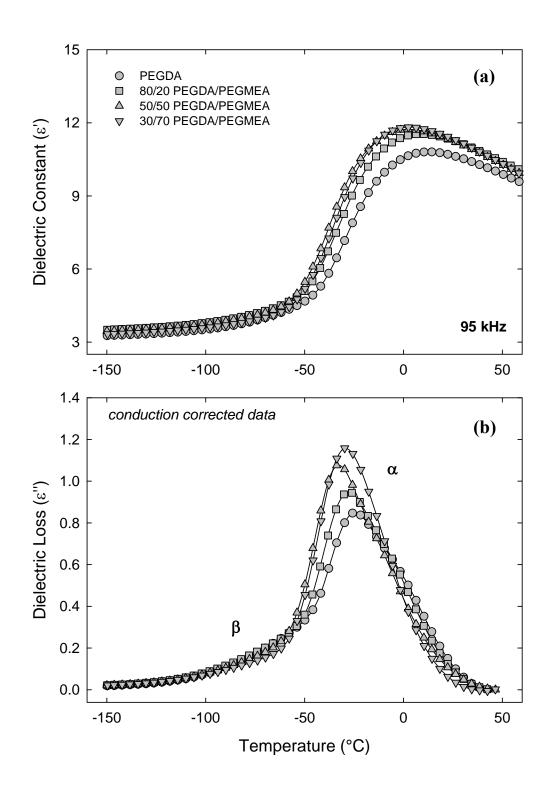
**Figure 5.14:** Dielectric properties of PEGDA/PEGMEA copolymer networks: (a) dielectric constant ( $\varepsilon$ '); (b) dielectric loss ( $\varepsilon$ ") vs. temperature. Frequency of 95 kHz. Dielectric loss data corrected for conduction.
