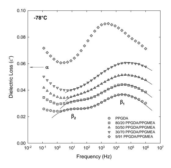
**Figure 5.31:** Dielectric loss ( $\varepsilon'$ ) vs. frequency for PPGDA/PPGMEA copolymer networks at -78°C. Solid curves are dual HN fits.
