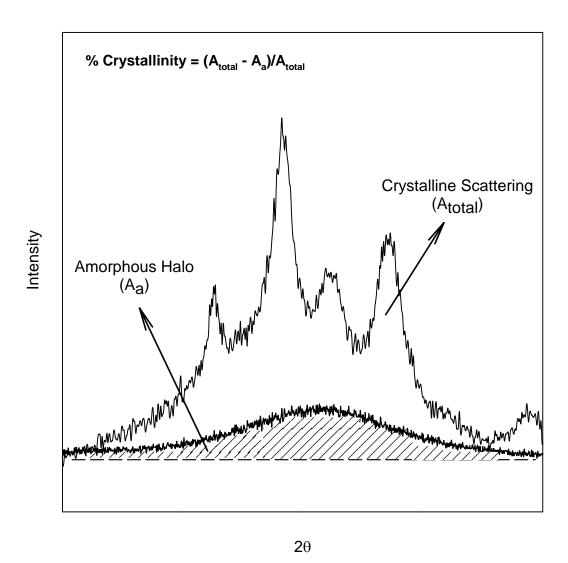
**Figure 3.18:** Typical WAXS pattern for a semicrystalline polymer plotted as intensity versus scattering angle  $(2\theta)$ .
