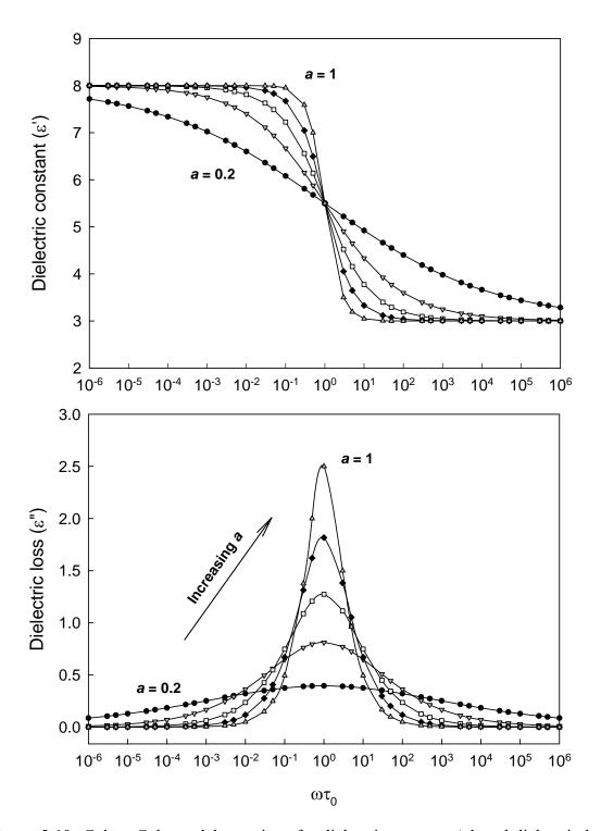
**Figure 3.10:** Cole – Cole model equations for dielectric constant ( $\varepsilon'$ ) and dielectric loss ( $\varepsilon''$ ) plotted versus  $\omega \tau_0$  on a semi-logarithmic plot (see Equation 3.17). Broadening parameter (a) = 1 gives the Debye model. For this example,  $\varepsilon_U$  = 3,  $\varepsilon_R$  = 8 and a = 0.2, 0.4, 0.6, 0.8 and 1.
