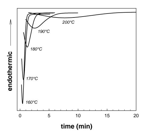
**Figure 6.3:** DSC heating sweeps (10°C min<sup>-1</sup>) for isothermally melt crystallized PTT plotted versus time. Samples quenched from melt (260°C) at 80°C/min.
