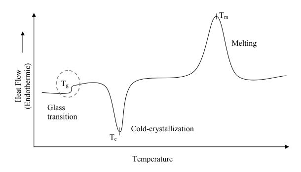
**Figure 3.16:** Typical DSC scan for a semicrystalline polymer. *Inset:* Expanded view of glass-rubber transition and estimation of  $T_g$ .
