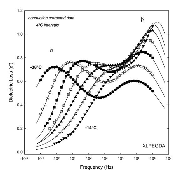
**Figure 5.10:** Dielectric loss ( $\varepsilon''$ ) vs. frequency (Hz) for XLPEGDA; temperatures from - 38°C to -14°C at 4°C intervals. Data are corrected for conduction contribution according to equation 5.2. Solid curves are dual HN fits.
