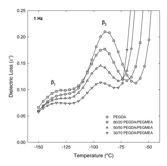
**Figure 5.16:** Dielectric loss ( $\varepsilon'$ ) vs. temperature for PEGDA/PEGMEA copolymer networks across the sub-glass transition region. Frequency of 1 Hz.
