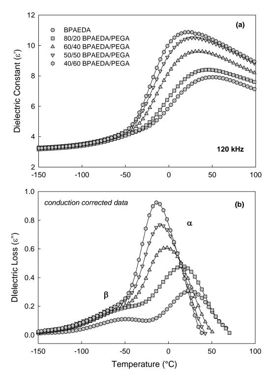
**Figure 5.37:** Dielectric properties of BPAEDA/PEGA copolymer networks: (a) dielectric constant ( $\varepsilon'$ ); (b) dielectric loss ( $\varepsilon''$ ) vs. temperature. Frequency of 120 kHz. Dielectric loss data corrected for conduction.
