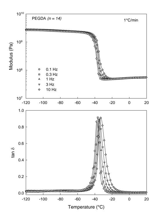
**Figure 4.2:** Dynamic mechanical properties  $(E', tan\delta)$  versus temperature for 100% PEGDA (n=14) network; heating rate of 1°C/min.
