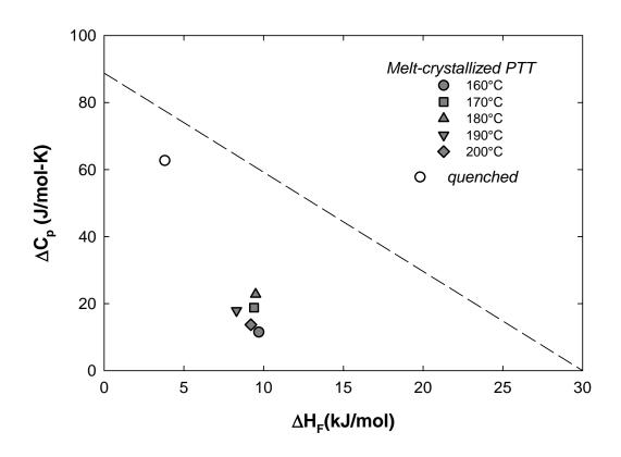
**Figure 6.4:** Incremental increase in heat capacity  $(\Delta C_p(T_g); \text{ J/mol-K})$  versus net heat of fusion  $(\Delta H_F; \text{ kJ/mol})$  for melt crystallized PTT.
