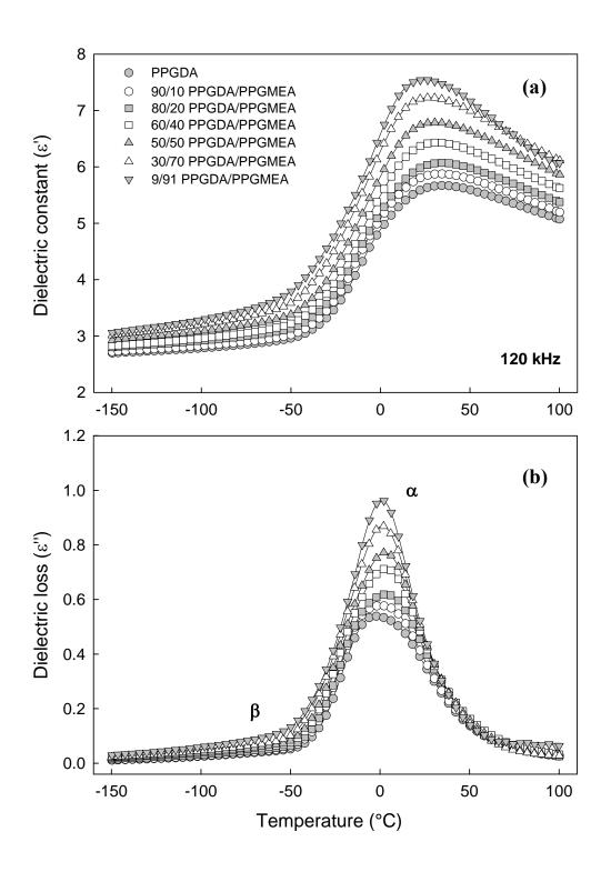
**Figure 5.30:** Dielectric properties of PPGDA/PPGMEA copolymer networks: (a) dielectric constant ( $\varepsilon$ '); (b) dielectric loss ( $\varepsilon$ '') vs. temperature. Frequency of 120 kHz.
