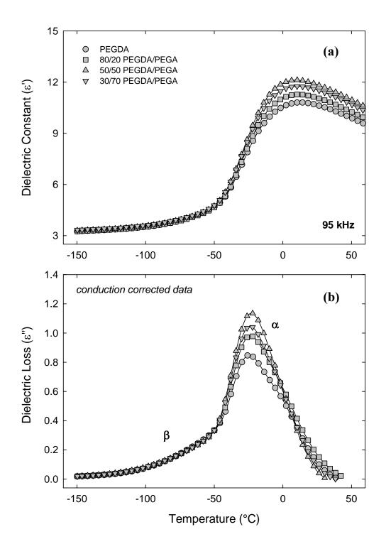
**Figure 5.15:** Dielectric properties of PEGDA/PEGA copolymer networks: (a) dielectric constant ( $\varepsilon$ '); (b) dielectric loss ( $\varepsilon$ '') vs. temperature. Frequency of 95 kHz. Dielectric loss data corrected for conduction.
