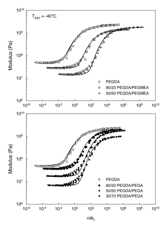
**Figure 4.16:** Time-temperature master curves for PEGDA copolymer networks;  $T_{REF} = -40$ °C. Solid curves are KWW best fits.
