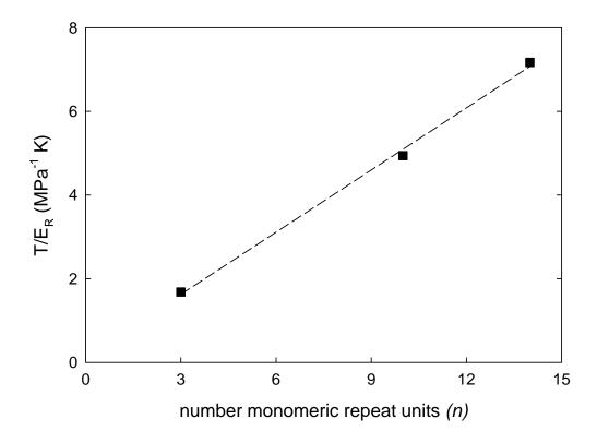
**Figure 4.4:** Ratio of temperature/rubbery modulus  $[T(K)/E_R]$  for PEGDA networks with varying ethylene oxide repeat length, n. Values of the rubbery modulus,  $E_R$ , established from time-temperature master curves.
