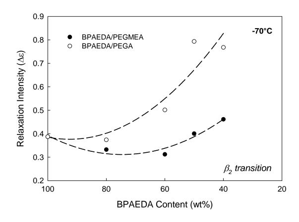
**Figure 5.40:** Dielectric relaxation intensity ( $\Delta \varepsilon$ , determined from HN fits) vs. BPAEDA content (wt%) for BPAEDA/PEGMEA and BPAEDA/PEGA copolymer networks.  $\beta_2$  sub-glass transition at -70°C.
