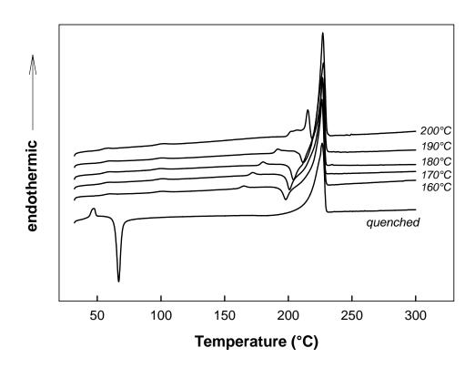
**Figure 6.1:** DSC heating sweeps (10°C min<sup>-1</sup>) for quenched and isothermally melt crystallized PTT.
