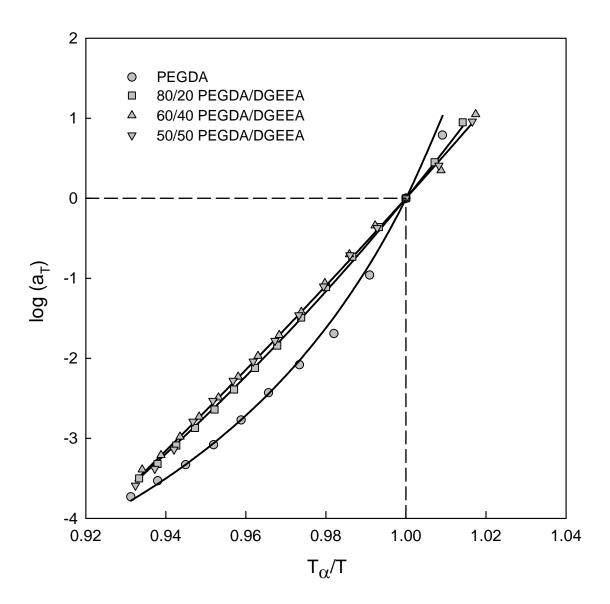
**Figure 4.24:** Cooperativity plots  $(\log(a_T) \text{ versus } T_{\alpha}/T)$  for PEGDA/DGEEA copolymer networks. Solid curves are WLF fits.
