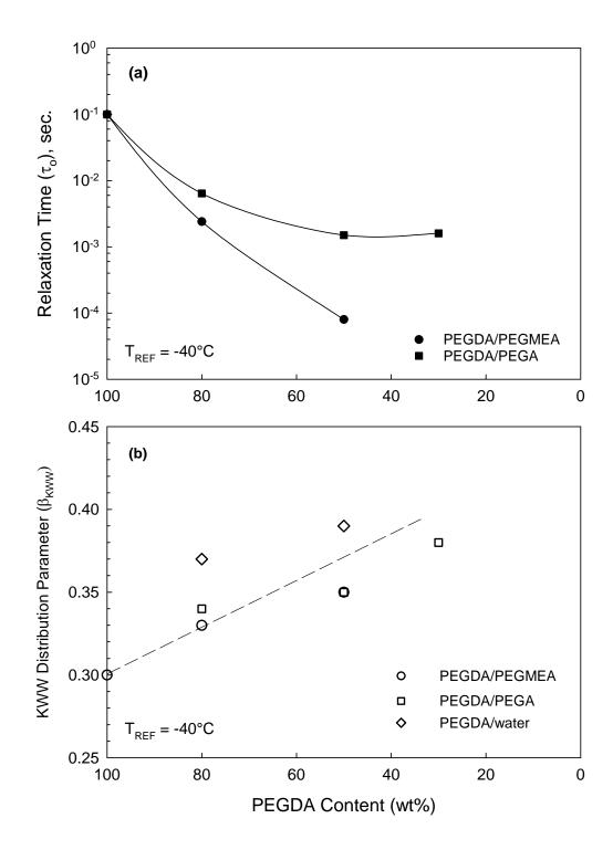
**Figure 4.18:** KWW parameters for the glass-rubber relaxation in PEGDA networks;  $T_{REF} = -40^{\circ}\text{C}$ . (a) Relaxation time ( $\tau_o$ , sec) versus PEGDA content; (b) Distribution parameter ( $\beta_{KWW}$ ) versus PEGDA content.
