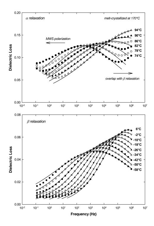
**Figure 6.13:** Dielectric loss ( $\varepsilon''$ ) versus frequency for melt crystallized ( $T_c = 170^{\circ}$ C) PTT across the glass-rubber ( $\alpha$ ) and sub-glass ( $\beta$ ) relaxation regions. Solid curves are Havriliak-Negami best fits.
