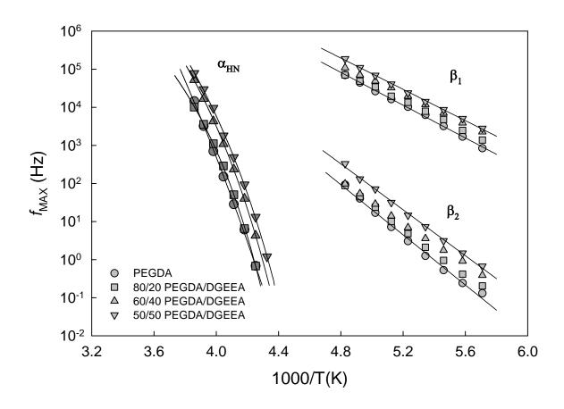
**Figure 5.28:** Arrhenius plot of  $f_{MAX}$  (Hz) vs. 1000/T(K) for PEGDA/DGEEA copolymer networks.
