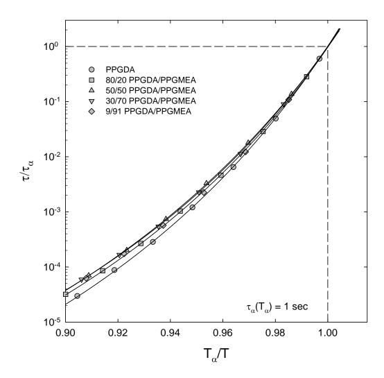
**Figure 5.33:** Cooperativity plots of  $\tau/\tau_{\alpha}$  vs.  $T_{\alpha}/T$  for PPGDA/PPGMEA copolymer networks. Solid curves are WLF fits.
