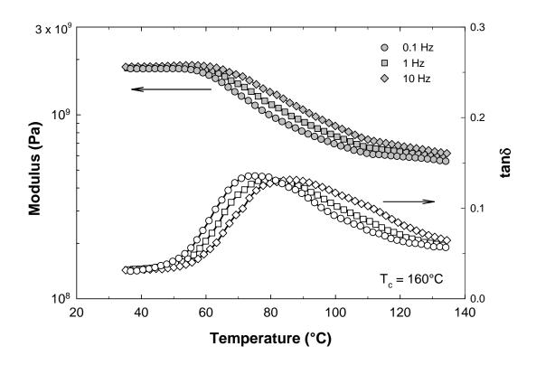
**Figure 6.7:** Dynamic mechanical storage modulus (filled symbols) and loss factor  $(tan \delta)$  (empty symbols) versus temperature for melt crystallized  $(T_c = 160^{\circ}\text{C})$  PTT; heating rate of 1°C min<sup>-1</sup>.
