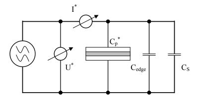
**Figure 3.14:** Schematic of the measurement circuit for the BDS Novocontrol Concept 40 spectrometer.
