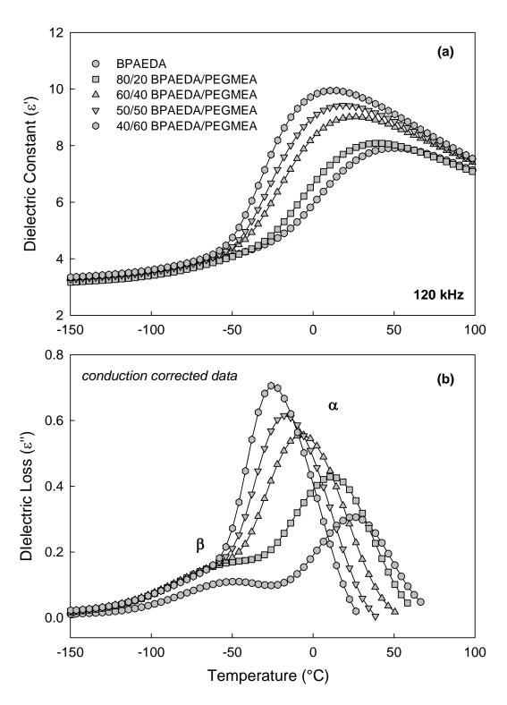
**Figure 5.36:** Dielectric properties of BPAEDA/PEGMEA copolymer networks: (a) dielectric constant ( $\varepsilon$ '); (b) dielectric loss ( $\varepsilon$ ') vs. temperature. Frequency of 120 kHz. Dielectric loss data corrected for conduction.
