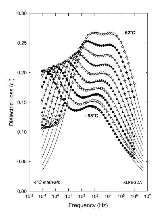
**Figure 5.6:** Dielectric loss ( $\varepsilon'$ ) vs. frequency (Hz) for XLPEGDA; temperatures from - 98°C to -62°C at 4°C intervals. Solid curves are dual HN fits.
