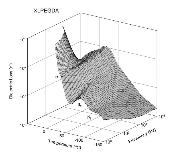
**Figure 5.2:** Contour plot of dielectric loss ( $\varepsilon'$ ) vs. temperature (°C) vs. frequency (Hz) for XLPEGDA network.
