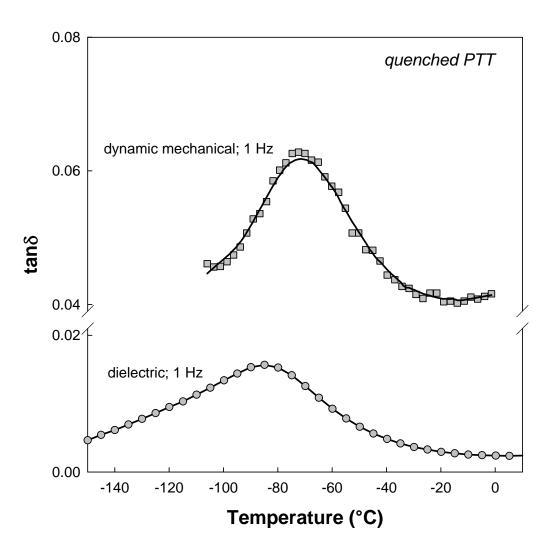
**Figure 6.15:** Comparison of  $tan\delta$  versus temperature curves for quenched PTT; 1 Hz.
