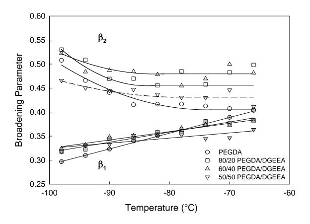
**Figure 5.27:** Havriliak-Negami [HN] broadening parameter vs. temperature for PEGDA/DGEEA copolymer networks.  $\beta_1$  and  $\beta_2$  sub-glass transitions.
