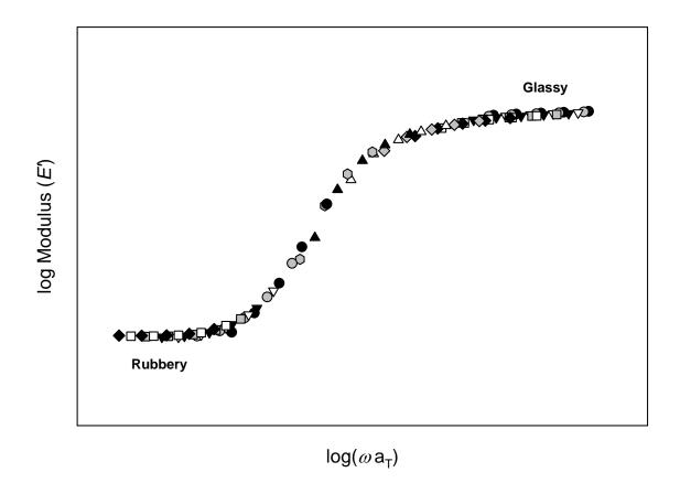
**Figure 3.4:** Modulus-frequency master curve obtained by time-temperature superposition; groups of data points (*i.e.*, same symbols) correspond to discrete temperatures.
