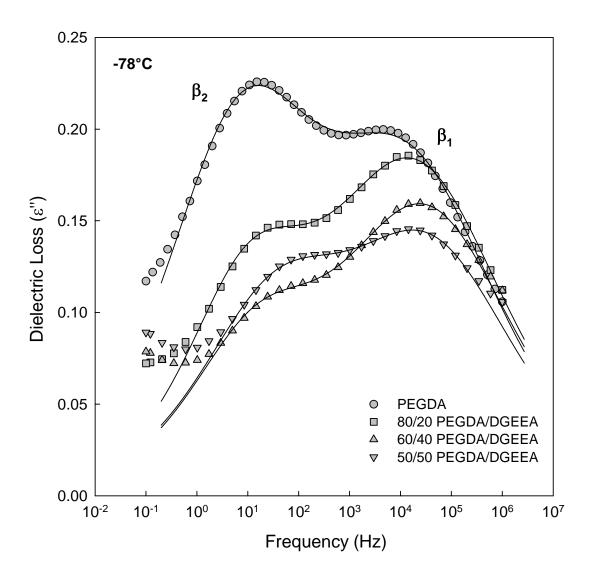
**Figure 5.25:** Dielectric loss ( $\varepsilon''$ ) vs. frequency for PEGDA/DGEEA copolymer networks at -78°C. Solid curves are dual HN fits.
