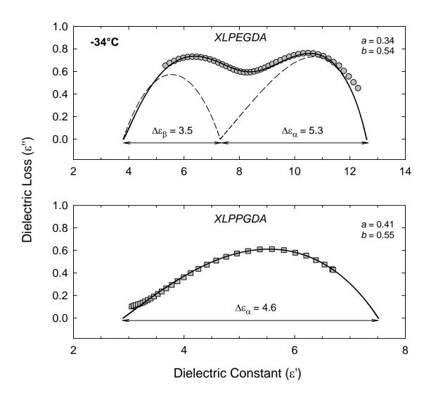
**Figure 5.12:** Cole-Cole plots of dielectric loss ( $\varepsilon'$ ) vs. dielectric constant ( $\varepsilon'$ ) for XLPEGDA and XLPPGDA at -34°C. Solid curve is HN best fit. HN fit parameters (a,b) for the glass-rubber relaxation are as indicated.
