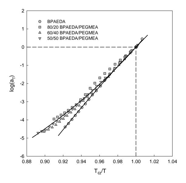
**Figure 4.31:** Cooperativity plots  $(\log(a_T) \text{ versus } T_{\alpha}/T)$  for BPAEDA/PEGMEA copolymer networks. Solid curves are WLF fits.
