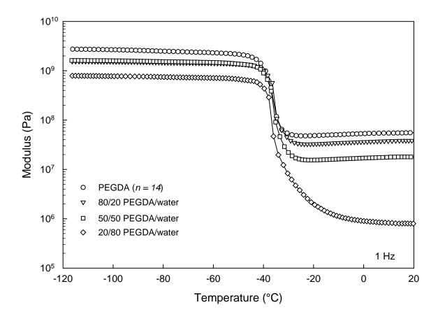
**Figure 4.9:** Storage modulus versus temperature for PEGDA (n=14) networks with varying amounts of water in the initial reaction mixture. Frequency of 1 Hz; heating rate of 1°C/min.
