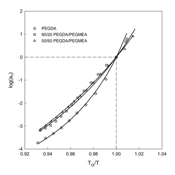
**Figure 4.19:** Cooperativity plots ( $\log(a_T)$  versus  $T_{\alpha}/T$ ) for PEGDA/PEGMEA copolymer networks. Solid curves are WLF fits.
