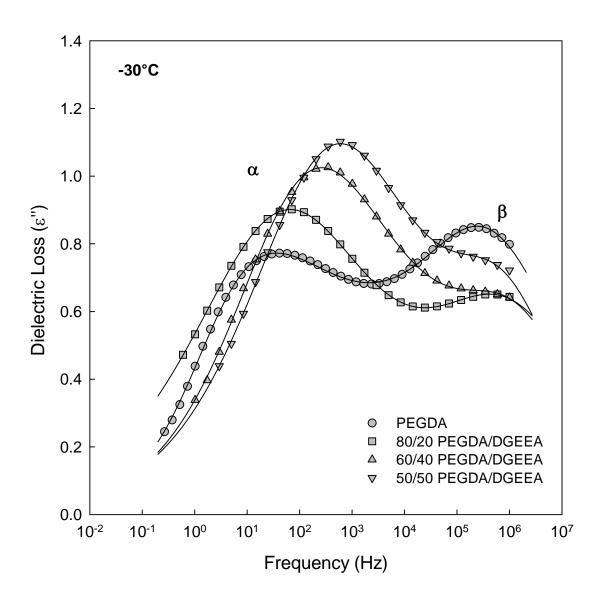
**Figure 5.29:** Dielectric loss ( $\varepsilon''$ ) vs. frequency for PEGDA/DGEEA copolymer networks at -30°C. Solid curves are dual HN fits.
