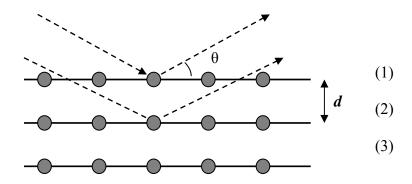
**Figure 3.17:** Elastic scattering of X-rays from parallel crystal planes (1, 2 & 3) with a characteristic spacing d.
