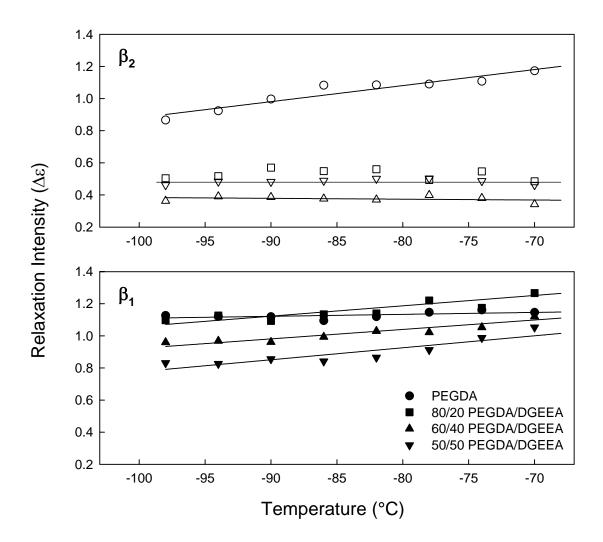
**Figure 5.26:** Dielectric relaxation intensity ( $\Delta \varepsilon$ , determined from HN fits) vs. temperature for PEGDA/DGEEA copolymer networks.  $\beta_1$  and  $\beta_2$  sub-glass transitions.
