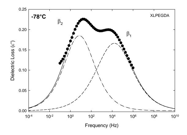
**Figure 5.5:** Dielectric loss ( $\varepsilon''$ ) vs. frequency (Hz) for XLPEGDA at -78°C. Solid curve is dual HN fit; dashed curves are individual HN fits for the  $\beta_1$  and  $\beta_2$  relaxations.
