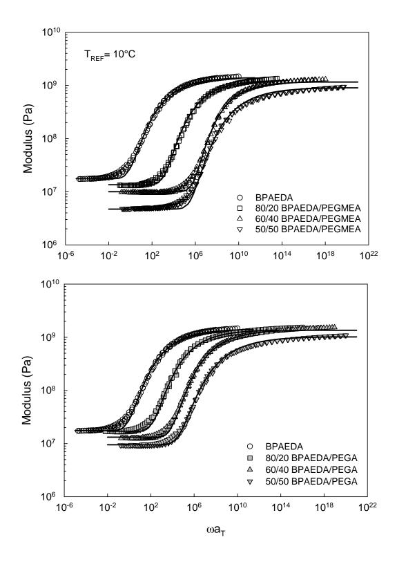
**Figure 4.30:** Time-temperature master curves for BPAEDA copolymer networks;  $T_{REF} = 10^{\circ}$ C. Solid curves are KWW best fits.
