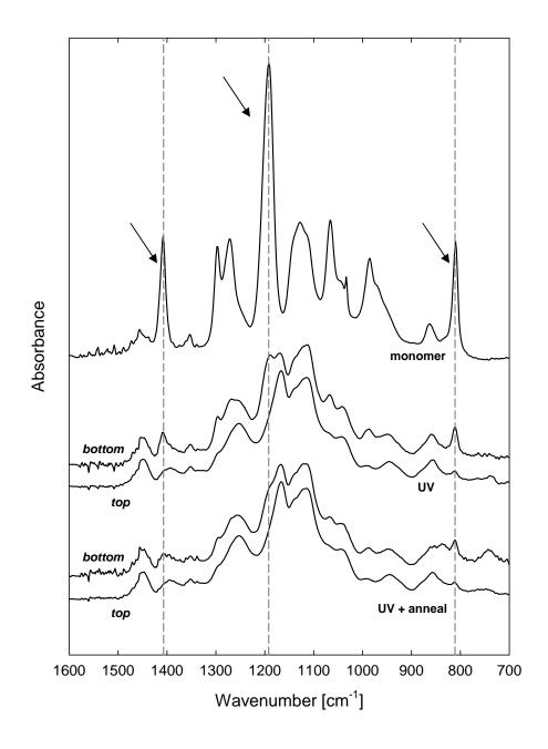
**Figure 4.1:** FTIR spectra of liquid PEGDA and solid crosslinked PEGDA films (n=3). For the solid polymer films, one side was exposed directly to UV light ("top"), and the other side was positioned opposite to the UV source ("bottom"). Annealed films were held at  $100^{\circ}$ C for one hour after UV exposure.
