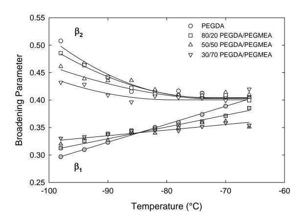
**Figure 5.19:** Havriliak-Negami [HN] broadening parameter vs. temperature for PEGDA/PEGMEA copolymer networks.  $\beta_1$  and  $\beta_2$  sub-glass transitions.
