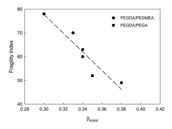
**Figure 4.21:** Fragility index (m), as defined in Eq. 2.11, versus KWW distribution parameter  $(\beta_{KWW})$  for PEGDA copolymer networks.
