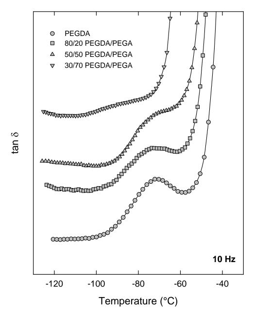
**Figure 4.15:**  $tan\delta$  versus temperature for PEGDA/PEGA networks in the sub-glass transition range. Curves are offset vertically for clarity. Frequency of 10 Hz; heating rate of 1°C/min.
