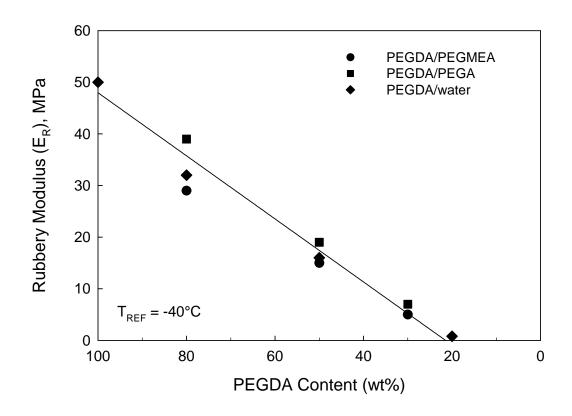
**Figure 4.17:** Rubbery modulus ( $E_R$ , MPa) versus PEGDA content for PEGDA/PEGMEA, PEGDA/PEGA, and PEGDA/water networks.  $E_R$  evaluated from time-temperature master curves at -40°C.
