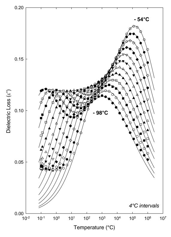
**Figure 5.35:** Dielectric loss ( $\varepsilon''$ ) vs. frequency (Hz) for XLBPAEDA; temperatures from -98°C to -54°C at 4°C intervals. Solid curves are dual HN fits.
