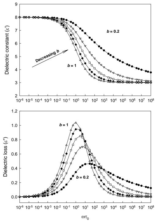
**Figure 3.11:** Havriliak – Negami model equations for dielectric constant ( $\varepsilon'$ ) and dielectric loss ( $\varepsilon''$ ) plotted versus  $\omega \tau_0$  on a semi-logarithmic plot (see Equation 2.10). Broadening parameter (a) = 0.5. Skewing parameter (b) = 1 gives the Cole-Cole model. For this example,  $\varepsilon_U = 3$ ,  $\varepsilon_R = 8$  and b = 0.2, 0.4, 0.6, 0.8 and 1.
