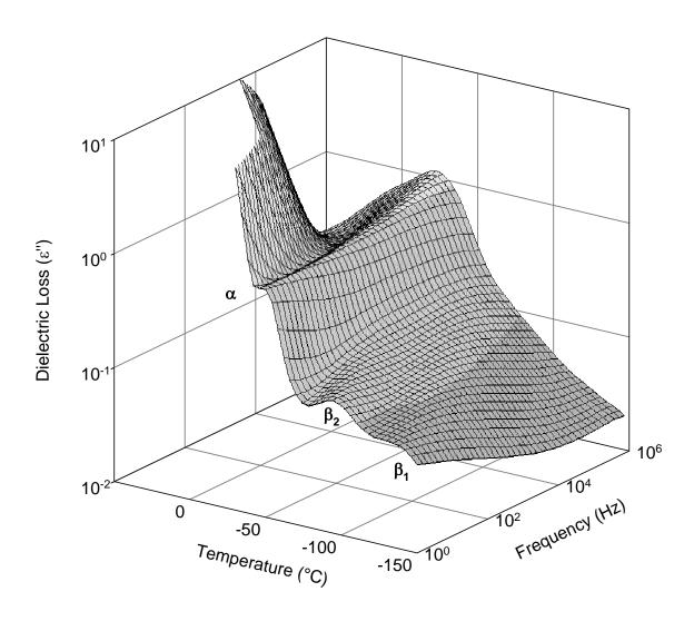
**Figure 5.13:** Contour plot of dielectric loss ( $\varepsilon''$ ) vs. temperature (°C) vs. frequency (Hz) for 50/50 (wt%) PEGDA/PEGMEA network.
