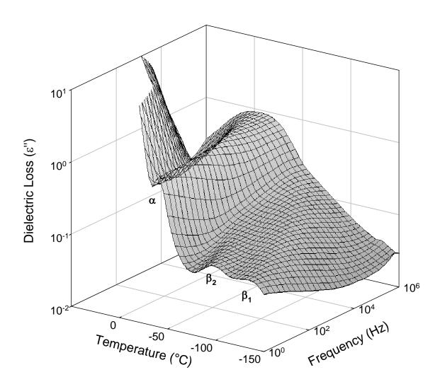
**Figure 5.24:** Contour plot of dielectric loss ( $\varepsilon''$ ) vs. temperature (°C) vs. frequency (Hz) for 60/40 (wt%) PEGDA/DGEEA copolymer network.
