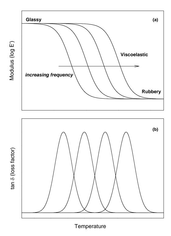
**Figure 3.8:** Representative dynamic mechanical (DMA) result for a polymeric material across the glass transition, plotted as a function of temperature for varying frequencies; (a): Storage modulus (E'), (b):  $\tan \delta$  (loss factor).
