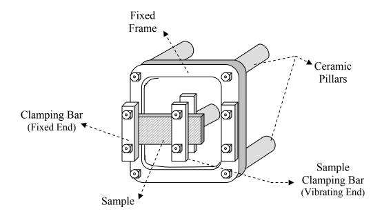
**Figure 3.7:** Single cantilever arrangement of a sample in the DMTA.
