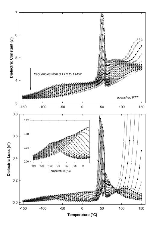
**Figure 6.10:** Dielectric constant ( $\varepsilon$ ') and loss ( $\varepsilon$ '') versus temperature for quenched PTT; selected frequencies from 0.1 Hz to 1 MHz. *Inset*: expanded view of dielectric loss across the sub-glass transition region.
