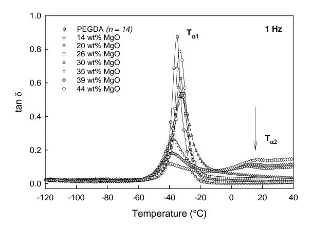
**Figure 4.36:** Dynamic mechanical loss factor  $(tan\delta)$  versus temperature for PEGDA networks with varying MgO (wt%) loading. Frequency of 1 Hz; heating rate of 1°C/min.
