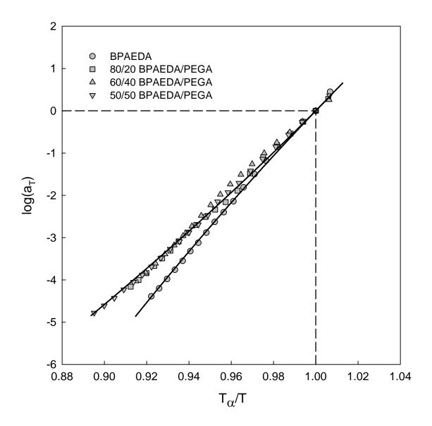
**Figure 4.32:** Cooperativity plots ( $\log(a_T)$  versus  $T_{\alpha}/T$ ) for BPAEDA/PEGA copolymer networks. Solid curves are WLF fits.
