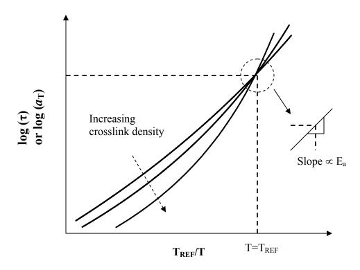
**Figure 2.6:** Schematic of the Fragility or Cooperativity plot  $(\log(\tau))$  or  $\log(a_T)$  versus  $T_{REF}/T$ ) showing the temperature sensitivity of the glass-rubber relaxation process as a function of crosslink density.
