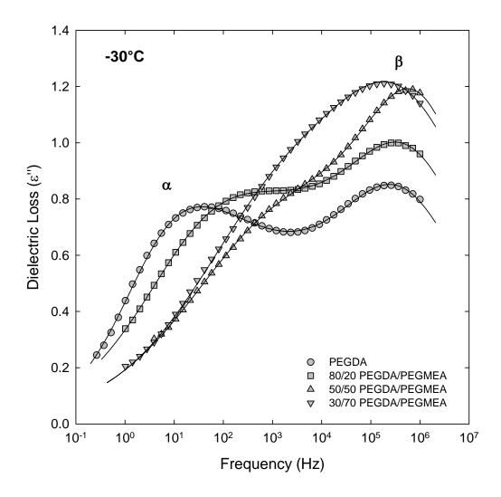
**Figure 5.22:** Dielectric loss ( $\varepsilon''$ ) vs. frequency for PEGDA/PEGMEA copolymer networks at -30°C. Data are corrected for conduction contribution according to Equation 5.2. Solid curves are dual HN fits.
