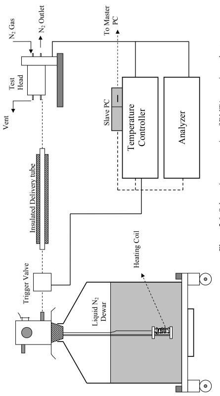
Figure 3.6: Schematic representation of DMTA experimental set-up.
