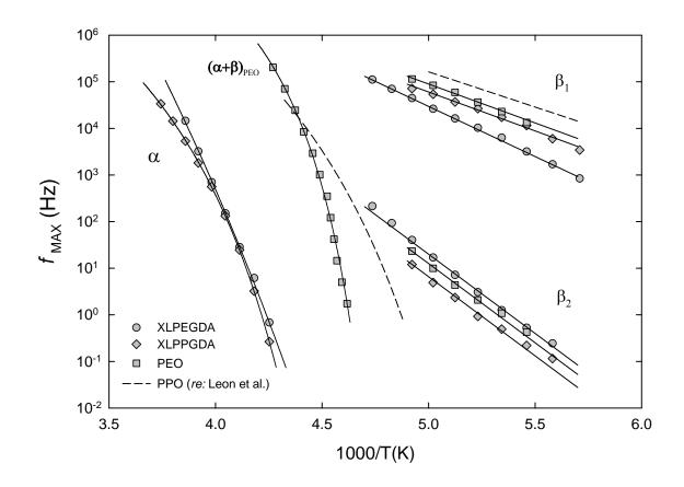
**Figure 5.9:** Arrhenius plot of  $f_{MAX}$  (Hz) vs. 1000/T(K) for XLPEGDA, XLPPGDA and PEO. Dashed lines correspond to data for PPO polymer (see ref. 151).
