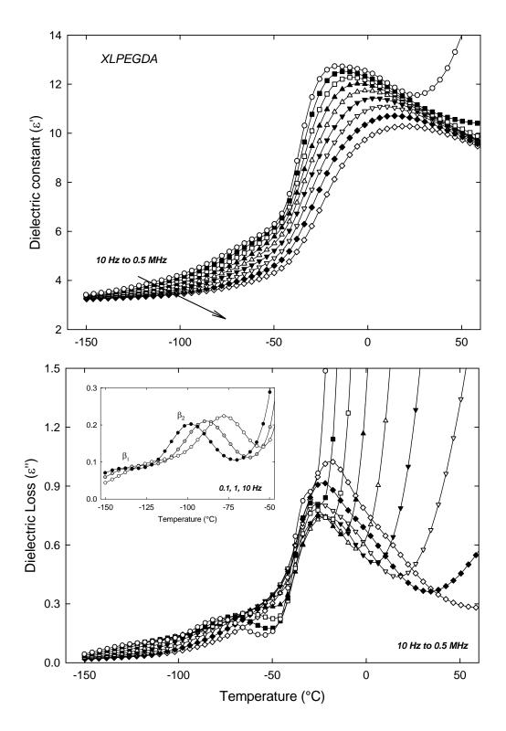
**Figure 5.1:** Dielectric constant ( $\varepsilon'$ ) and loss ( $\varepsilon''$ ) vs. temperature for XLPEGDA; selected frequencies from 10 Hz to 0.5 MHz. *Inset*: expanded view of dielectric loss across the sub-glass region at 0.1, 1, and 10 Hz.
