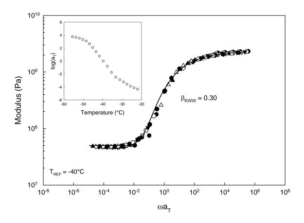
**Figure 4.6:** Time-temperature master curve for PEGDA (n=14) network;  $T_{REF} = -40$ °C. Solid curve is KWW best-fit. *Inset:* log(shift factor,  $a_T$ ) versus temperature (°C).
