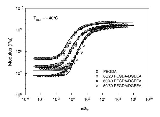
**Figure 4.23:** Time-temperature master curves for PEGDA/DGEEA copolymer networks;  $T_{REF} = -40$ °C. Solid curves are KWW best fits.
