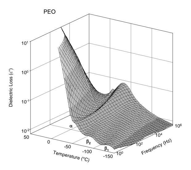
**Figure 5.4:** Contour plot of dielectric loss ( $\varepsilon'$ ) vs. temperature (°C) vs. frequency (Hz) for PEO network.
