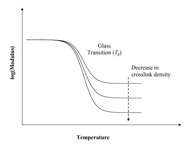
**Figure 2.4:** Schematic showing the typical modulus behavior for crosslinked networks with decreasing crosslink density.
