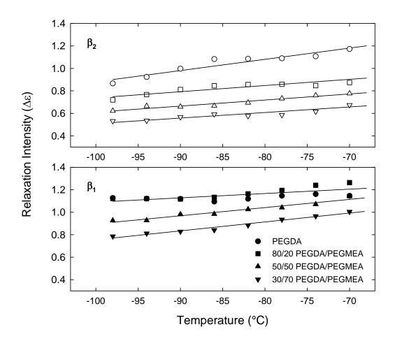
**Figure 5.18:** Dielectric relaxation intensity ( $\Delta \varepsilon$ , determined from HN fits) vs. temperature for PEGDA/PEGMEA copolymer networks.  $\beta_1$  and  $\beta_2$  sub-glass transitions.
