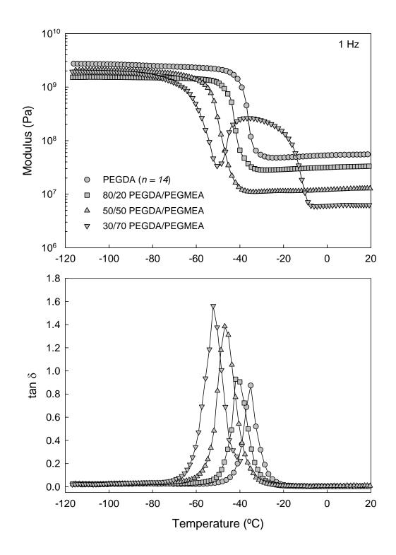
**Figure 4.12:** Dynamic mechanical properties  $(E'; tan\delta)$  versus temperature for PEGDA/PEGMEA copolymer networks. Frequency of 1 Hz; heating rate of 1°C/min.
