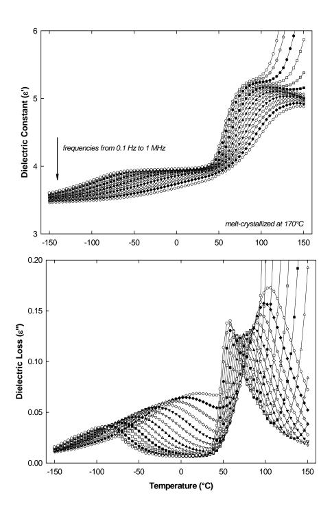
**Figure 6.11:** Dielectric constant ( $\varepsilon'$ ) and loss ( $\varepsilon''$ ) versus temperature for melt crystallized ( $T_c = 170$ °C) PTT; selected frequencies from 0.1 Hz to 1 MHz.
