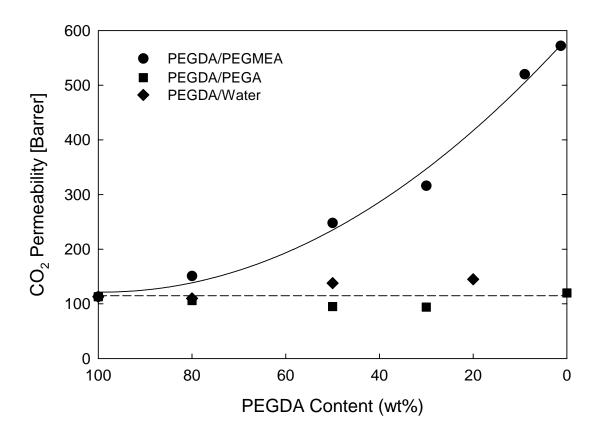
**Figure 4.34:**  $CO_2$  permeability (Barrer) determined at 35°C and infinite dilution for PEGDA networks. <sup>115,124</sup> 1 Barrer =  $10^{-10}$  cm<sup>3</sup>(STP) cm/(cm<sup>2</sup>s cm-Hg).
