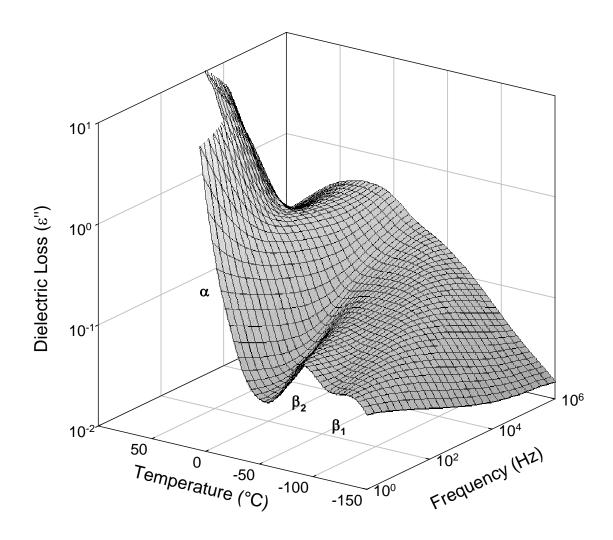
**Figure 5.34:** Contour plot of dielectric loss ( $\varepsilon''$ ) vs. temperature (°C) vs. frequency (Hz) for XLBPAEDA network.
