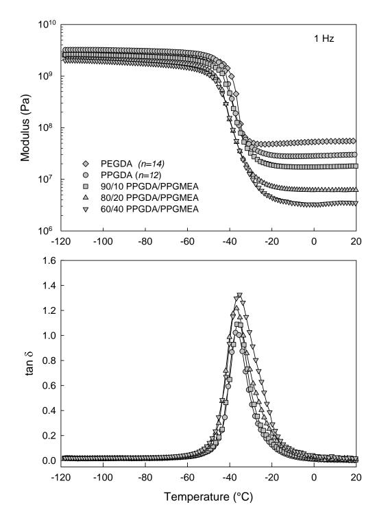
**Figure 4.25:** Dynamic mechanical properties (E';  $tan\delta$ ) versus temperature for 100% PEGDA and PPGDA/PPGMEA copolymer networks. Frequency of 1 Hz; heating rate of 1°C/min.
