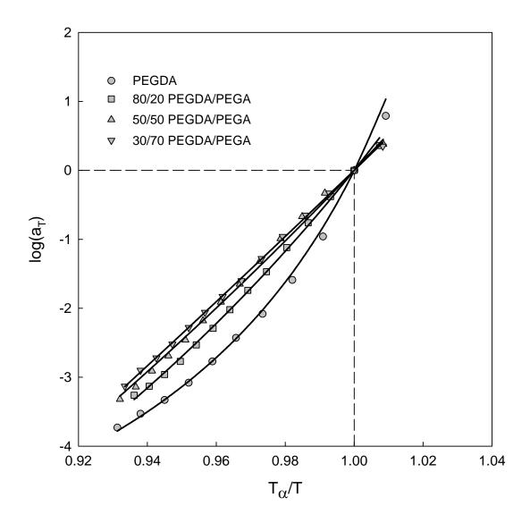
**Figure 4.20:** Cooperativity plots  $(\log(a_T) \text{ versus } T_{\alpha}/T)$  for PEGDA/PEGA copolymer networks. Solid curves are WLF fits.
