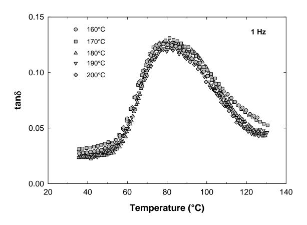
**Figure 6.9:** Dynamic mechanical  $tan\delta$  versus temperature for melt crystallized PTT. Frequency of 1 Hz; heating rate of 1°C min<sup>-1</sup>.
