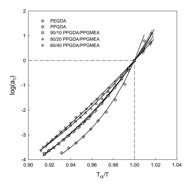
**Figure 4.27:** Cooperativity plots  $(\log(a_T) \text{ versus } T_{\mathcal{O}}/T)$  for PPGDA/PPGMEA copolymer networks. Solid curves are WLF fits.
