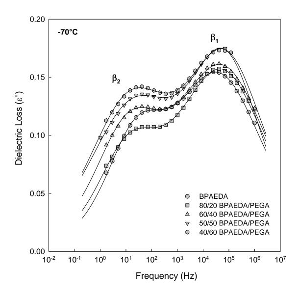
**Figure 5.39:** Dielectric loss ( $\varepsilon''$ ) vs. frequency for BPAEDA/PEGA copolymer networks at -70°C. Solid curves are dual HN fits.
