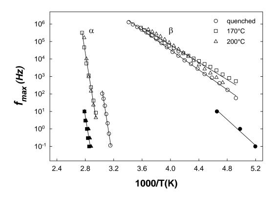
**Figure 6.14:** Arrhenius plot of  $f_{\text{MAX}}$  (Hz) versus 1000/T(K) for quenched and melt crystallized PTT. ( $\bigcirc$ ) quenched; ( $\square$ )  $T_c = 170^{\circ}\text{C}$ ; ( $\triangle$ )  $T_c = 200^{\circ}\text{C}$ . Empty symbols: dielectric results. Filled symbols: dynamic mechanical results.
