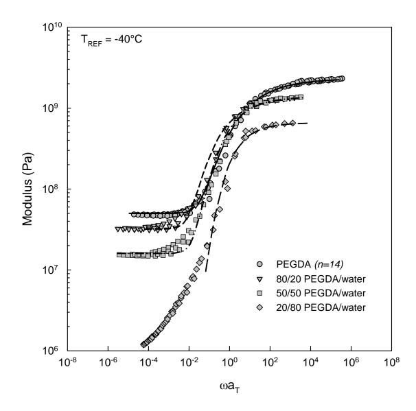
**Figure 4.10:** Time-temperature master curves for PEGDA/water networks. Curves are KWW best fits at  $T_{REF} = -40$ °C.
