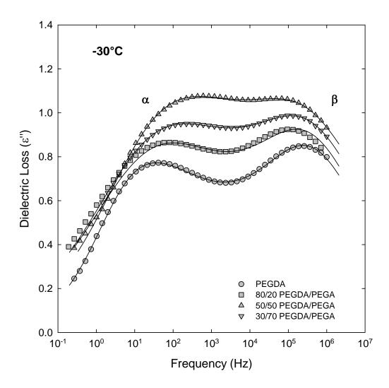
**Figure 5.23:** Dielectric loss ( $\varepsilon''$ ) vs. frequency for PEGDA/PEGA copolymer networks at -30°C. Data are corrected for conduction contribution according to Equation 5.2. Solid curves are dual HN fits.
