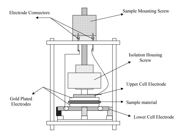
**Figure 3.13:** Novocontrol Concept 40 BDS sample cell arrangement.
