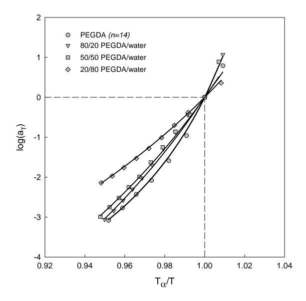
**Figure 4.11:** Cooperativity plots ( $\log(a_T)$  versus  $T_{\alpha}/T$ ) for PEGDA/water networks. Solid curves are WLF fits.
