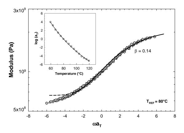
**Figure 6.8:** Time-temperature master curve for melt crystallized ( $T_c = 160$ °C) PTT;  $T_{REF} = 80$ °C. Solid curve is KWW best-fit. *Inset:* time-temperature shift factor ( $a_T$ ) versus temperature.
