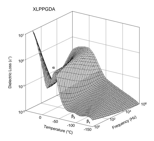
**Figure 5.3:** Contour plot of dielectric loss ( $\varepsilon'$ ) vs. temperature (°C) vs. frequency (Hz) for XLPPGDA network.
