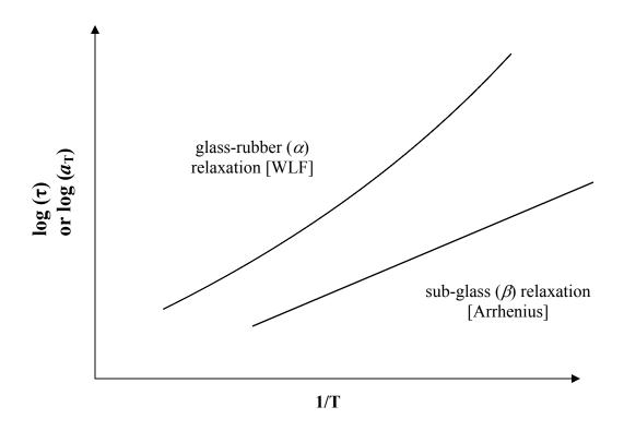
**Figure 2.5:** Arrhenius plot  $(\log(\tau) \text{ or } \log(a_T) \text{ versus } 1/T)$  showing the temperature dependence of the sub-glass and glass-rubber relaxation processes in polymer networks.
