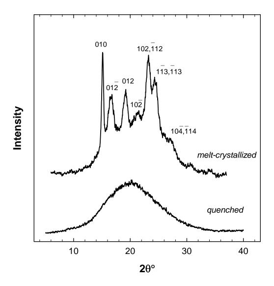
**Figure 6.5:** Wide-angle X-ray diffraction patterns (intensity versus  $2\theta$ ) for quenched and melt crystallized ( $T_c = 180^{\circ}\text{C}$ ) PTT; Cu K<sub>\alpha</sub> radiation,  $\lambda = 1.5406\text{Å}$ . Indexing of diffraction peaks as per reference 162.
