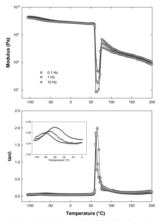
**Figure 6.6:** Dynamic mechanical storage modulus (E'; Pa) and loss factor ( $tan\delta$ ) versus temperature for quenched PTT; heating rate of 1°C min<sup>-1</sup>. *Inset:*  $tan\delta$  versus temperature for sub-glass ( $\beta$ ) transition region.
