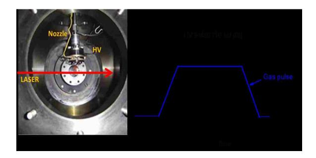
**Figure 2.2:** Schematic diagram illustrating pulsed discharge technique and high voltage (HV) pulser used to reduce background on laser induced fluorescence.
