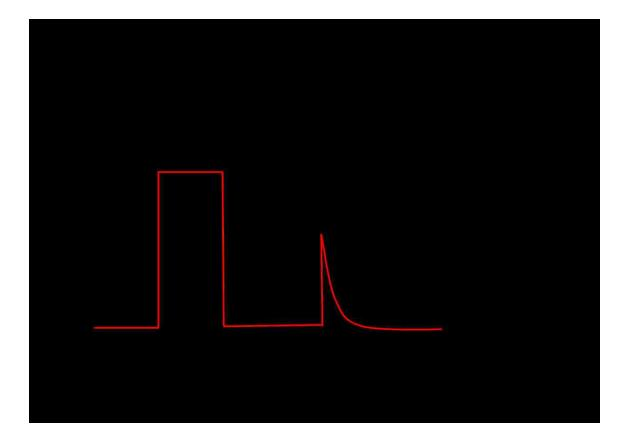
**Figure 2.3:** Schematic diagram illustrating how pulsed discharge technique and high voltage (HV) pulser separates in time the background and fluorescence.
