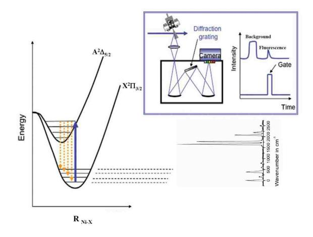
**Figure 2.5** : Illustration of the SVL emission technique applied to probe the low-lying states of nickel monohalides. Modern spectrographs are usually equipped with a gated, intensified CCD detector as shown in the figure.
