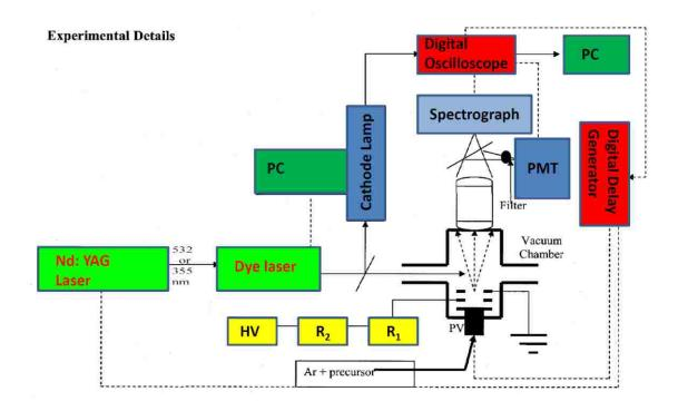
**Figure 2.1:** Generalized schematic layout of the Single Vibronic Level (SVL) emission and Laser Induced Fluorescence (LIF) experiment using pulsed lasers.
