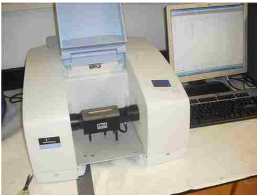
Figure 2.1 FTIR spectroscopy experimental set up for studying sorption of quercetin in polymer films. Polymer films were deposited on the Horizontal ATR prism shown in the picture
