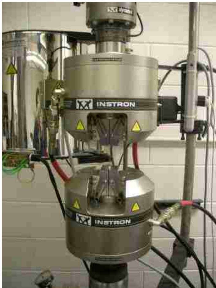
Figure 2.1 The Instron 8800 servo-hydraulic test machine used for tensile test.
