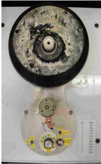
Figure 3.2 A) Shows the “in house” spin coating system used to make the ultra-thin film coatings. B) Shows the White Lightning UV source used to cure the coatings.
