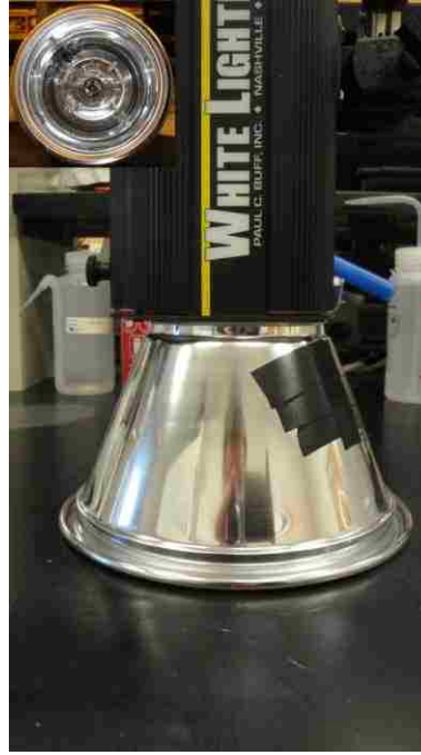
Figure 3.2 A) Shows the “in house” spin coating system used to make the ultra-thin film coatings. B) Shows the White Lightning UV source used to cure the coatings.
