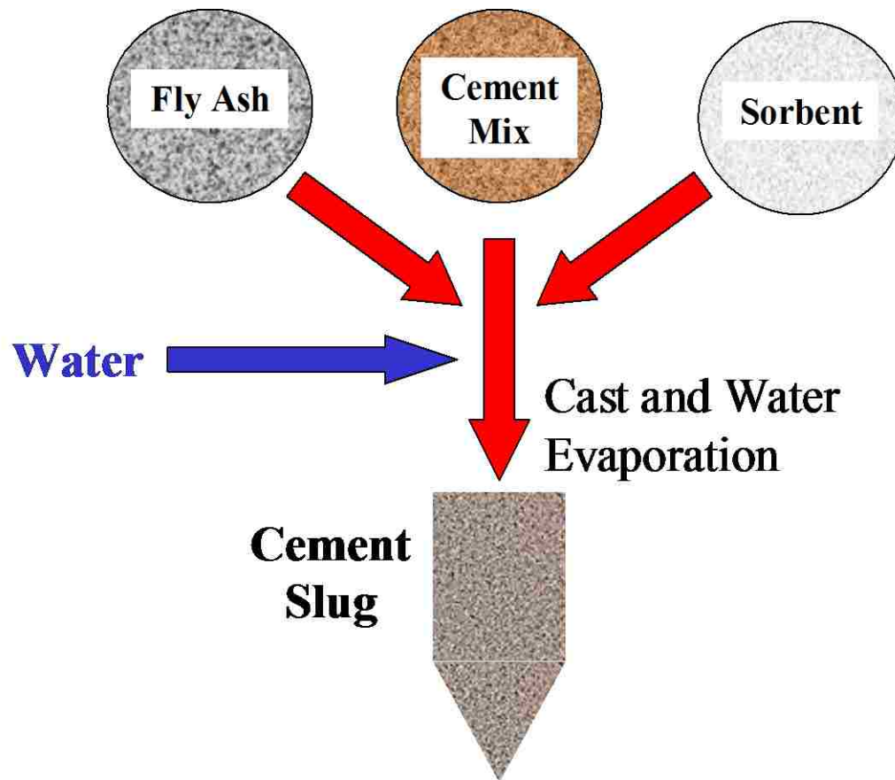
Figure 3.2 Cement slug composition for metal leaching experiments. Exact experimental compositions are given in Chapter 7.
