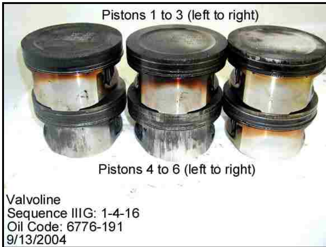
Figure 8. Pistons from Sequence IIIG test
