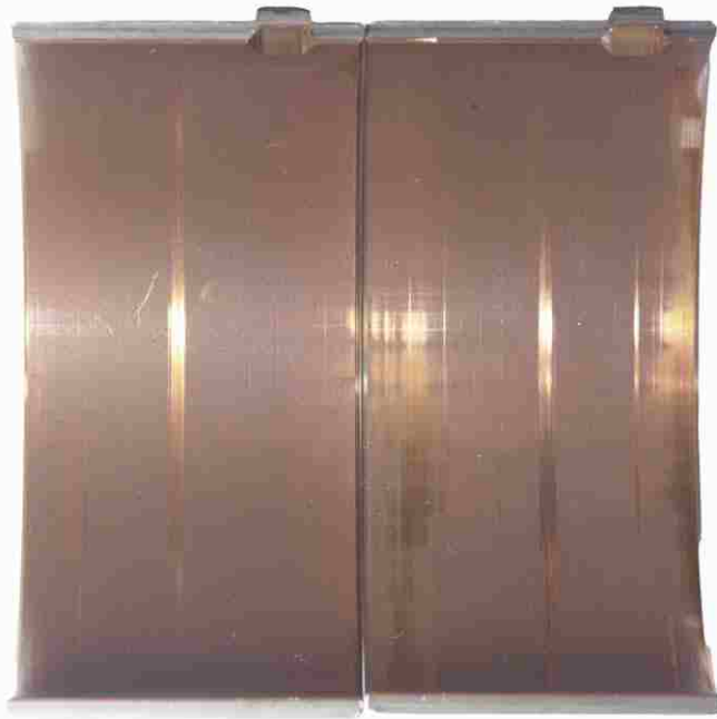
Figure 6. Sequence VIII bearings from Baseline + Inhibitors
