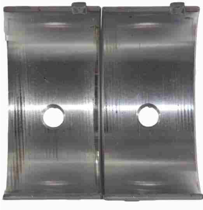
Figure 7. Sequence VIII lead alloy bearings
