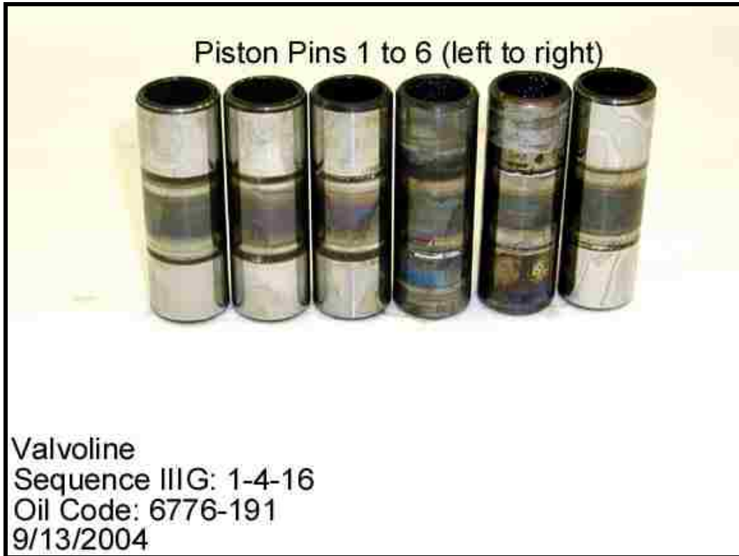
Figure 9. Piston pins from Sequence IIIG test
