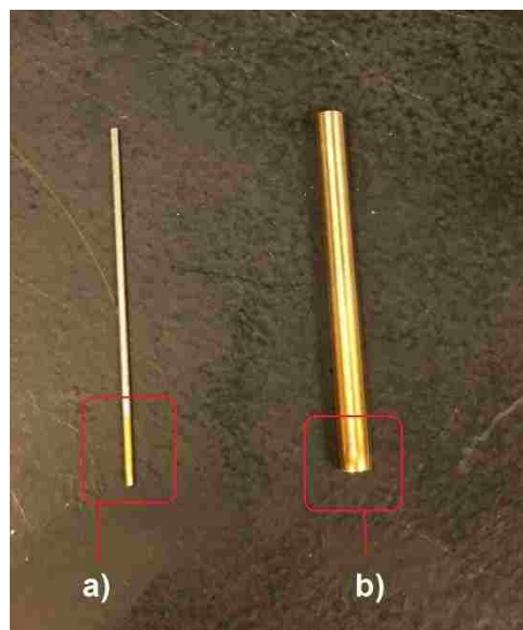
Figure 5.7. Round punches used to make the inlet and outlet of the PDMS microfluidic devices. The highlighted areas show their cutting edges. The round punch of 0.71 mm cutting edge diameter is shown on a) and the punch of 3.02 mm is shown on b).
