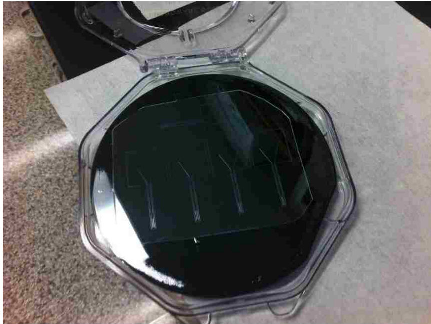
Figure 5.4. SU-8 master mold in a wafer transport box after microfabrication. Up to five PDMS replicas at a time can be made using this mold.
