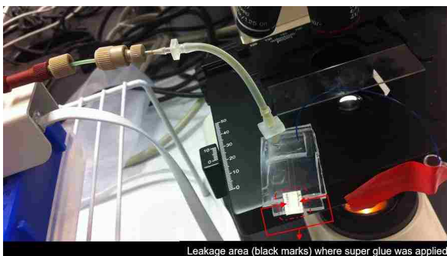
Figure 5.26. PDMS microfluidic device made using fifth assembly during leakage testing using 100 \mu\text{M} methyl orange solution. The red arrows indicate the leakage area where super glue was applied before testing.
