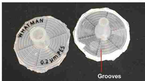
Figure 5.9. PES syringe filter before and after retrieving the PES filter.
