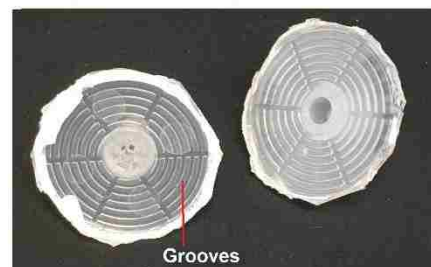
Figure 5.9. PES syringe filter before and after retrieving the PES filter.
