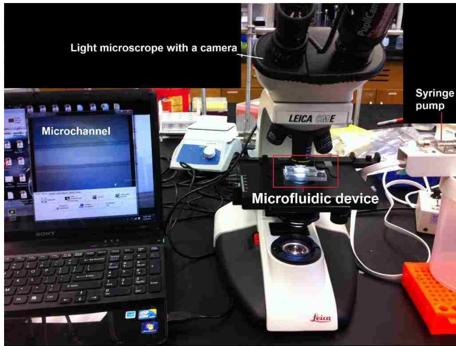
Figure 5.14. Setup used to inspect the microfluidic devices after microfabrication. The left side shows the perfusion fluid flowing in the channel having the PES membrane at the bottom. The microfluidic device shown in this picture corresponds to the simple microfluidic device of one channel made to test Aran et al's method (Figure 5.15).
