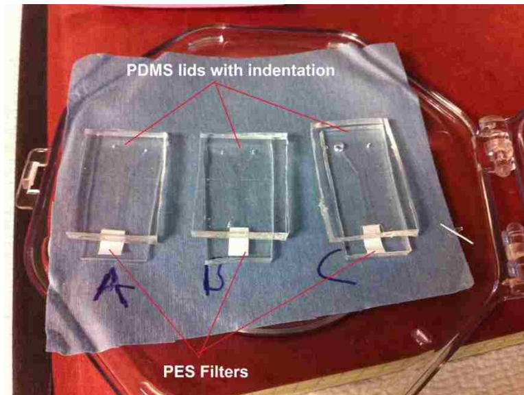
Figure 5.24. Uncut and unbound microfluidic devices for fifth assembly approach.
