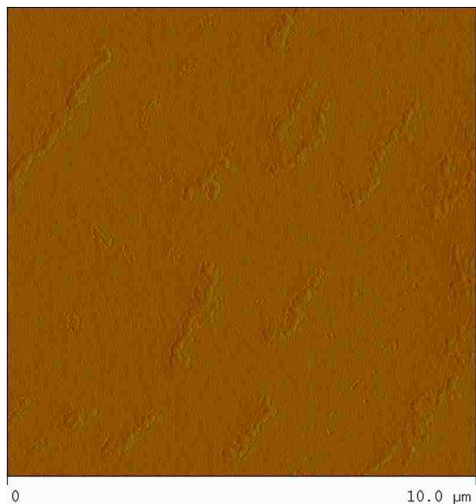
Figure 4.7. Phase AFM image of DSS-SWNT that separated from the free DSS. Notice the minimal free DSS in the field.
