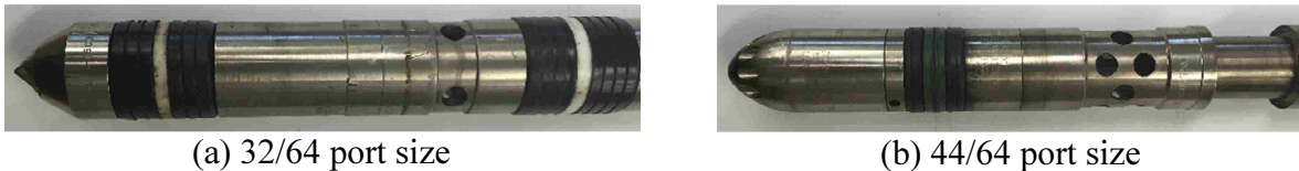
Figure 3.10 . Orifice GLV (a) 32/64, (b) 44/64.
