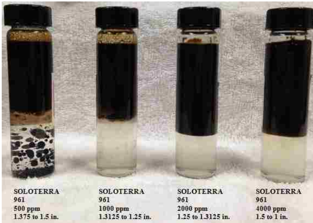
Figure 3.5. Emulsion stability test for SOLOTERRA 961.
