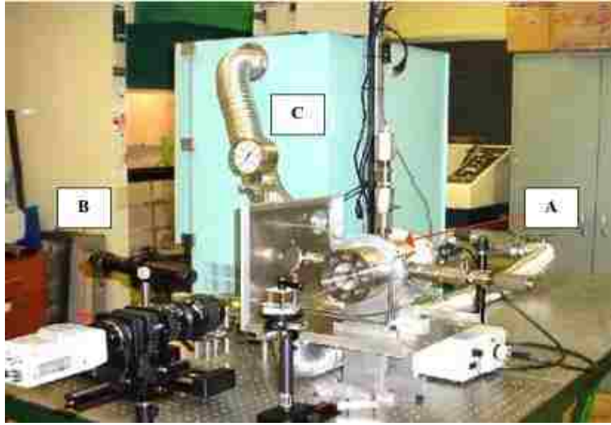
Figure 3.10. IFT and contact angle measurements setup for HPHT conditions, A: Optical cell, B: Digital camera, C: Oven (Xu, 2005).
