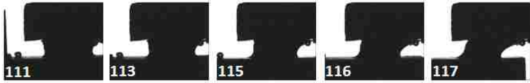
Figure 4.31. Actual images of DDDC method and the corresponding contact angles using Yates oil, limestone, and surfactant (ALF 9S, 100 ppm) at ambient conditions.
