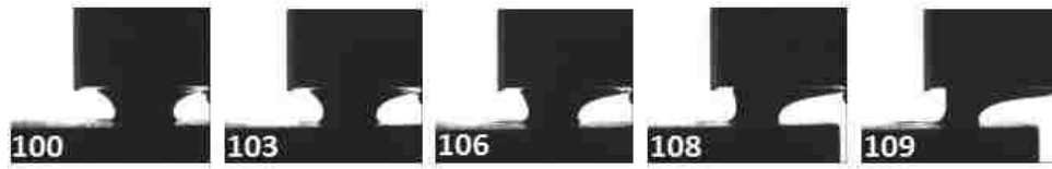
Figure 4.35. Actual images of DDDC method and the corresponding contact angles using Yates oil, limestone, and surfactant-based nanofluid (0.4 wt.% NP+ALF 9S, 50 ppm) at ambient conditions.
