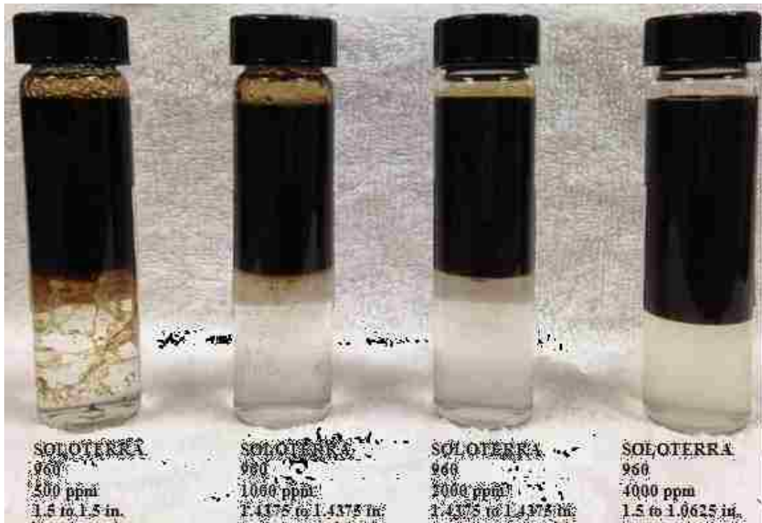
Figure 3.4. Emulsion stability test for SOLOTERRA 960.
