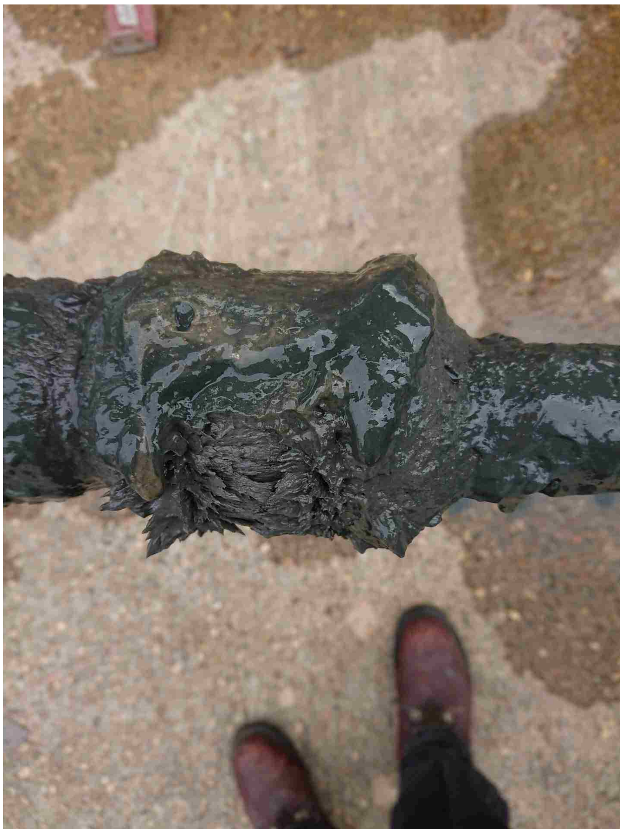
Image of gelled particles around magnets showing magnetic field lines
