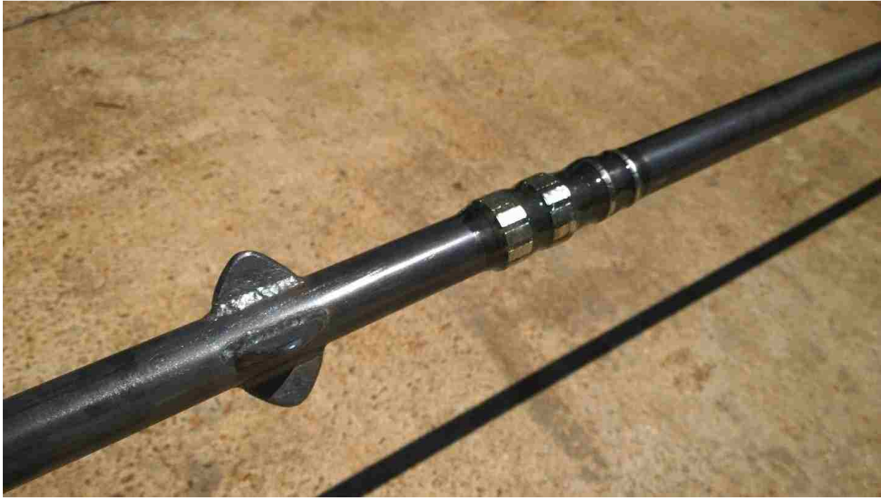
Image showing magnet rings and middle centralizer on inner pipe
