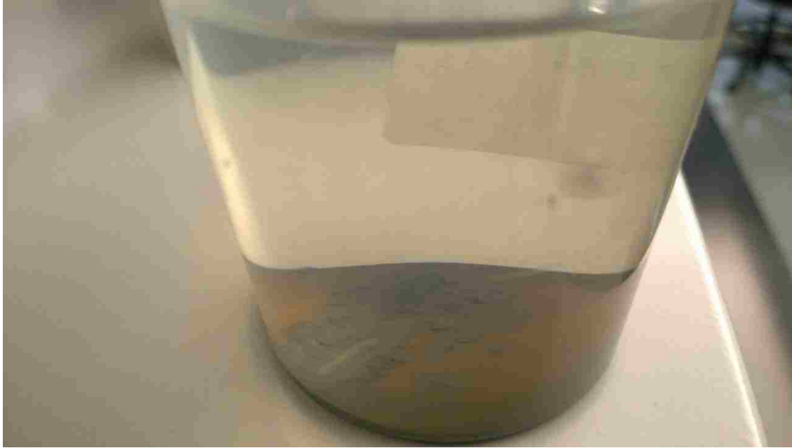
Image of Sample 5 at 8 days after mixing. Bottom has been scraped to reveal that the rust is only on the surface.
