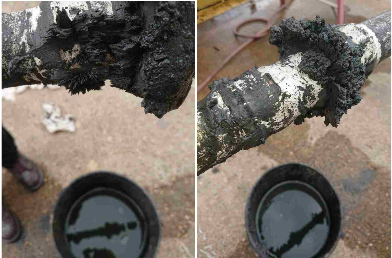
Images showing magnetorheological fluid aligning with magnetic field lines.
