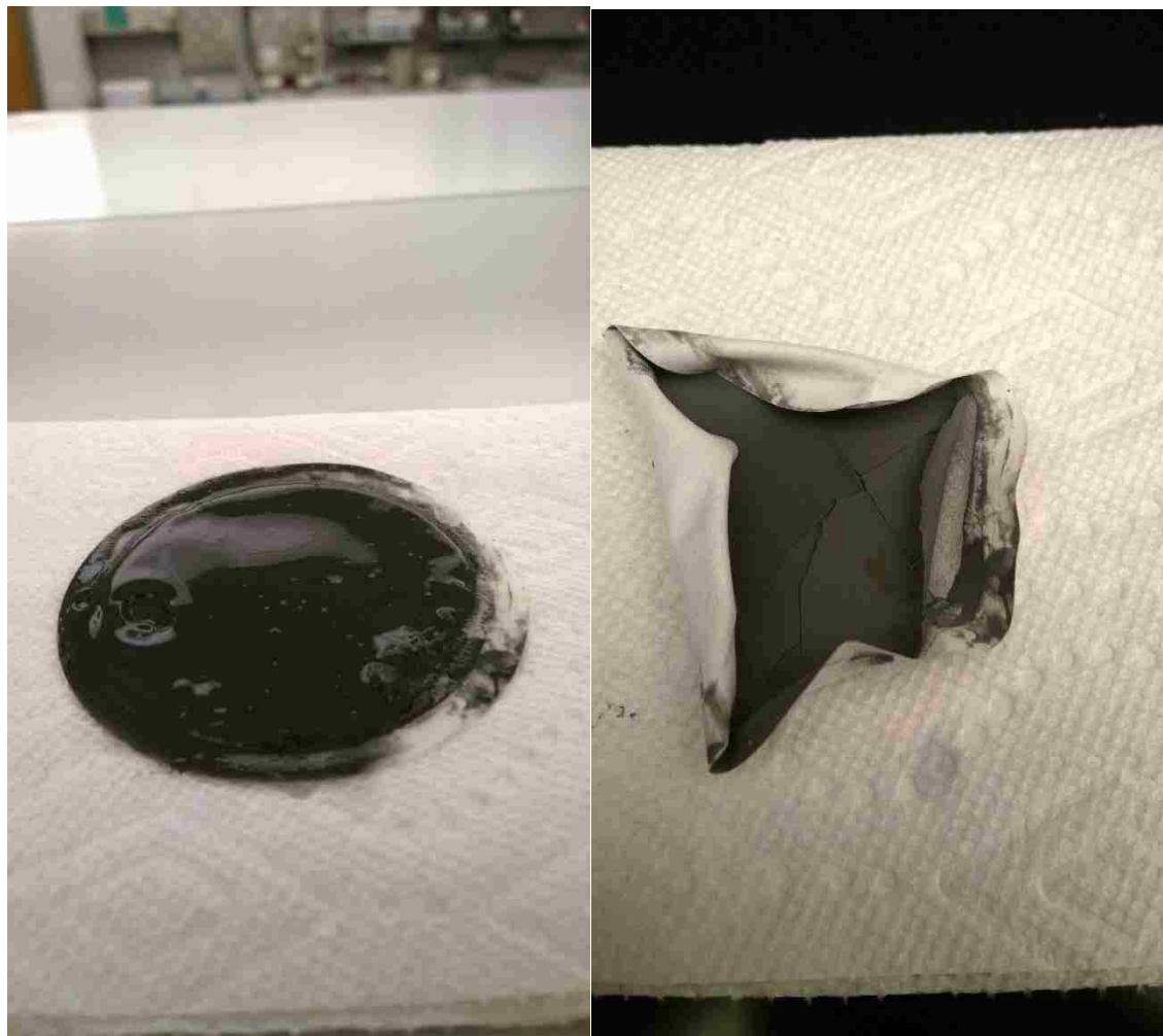
Images of Sample 2 filter paper immediately (left) and 24 hours (right) after API filter press test.
