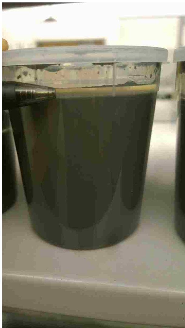
Image of Sample 3 taken 19 days after mixing showing the liquid water separating out of solution.
