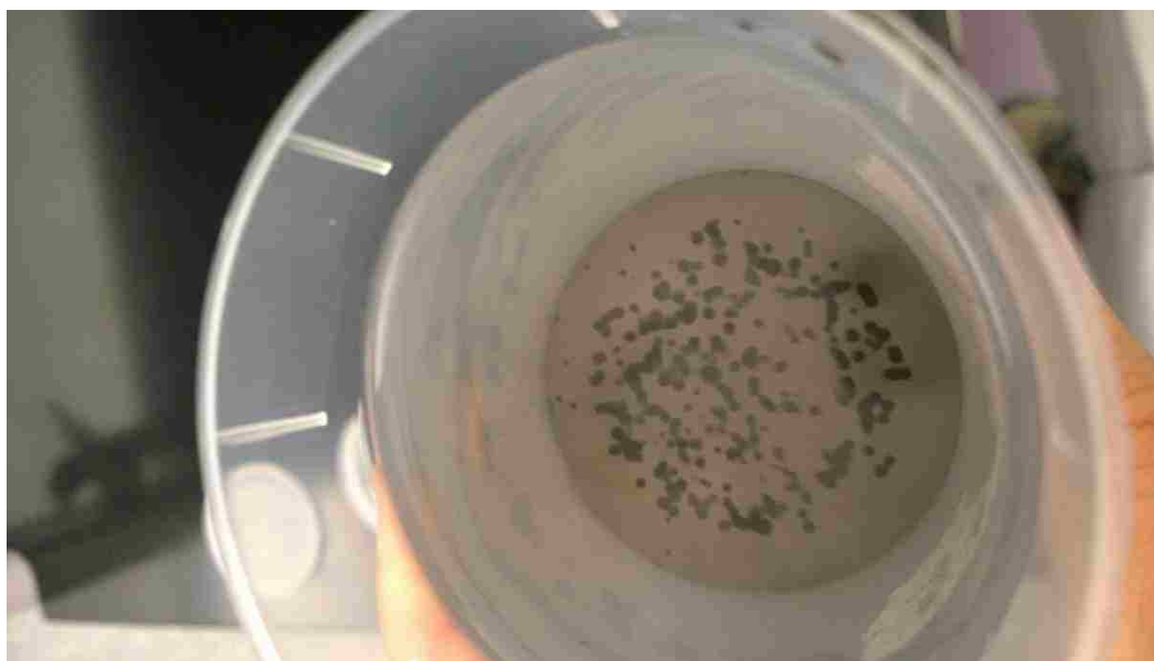
Image of Sample 5 at approximately 98 hours after mixing. Notice that particles on the edge of the container do not have the same discoloration seen at the bottom of the container.
