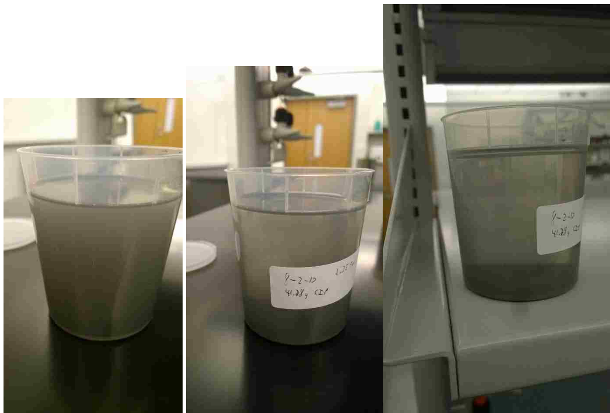
Image of Sample 5 taken at (from left to right) 4 minutes, 12 minutes and 17 minutes after mixing
