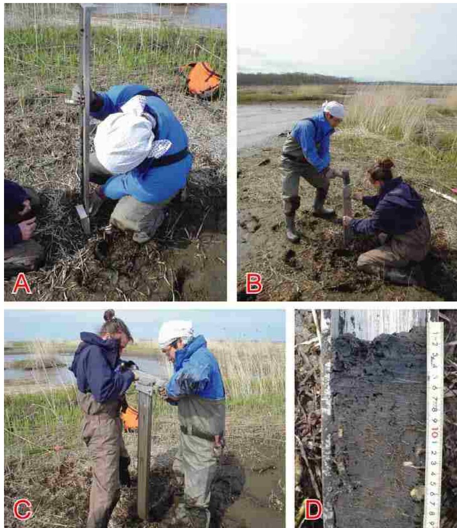
Figure 3.3 Photographs illustrating the use of a Geoslice corer. After the initial sampling tray is hammered into the sediment, a shutter plate is attached (A) and hammered into place. A handle is then screwed onto the Geoslice and is used to extract the sediment (C) ready for its lithostatigraphic description (D).
