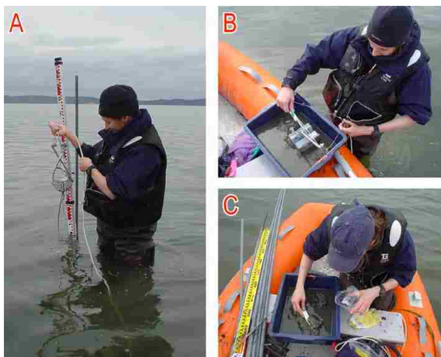
Figure 3.5 Subtidal sampling at Akkeshi-ko. (A) Sampling in Akkeshi-ko, with Ekman Bottom Grab sampler. At each location, the sampler is used to extrude the bay sediments and the depth of time-still water is noted to be used to calculate the elevation of the sample using the nearby Kushiro tidal-gauge station. (B) The grab sampler is emptied into a shallow tray, and the uppermost sediment is scraped for bio-, and lithostratigraphical analysis (C).
