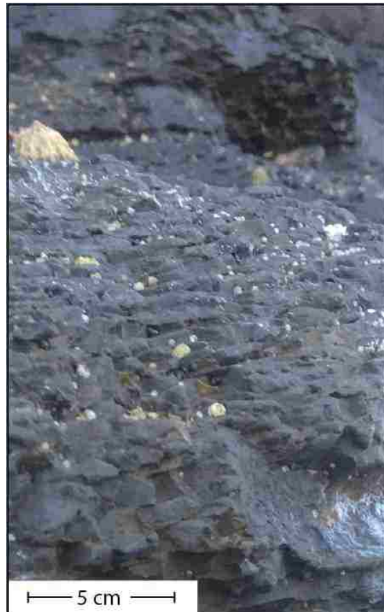
Figure 8.5: Detail of shale fabric at Site 4, illustrating considerable roughness and micro-relief as an indicator of platelet fragmentation.
