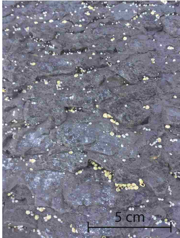
Figure 4.5: Detail from the shale at Site 5. Note the cm-scale platelets defined by horizontal laminations which break along seemingly randomly-oriented failure planes.
