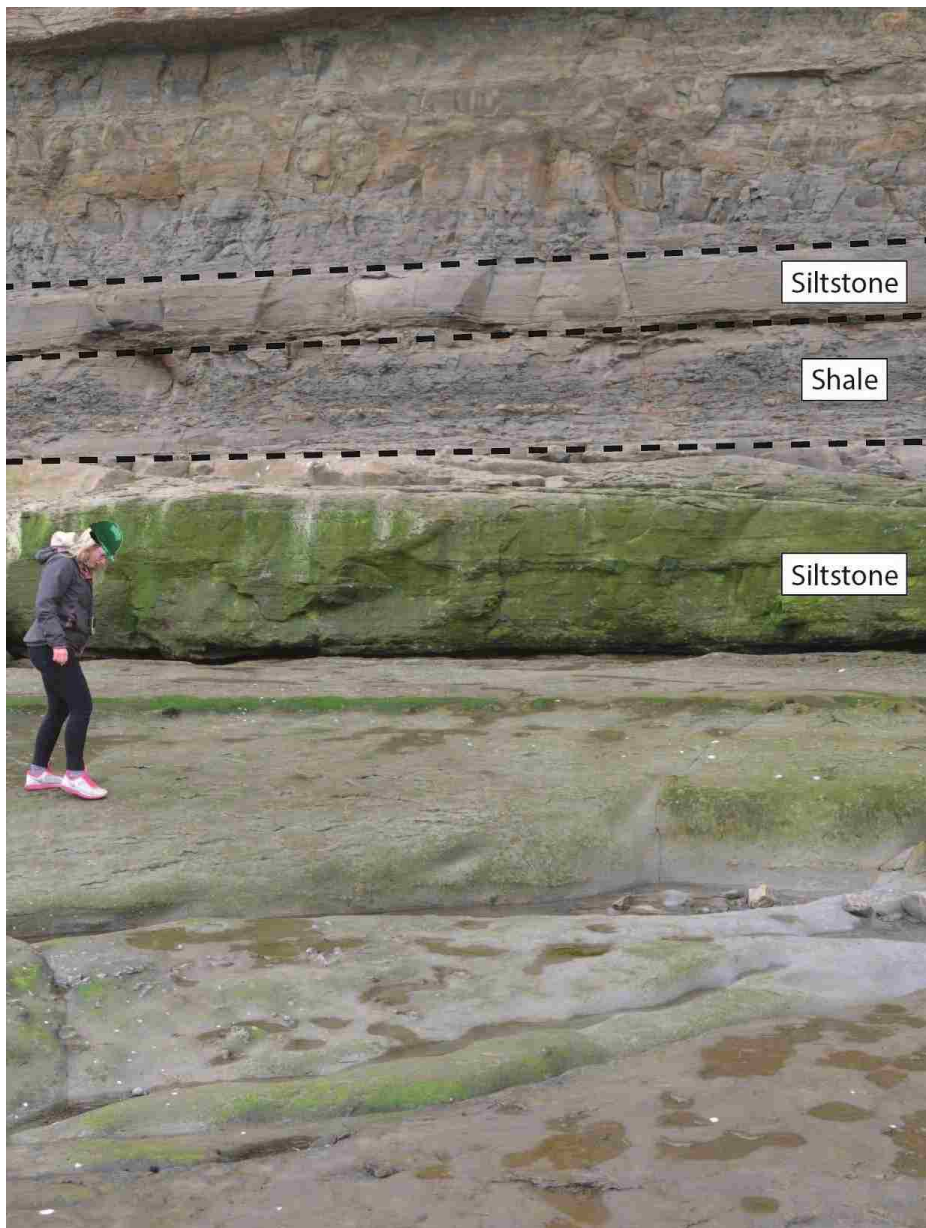
Figure 8.4: Cliff section showing the smooth, quarried joint boundaries in the upper siltstone contrasting with the fabric-controlled, rough shale surface. Fieldworker for scale.
