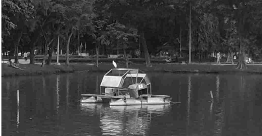
Image 4.8. Machine to increase oxygen level in water. Invented by the late Rama IX. Lumpini Park, Bangkok, 2015. Own image.
