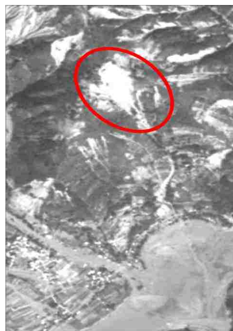
Figure 3.16: Extension of a co-seismic failure in the hanging wall at Huangjiaba – images (left to right): S1 (June 2008); S2 (October 2008); S3 (March 2009)
