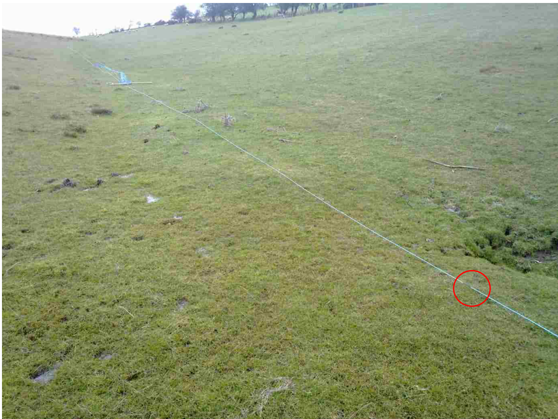
Figure 3.11: Image of marked rope strung between permanent transect stakes used to locate 5 m grid points. 5 m rope mark is highlighted by a red circle.
