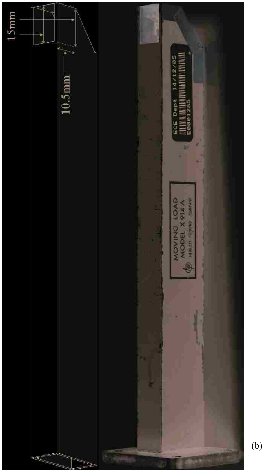
Figure 5.1. (a) Schematic of X-band HPB-radiator for experimental verification. (b) X-band HPB-radiator used for experimental verification.
