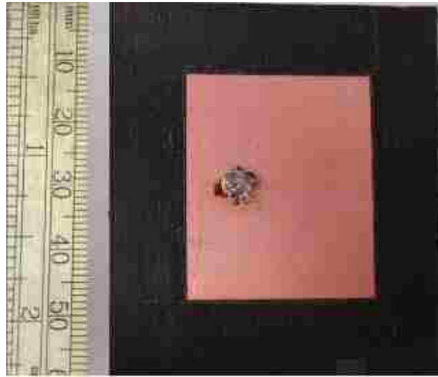
Figure 4.16: Fabricated conventional MSA with patch scaled by 0.7.
