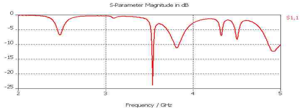
Figure D.2: Simulated reflection coefficient curve for stacked MSA with top layer of \epsilon_r = 1.05 .
