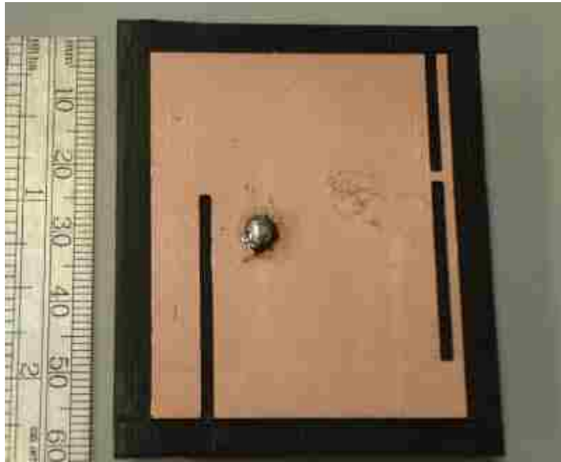
Figure 4.7: Fabricated bottom MSA with two slots when SW1 is OFF and SW2 is ON.
