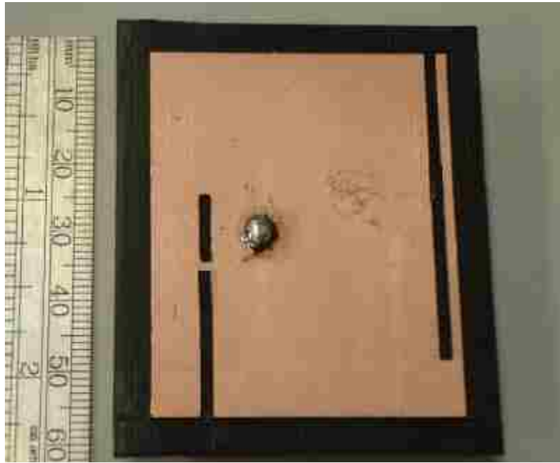
Figure 4.5: Fabricated bottom MSA with two slots when SW1 is ON and SW2 is OFF.
