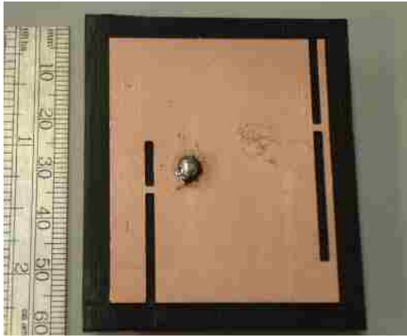
Figure 4.9: Fabricated bottom MSA with two slots when SW1 and SW2 are ON.
