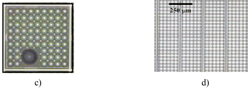
Figure 2.1 a) the cross-sectional schematic of the single CMUT Cell, b) The cross section of CMUT array; c) The 2-D array elements d) The 1-D array elements
