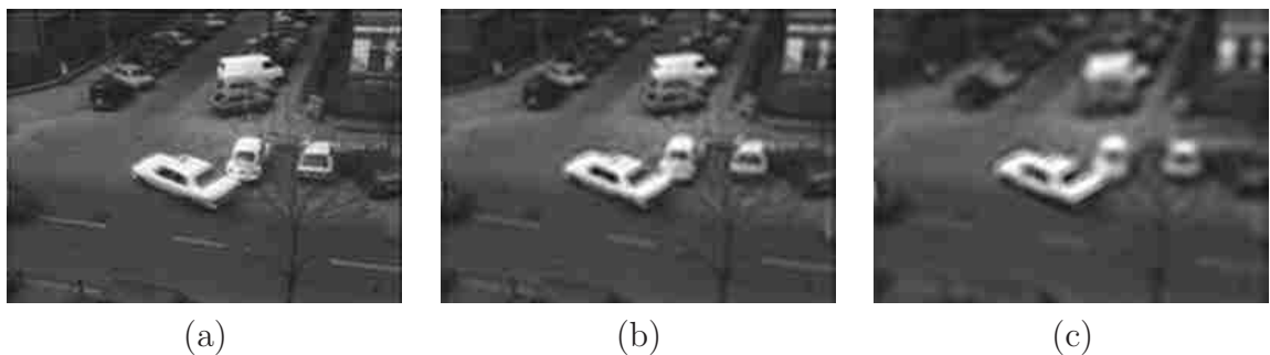
Figure 8.6: Video reconstructions for the taxi video (we only show frame 1) using dominant components from each scale. (a) 3D Single-scale filterbank. (b) 3D Two-scale filterbank. (c) 3D Three-scale filterbank.
