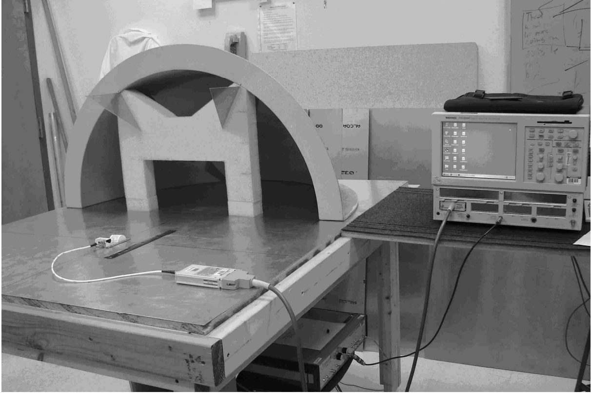
Figure 6.3: Experimental setup for a 60^\circ four-feed arm prolate-spheroidal IRA.
