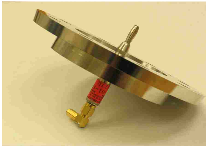
Figure 3.14: A single CVR threaded through the base plate for the calibration setup.
