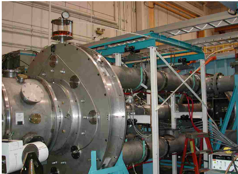
Figure 3.6: Load section of Tesla pulser. MITL hardware is contained within the vacuum section which is at the center of the insulator stack disk. Four pulse-forming water lines supply the power pulse to the MITL.
