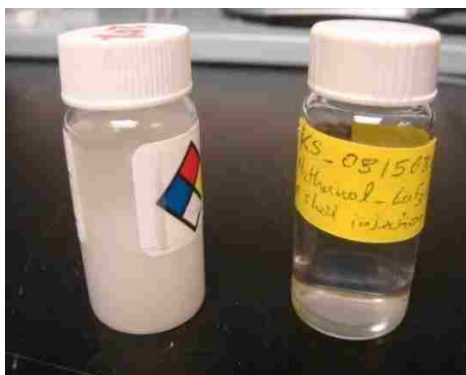
Figure 4.5: Anhydrous synthesis (right) produced a more stable and optically transparent colloidal dispersion compared to the aqueous synthesis (left)
