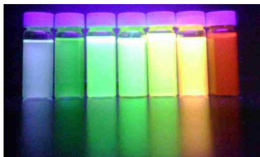
Figure 1.1: CdSe NCs of different sizes, synthesized at CHTM, fluorescing with different colors under UV excitation
