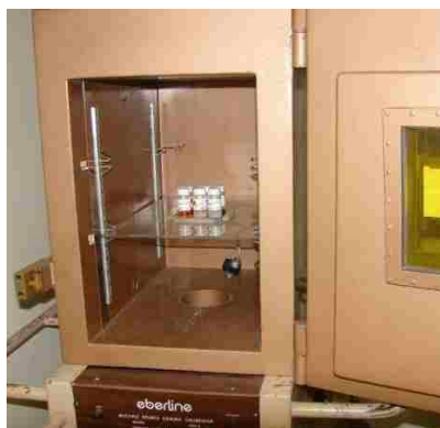
Figure 6.1: NC samples placed inside the Eberline 1000B multiple source \gamma calibrator (A ^{137}\text{Cs} 662 keV \gamma ray source was used for the experiment)
