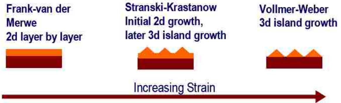
Figure 1.5: Three modes of strained heteroepitaxial growth.
