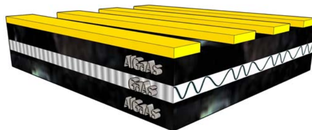
Figure 2-3: Plasmon oscillations in a MISFET
