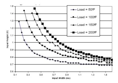
Figure 2.2 Noise rejection curves for an inverter [19].
