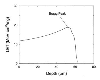
Figure. 1.1. Linear energy transfer (LET) versus depth curve for 210-MeV chlorine ions in silicon [2].
