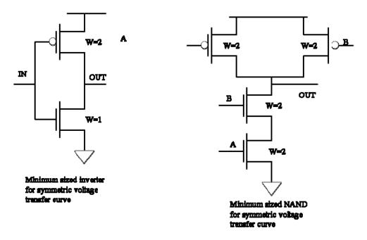
Figure 3.2. Minimum sized inverter and NAND gate for symmetric VTC.
