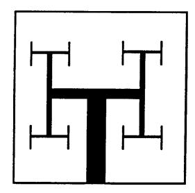
Figure 4.4. H-tree structure for global clock distribution [48].
