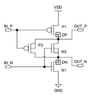
Figure 4.21. Radiation hardened clock driver from [34].
