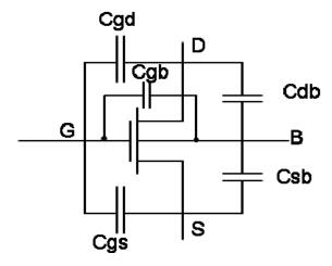
Figure 4.15. Parasitic capacitance of a NMOS transistor [43].
