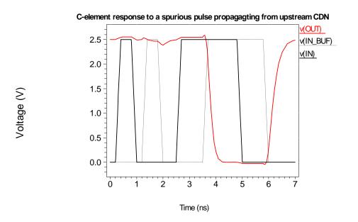
Figure 4.14. (a) Response of C-element to spurious pulse propagating from upstream CDN.  $T_{SEU} = 400 ps$  and  $T_D = 1.25 ns$ .
