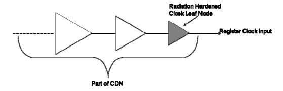
Figure 4.8. Implementation of radiation hardened clock leaf driver in a CDN
