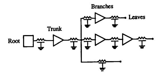
Figure 4.3. Clock tree structure [48].
