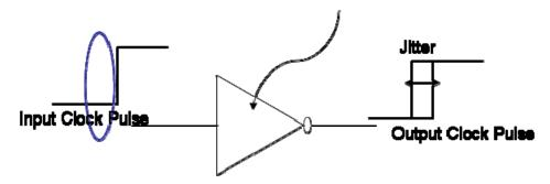
Figure 4.6. (a). Radiation induced clock jitter
