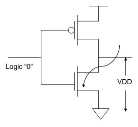
Figure 4.18. Radiation strike on NMOS of an inverter
