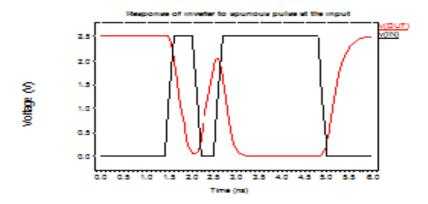
Figure 4.12. Spurious pulse at the input of a clock leaf driver may produce race condition.
