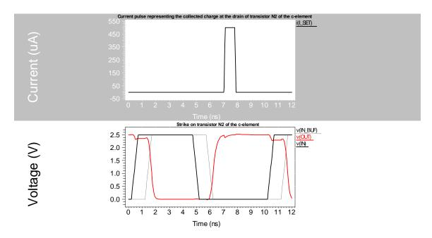
Figure 4.19.(b) Strike on transistor N2 of the C-element
