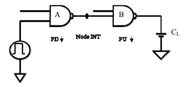
Figure 3.1. NAND 2x chain with different PD and PU strengths. First gate has a decreased PD strength and second gate has a decreased PU strength. A rising pulse input is given to the first gate.
