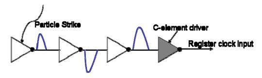
Figure 4.13. Particle strike on a clock driver before the C-element driver leading to spurious pulse at the input of C-element driver.
