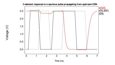
Figure 4.14. (b) Response of C-element to spurious pulse propagating from upstream CDN.  $T_{SEU} \sim 1$ ns and  $T_D = 1.25$ ns.
