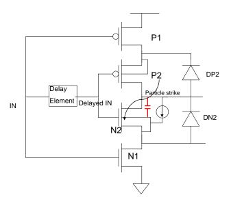
Figure 4.16. Strike on N2 modeled as a current source between drain and bulk of N2 charges the Cdb capacitor of N2.
