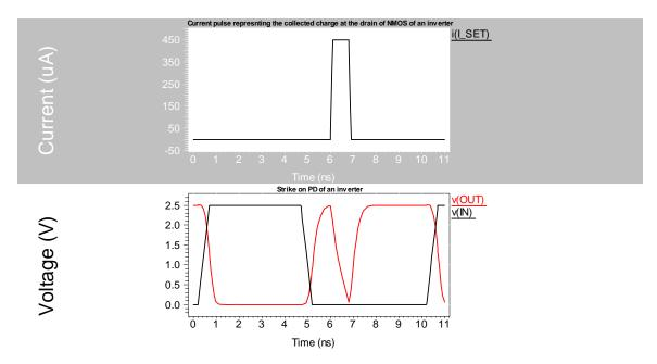
Figure 4.19.(a) Strike on PD of inverter.
