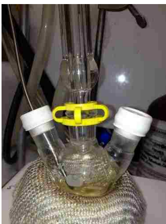
Figure 6.2: Ligand Exchange Reflux Apparatus
