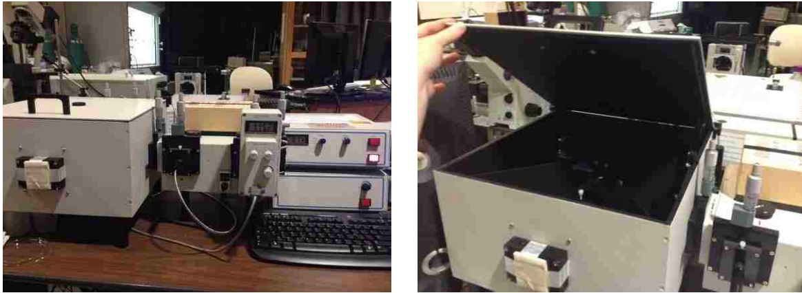
Figure 2.4: PTI Spectrofluorometer with top opening sample chamber hatch
