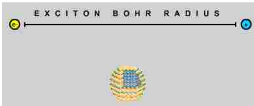
Figure 1.4. A quantum dot exhibits bandgap tunability because it is smaller than the spatial separation between the electron and its hole, known as the exciton Bohr radius. ( http://janosh.myweb.usf.edu/QDs.html )
