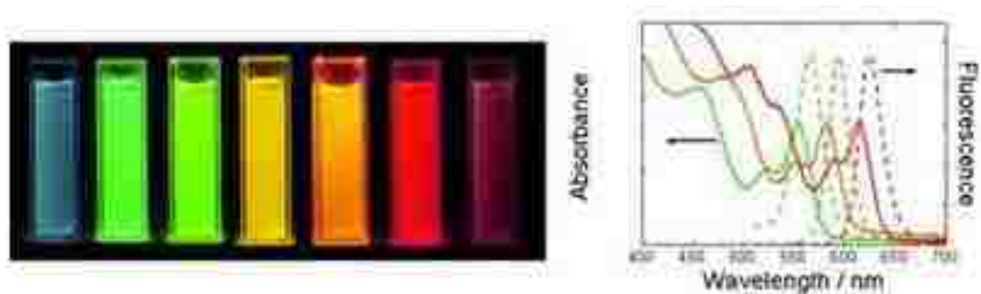
Figure 1.1. The wavelength of light emitted by quantum dots is tunable by changing the particle size. In this image, all of the quantum dot particles are excited by same UV wavelength, but emit different visible wavelengths depending upon particle size.
