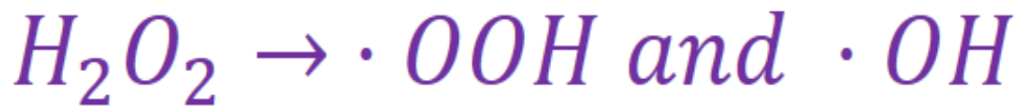
Figure 5. Fuel crossover allows the H_2 and O_2 to react and create hydroxy and hydroperoxy radicals. 7
